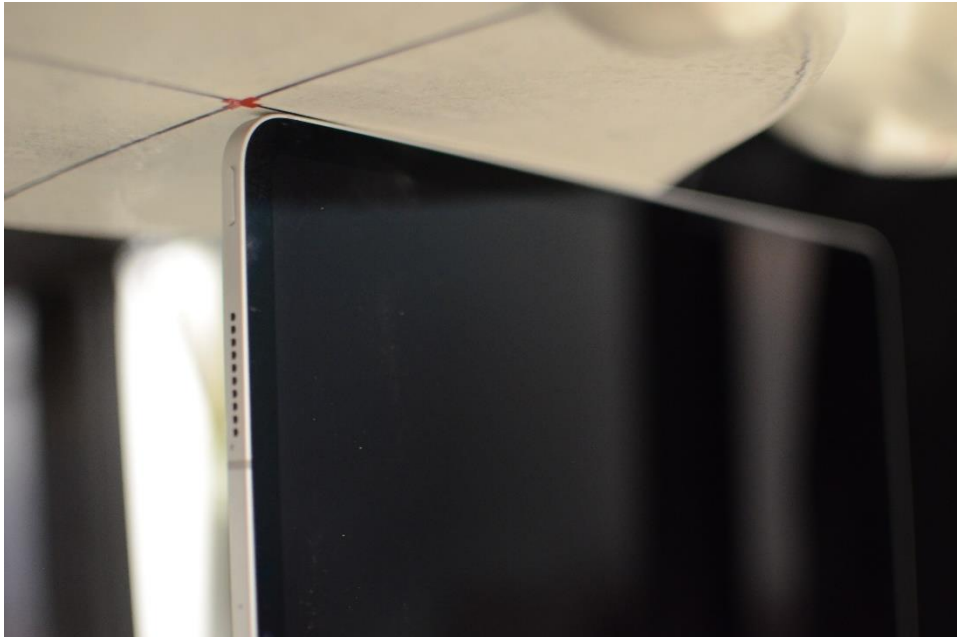
SAR Test Setup Photo 6 Right Edge at 0mm, Antennas WF7, WF8
