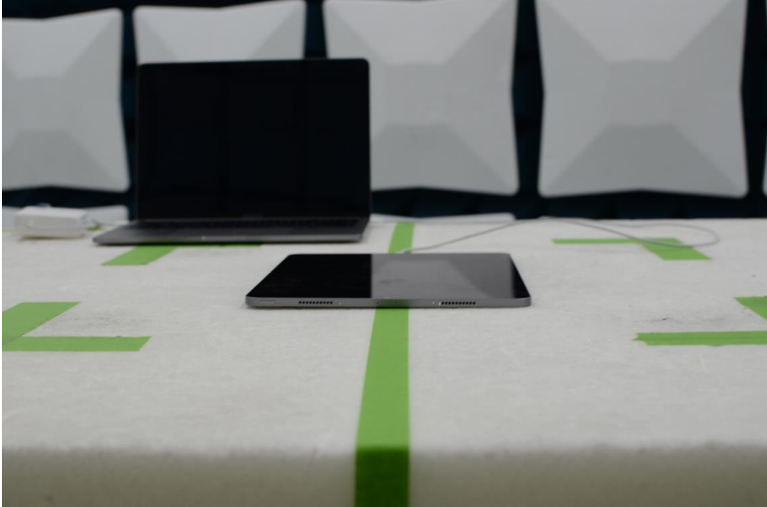
Figure 17: 30MHz-1GHz Test Setup (Front View)
