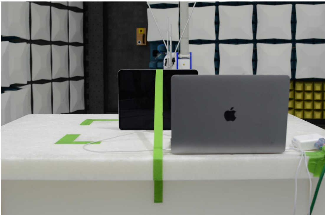
Figure 20: 30MHz-1GHz Test Setup (Rear View)
