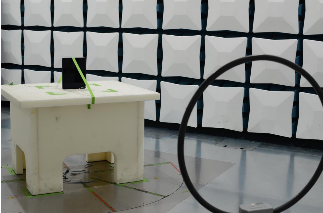
Figure 25: 9kHz-30MHz Test Setup (Front View)
