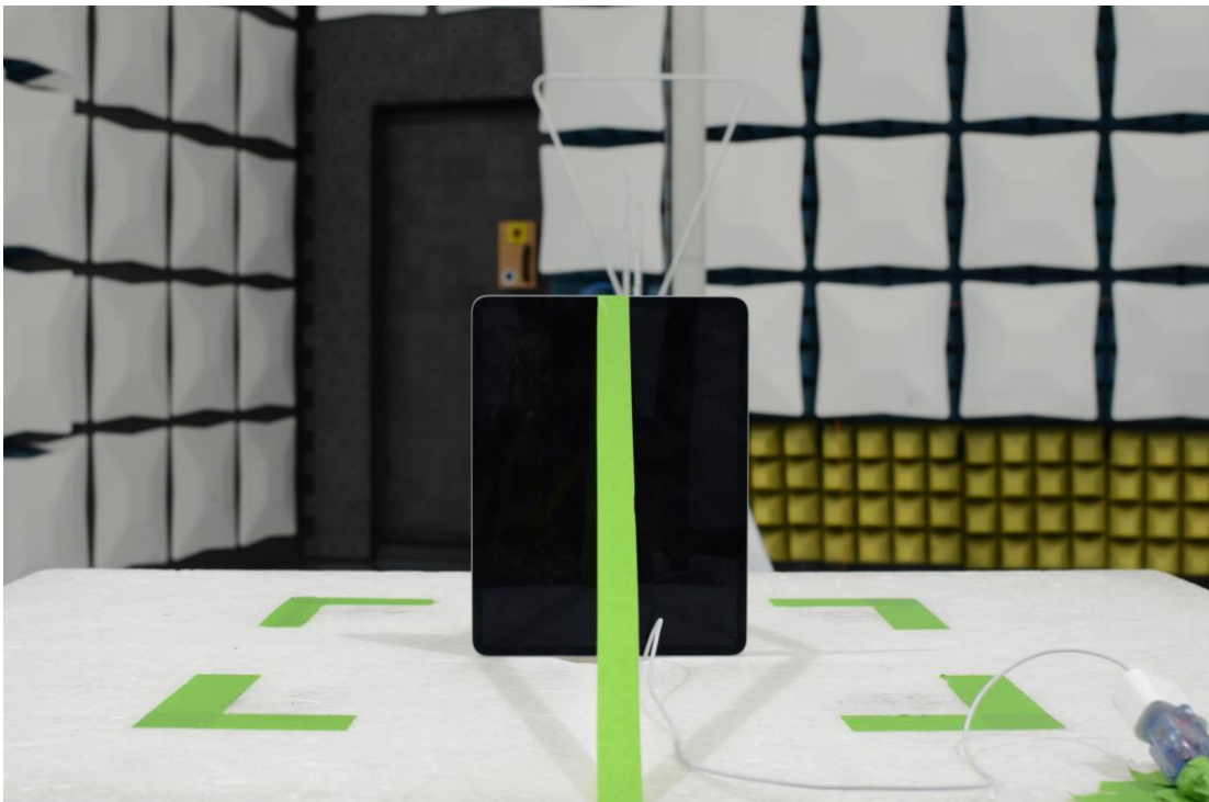
Figure 16: 30MHz-1GHz Test Setup (Rear View)
