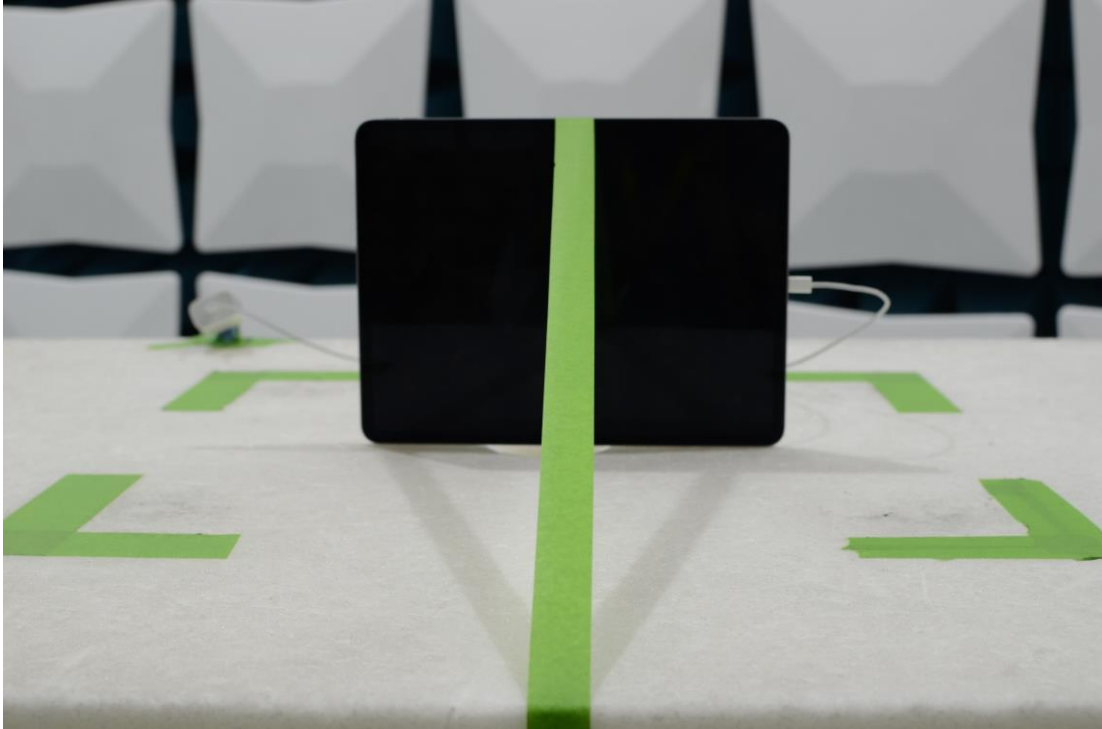
Figure 13: 30MHz-1GHz Test Setup (Front View)
