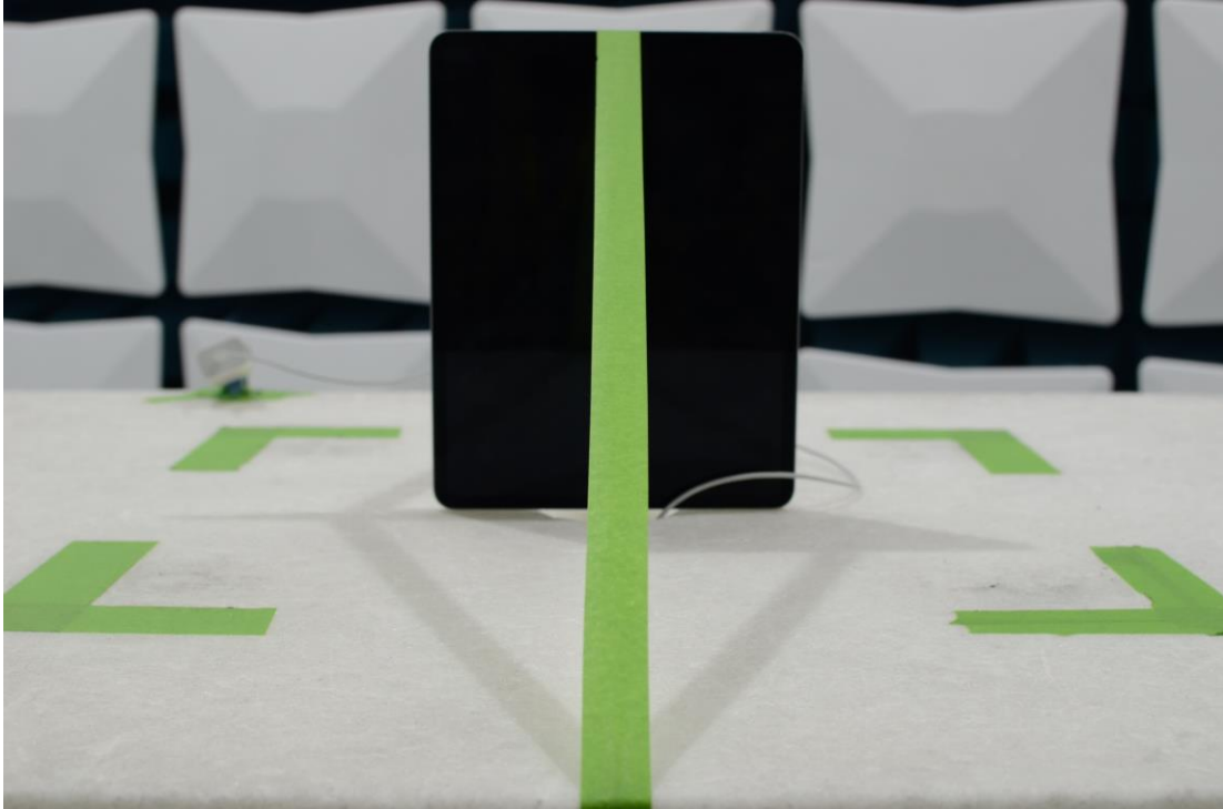
Figure 15: 30MHz-1GHz Test Setup (Front View)
