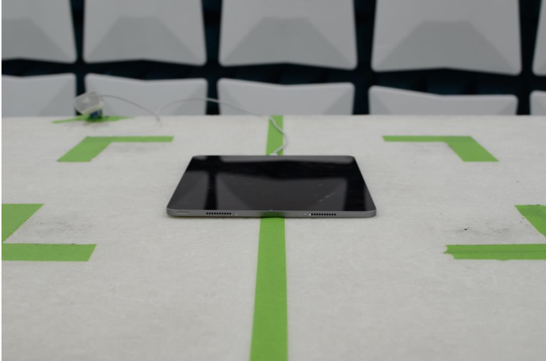
Figure 11: 30MHz-1GHz Test Setup (Front View)
