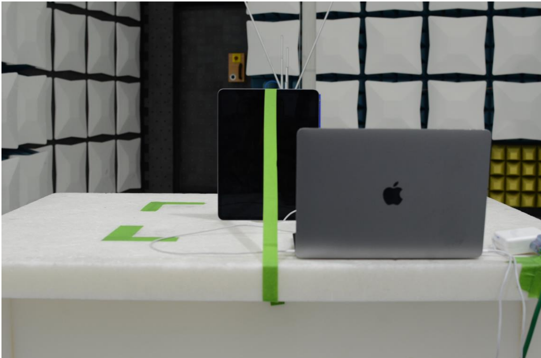
Figure 22: 30MHz-1GHz Test Setup (Rear View)
