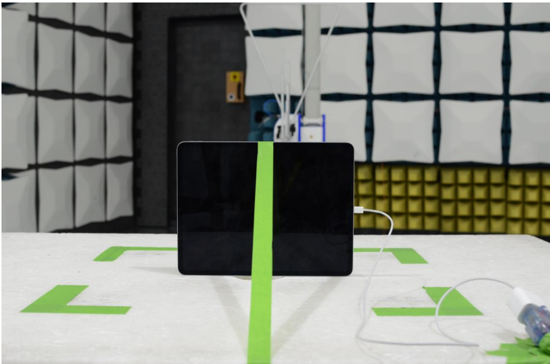
Figure 14: 30MHz-1GHz Test Setup (Rear View)
