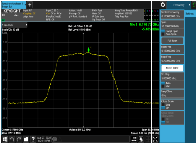
Plot 7-205. Power Spectral Density Plot Antenna 4a (20MHz 802.11a (UNII Band 5) – Ch. 45, MCS4)
