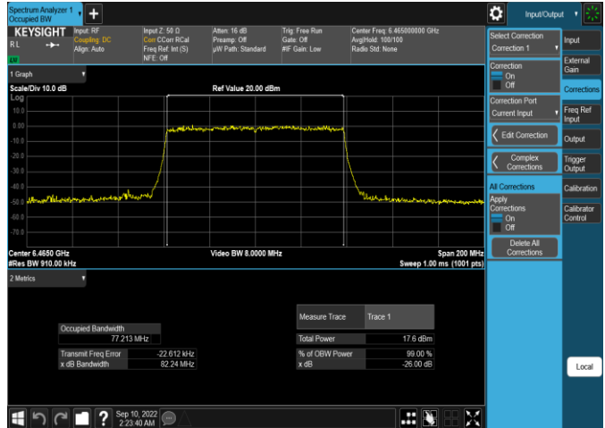
Plot 7-92. 26dB & 99% Bandwidth Plot Antenna 4a (80MHz 802.11ax RU96 (UNII Band 6) – Ch. 103)
