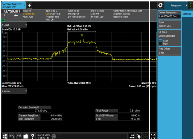
Plot 7-90. 26dB & 99% Bandwidth Plot Antenna 4a (80MHz 802.11ax RU26 (UNII Band 6) – Ch. 103)
