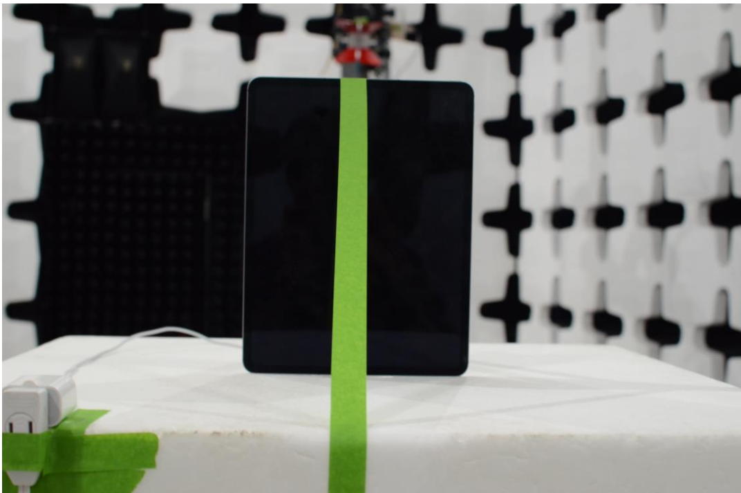
Figure 10: 1-18GHz Test Setup (Rear View)
