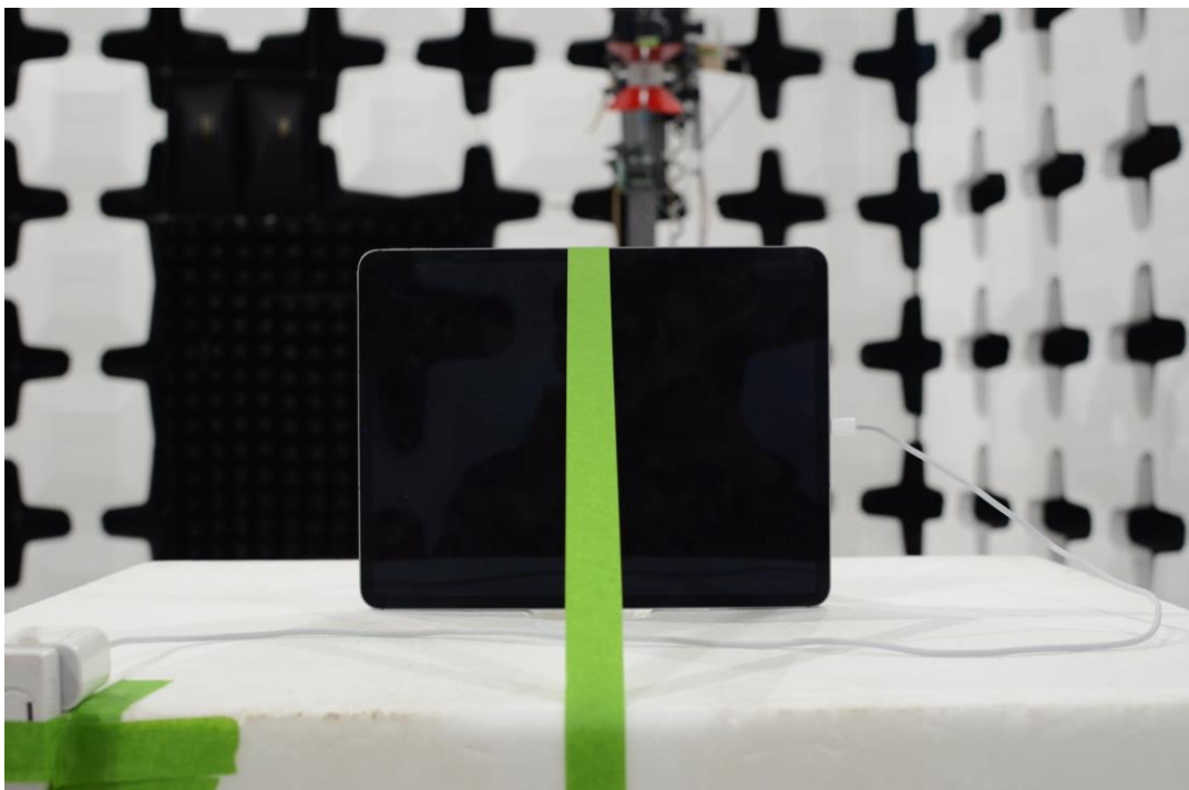
Figure 8: 1-18GHz Test Setup (Rear View)
