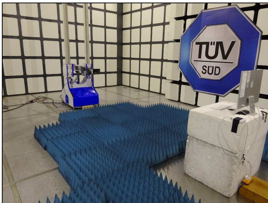
Figure 2 - Radiated Disturbance - Above 1 GHz
