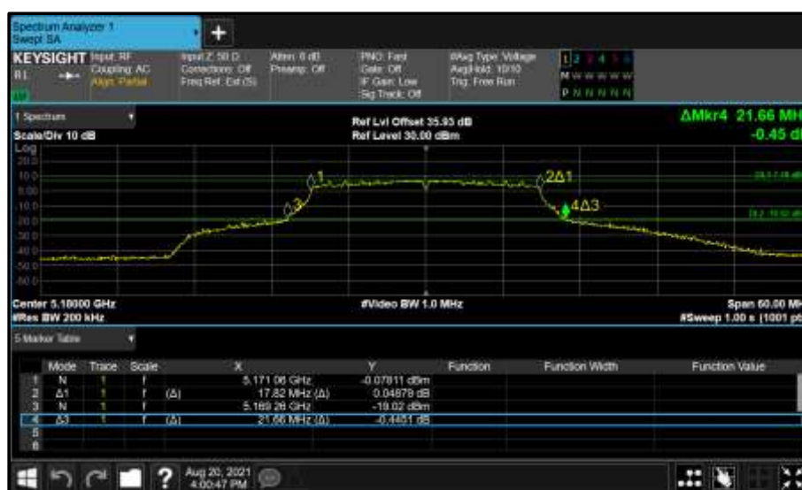
Figure 109 - Core 0 (A) 5180 MHz (CH36) 26 dB and 99% Bandwidth
