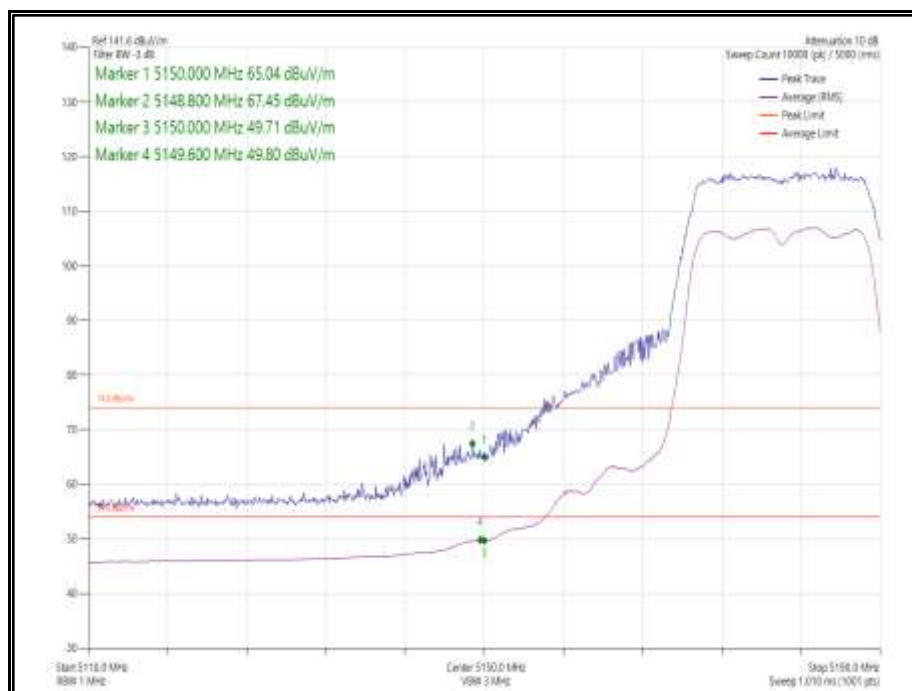
Figure 14 - 802.11n HT20 SDM, Cores 0-1 - 5180 MHz Band Edge Frequency 5150 MHz
