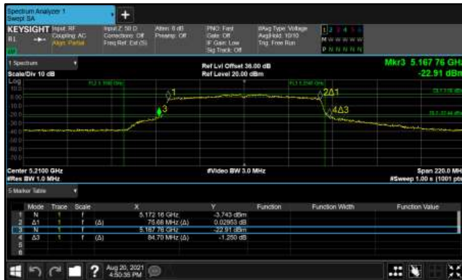
Figure 145 - Core 0 (A) 5210 MHz (CH42) 26 dB and 99% Bandwidth
