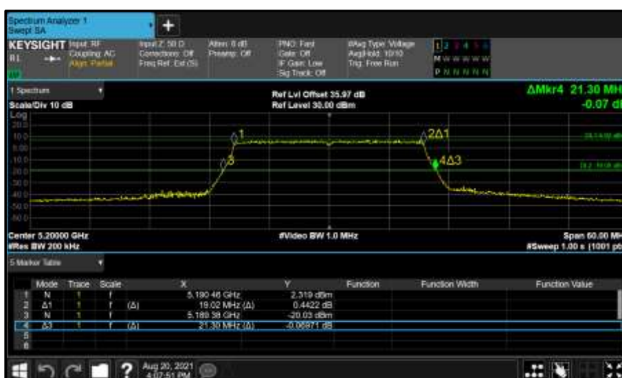
Figure 171 - Core 0 (A) 5200 MHz (CH40) 26 dB and 99% Bandwidth
