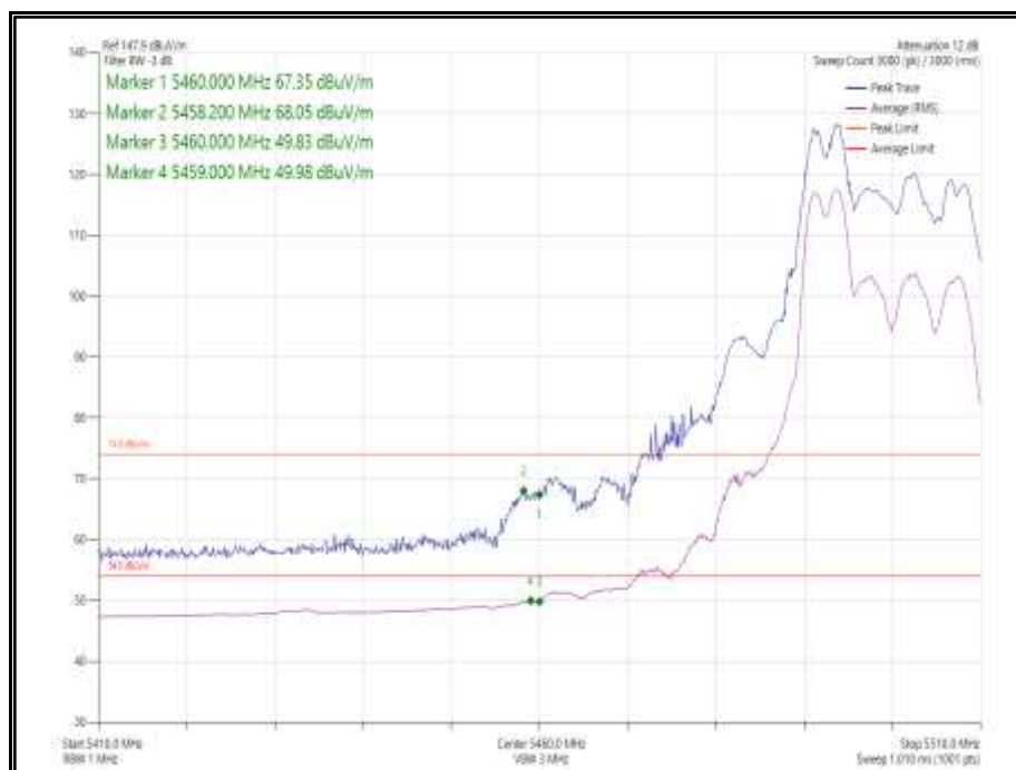
Figure 28 - 802.11ax HE20 CDD, Cores 0-1, 52-37 - 5500 MHz Band Edge Frequency 5460 MHz
