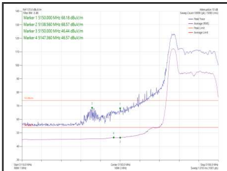
Figure 4 - 802.11ax HE20, Core 0, 26-0 - 5180 MHz, Band Edge Frequency 5150 MHz
