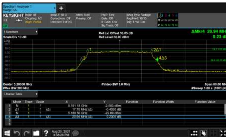
Figure 100 - Core 1 (B) 5200 MHz (CH40) 26 dB and 99% Bandwidth
