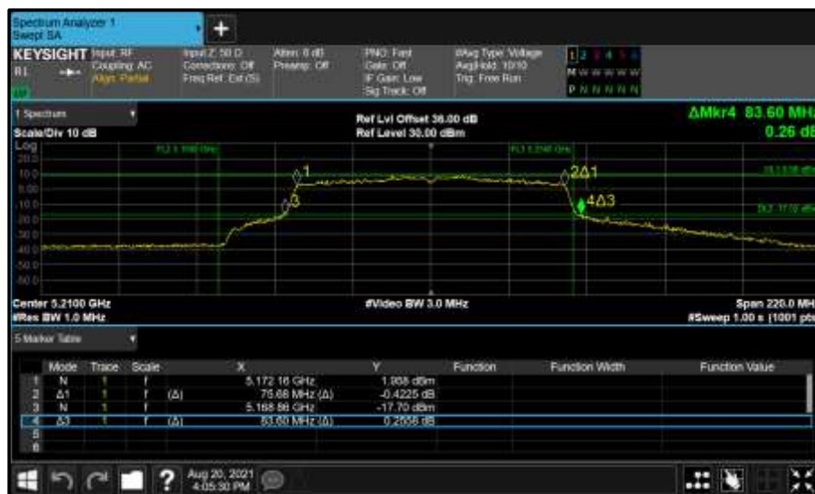
Figure 147 - Core 0 (A) 5210 MHz (CH42) 26 dB and 99% Bandwidth
