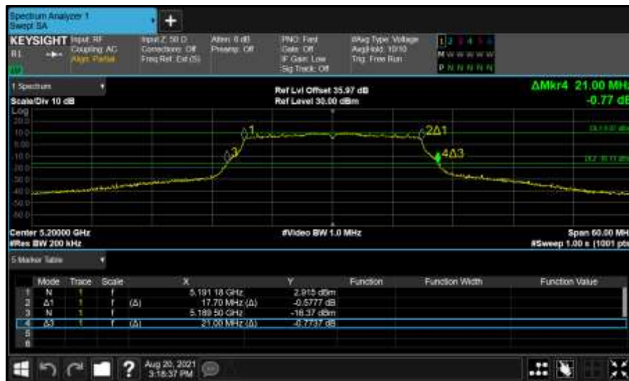
Figure 92 - Core 0 (A) 5200 MHz (CH40) 26 dB and 99% Bandwidth
