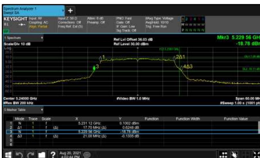
Figure 113 - Core 0 (A) 5240 MHz (CH48) 26 dB and 99% Bandwidth
