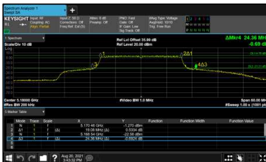
Figure 158 - Core 1 (B) 5180 MHz (CH36) 26 dB and 99% Bandwidth
