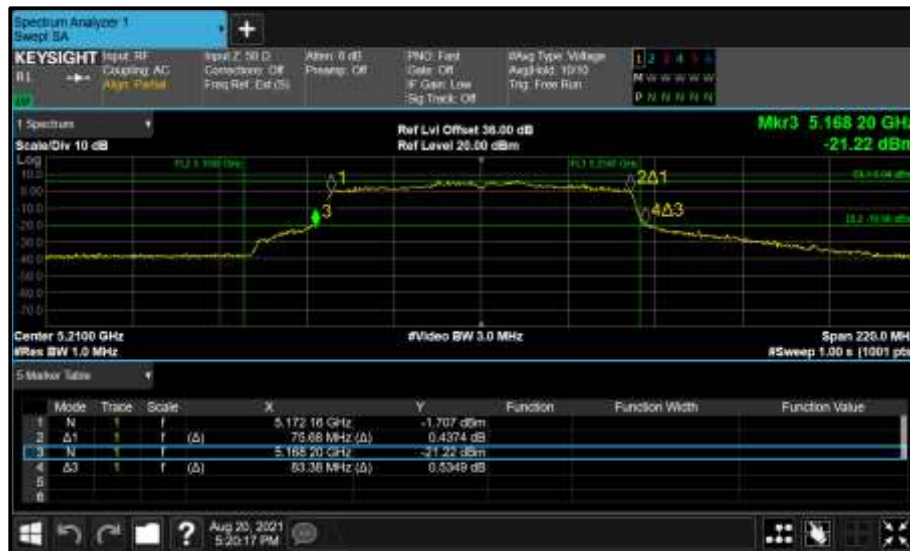
Figure 149 - Core 0 (A) 5210 MHz (CH42) 26 dB and 99% Bandwidth
