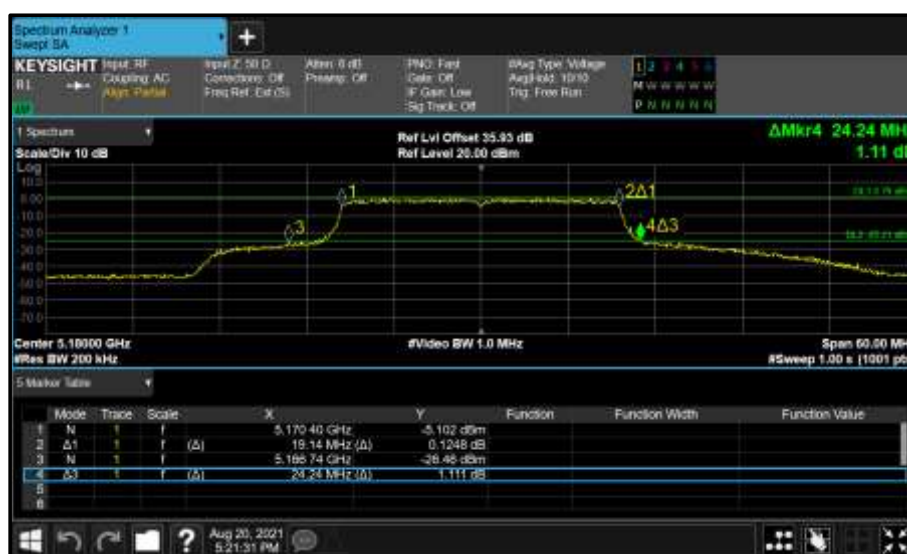
Figure 175 - Core 0 (A) 5180 MHz (CH36) 26 dB and 99% Bandwidth
