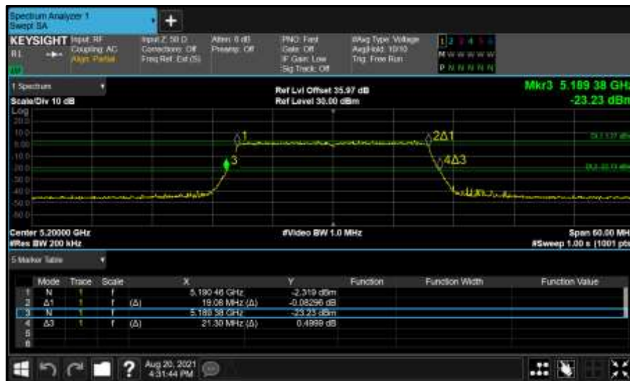
Figure 155 - Core 0 (A) 5200 MHz (CH40) 26 dB and 99% Bandwidth
