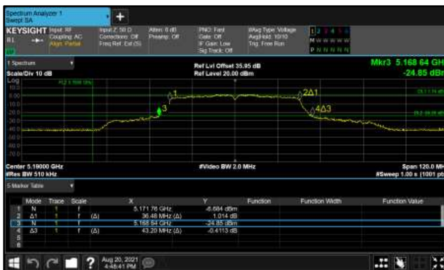
Figure 129 - Core 0 (A) 5190 MHz (CH38) 26 dB and 99% Bandwidth
