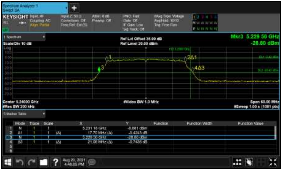
Figure 108 - Core 1 (B) 5240 MHz (CH48) 26 dB and 99% Bandwidth
