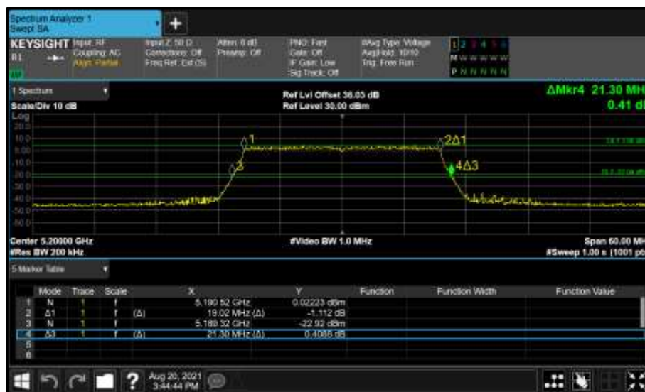
Figure 160 - Core 1 (B) 5200 MHz (CH40) 26 dB and 99% Bandwidth
