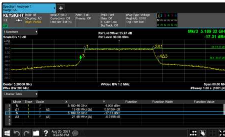
Figure 152 - Core 0 (A) 5200 MHz (CH40) 26 dB and 99% Bandwidth
