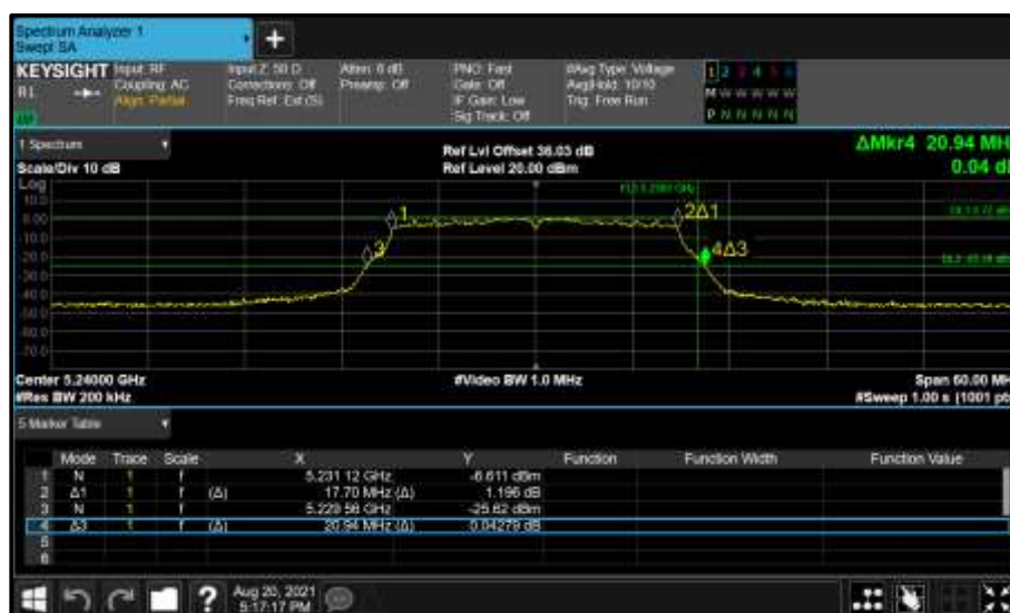
Figure 119 - Core 0 (A) 5240 MHz (CH48) 26 dB and 99% Bandwidth
