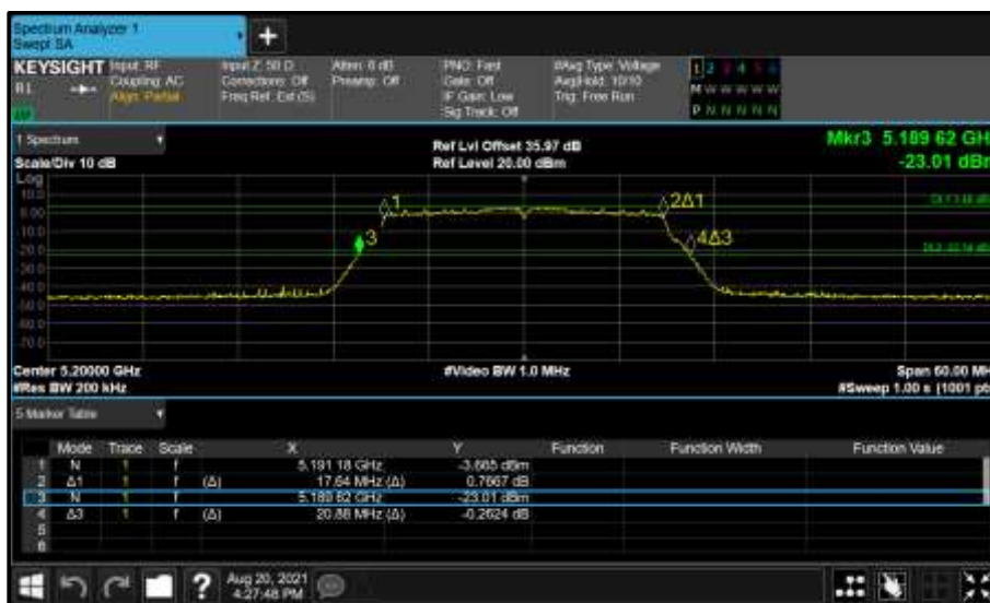
Figure 95 - Core 0 (A) 5200 MHz (CH40) 26 dB and 99% Bandwidth
