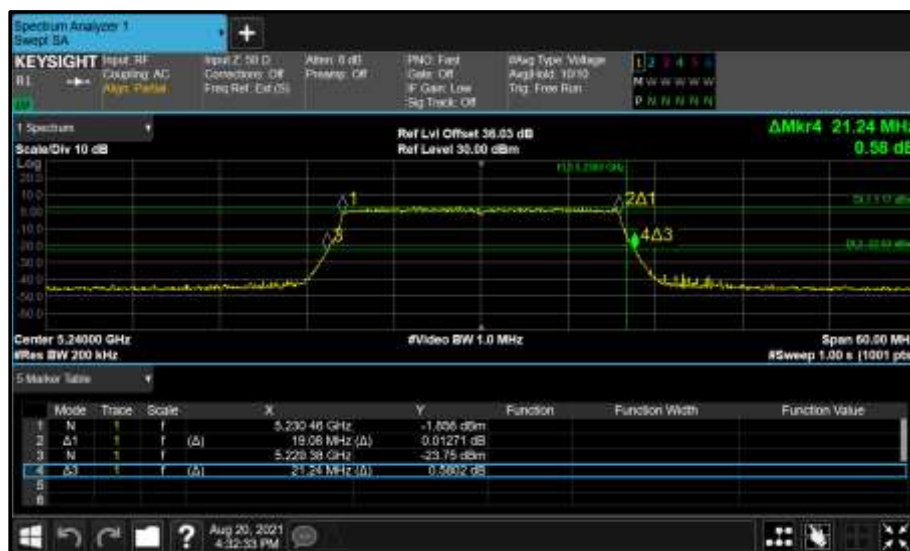
Figure 156 - Core 0 (A) 5240 MHz (CH48) 26 dB and 99% Bandwidth
