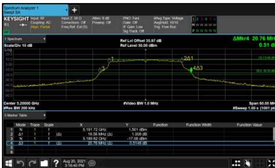
Figure 86 - Core 0 (A) 5200 MHz (CH40) 26 dB and 99% Bandwidth
