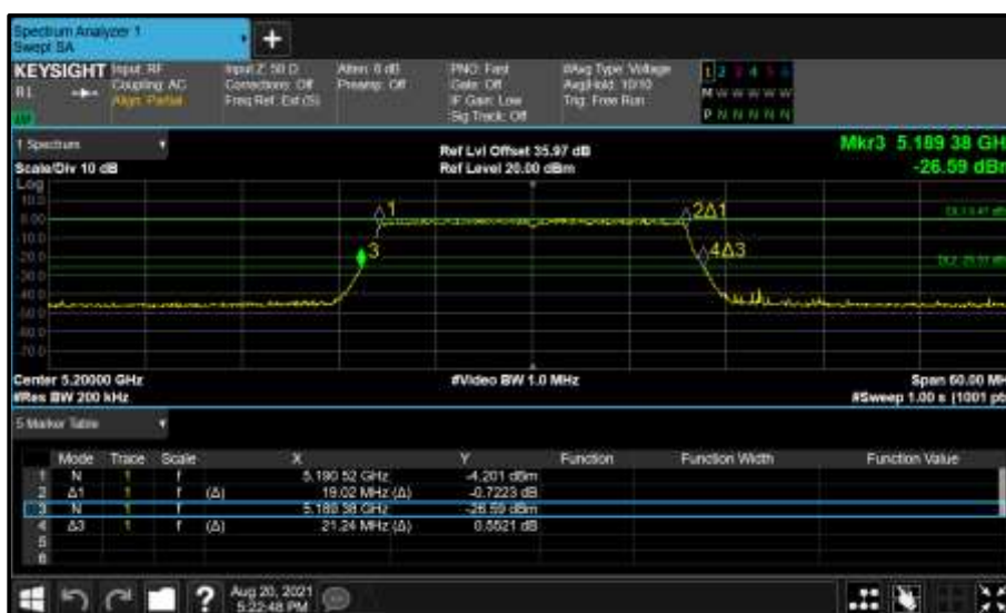
Figure 177 - Core 0 (A) 5200 MHz (CH40) 26 dB and 99% Bandwidth
