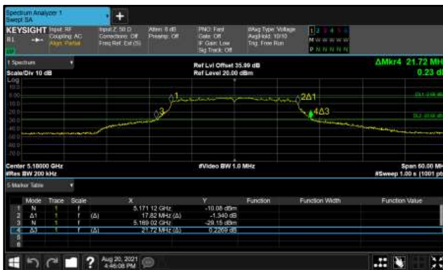
Figure 104 - Core 1 (B) 5180 MHz (CH36) 26 dB and 99% Bandwidth
