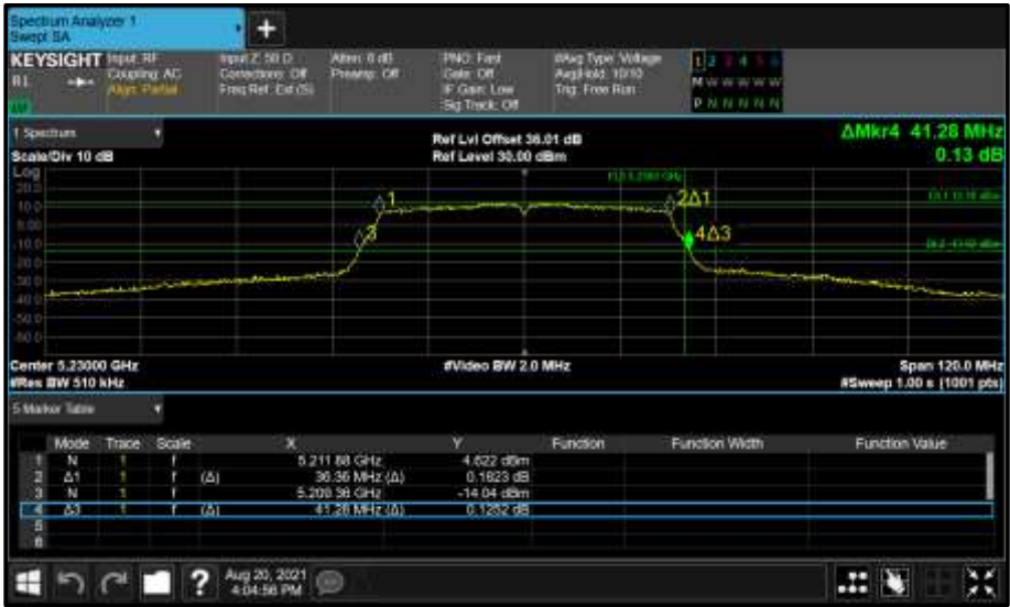
Figure 136 - Core 1 (B) 5230 MHz (CH46) 26 dB and 99% Bandwidth
