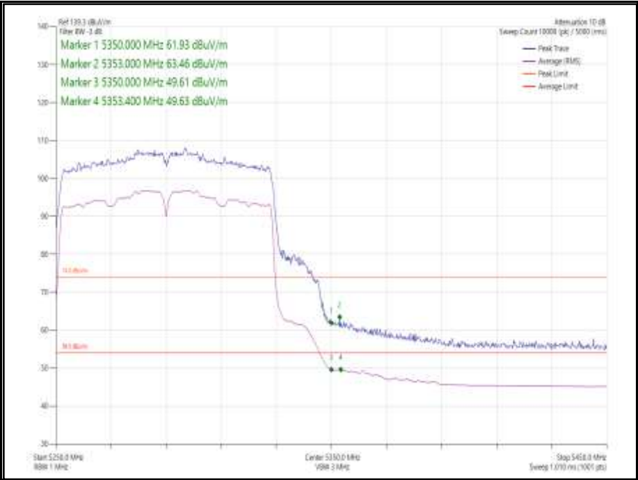
Figure 59 - 802.11ac VHT80, Core 0 - 5290 MHz Band Edge Frequency 5350 MHz
