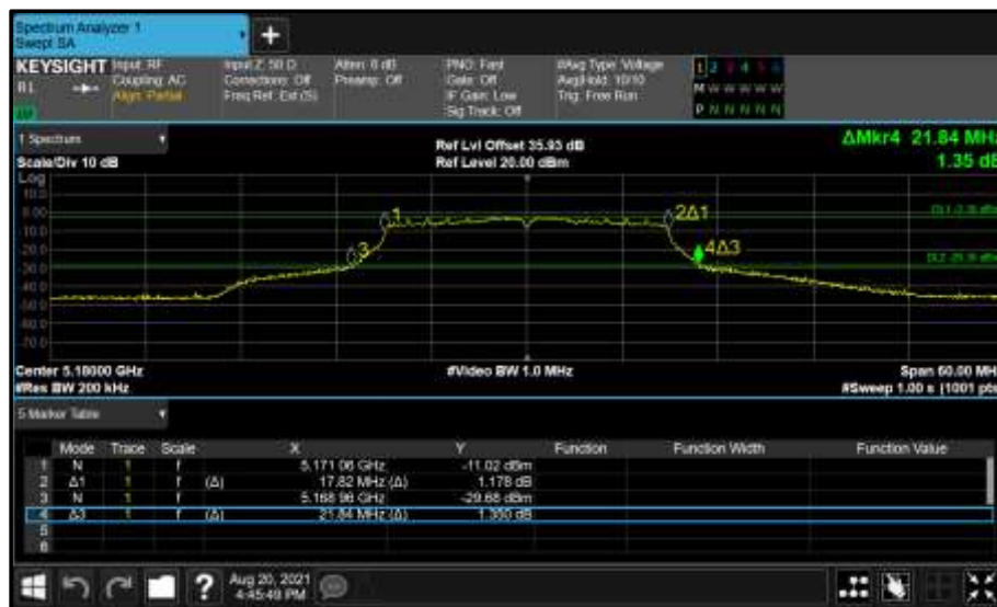
Figure 103 - Core 0 (A) 5180 MHz (CH36) 26 dB and 99% Bandwidth
