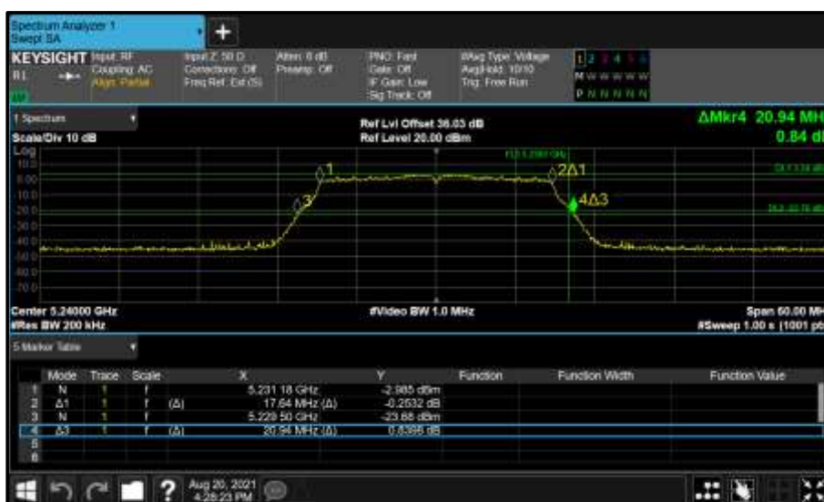
Figure 96 - Core 0 (A) 5240 MHz (CH48) 26 dB and 99% Bandwidth
