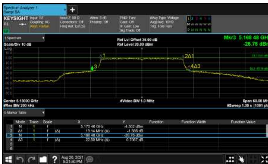
Figure 176 - Core 1 (B) 5180 MHz (CH36) 26 dB and 99% Bandwidth
