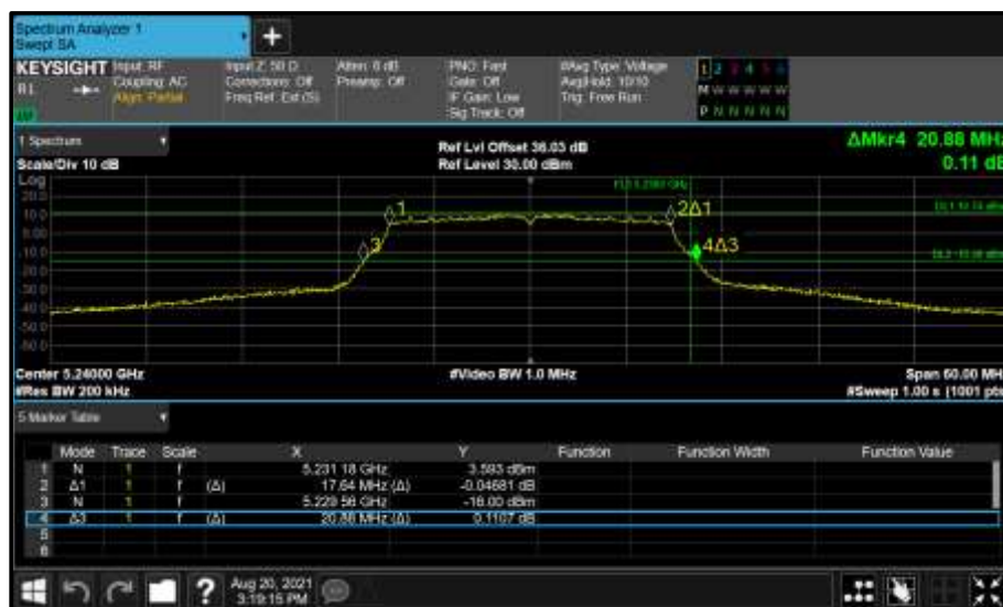
Figure 93 - Core 0 (A) 5240 MHz (CH48) 26 dB and 99% Bandwidth
