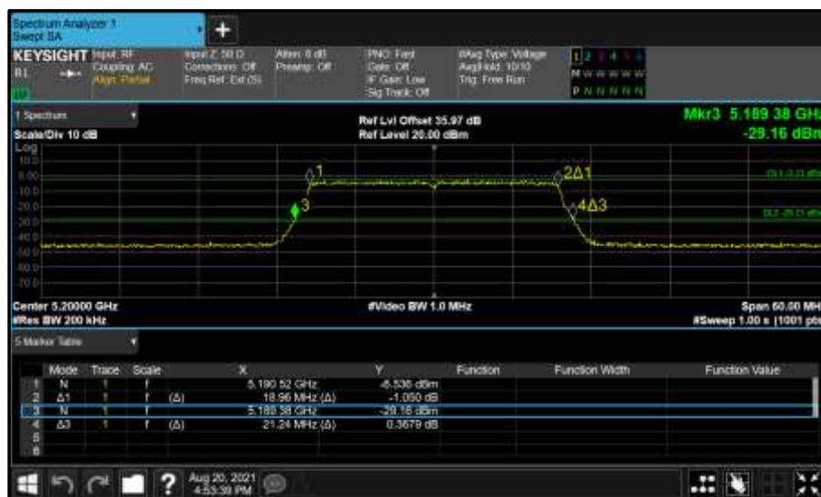
Figure 165 - Core 0 (A) 5200 MHz (CH40) 26 dB and 99% Bandwidth
