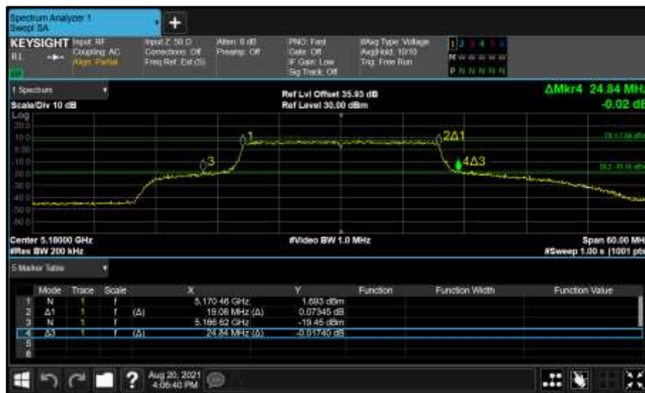
Figure 169 - Core 0 (A) 5180 MHz (CH36) 26 dB and 99% Bandwidth
