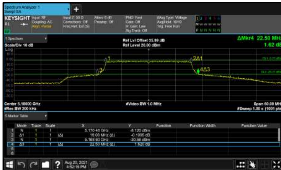
Figure 164 - Core 1 (B) 5180 MHz (CH36) 26 dB and 99% Bandwidth
