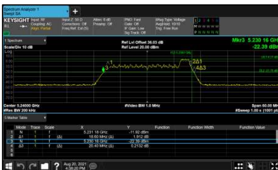
Figure 186 - Core 0 (A) 5240 MHz (CH48) 26 dB and 99% Bandwidth
