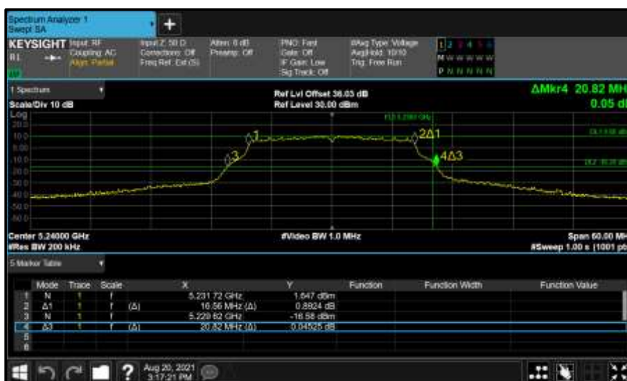
Figure 87 - Core 0 (A) 5240 MHz (CH48) 26 dB and 99% Bandwidth
