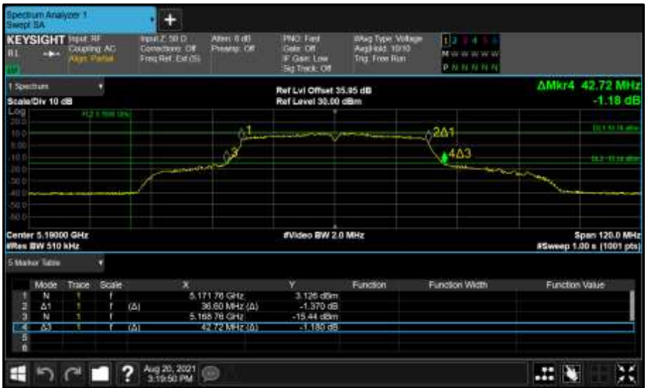
Figure 121 - Core 0 (A) 5190 MHz (CH38) 26 dB and 99% Bandwidth
