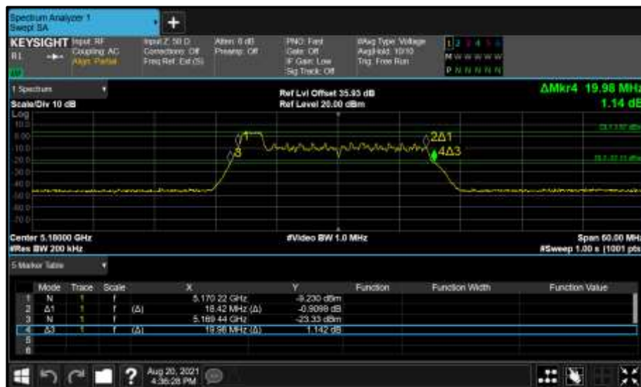
Figure 184 - Core 0 (A) 5180 MHz (CH36) 26 dB and 99% Bandwidth
