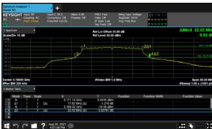
Figure 110 - Core 1 (B) 5180 MHz (CH36) 26 dB and 99% Bandwidth
