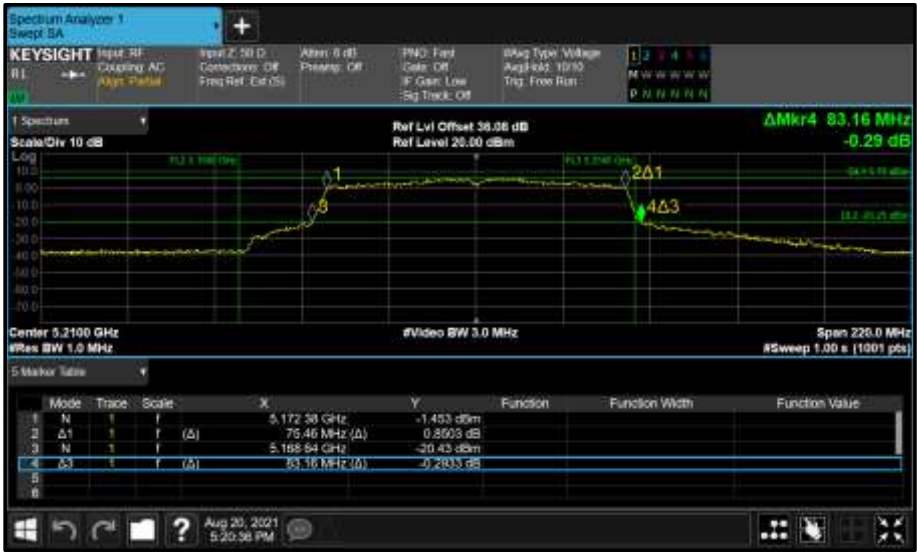
Figure 150 - Core 1 (B) 5210 MHz (CH42) 26 dB and 99% Bandwidth
