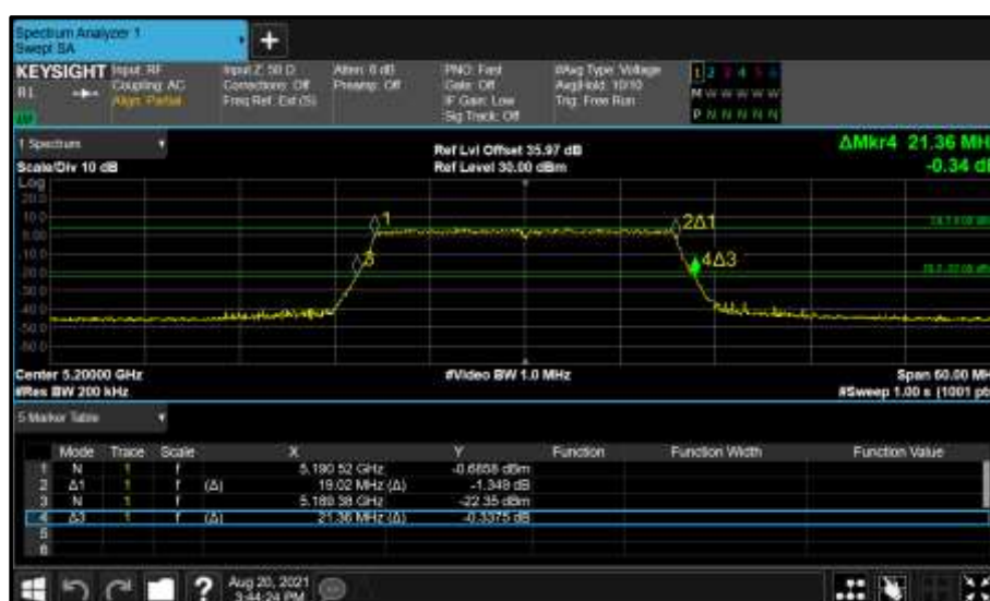
Figure 159 - Core 0 (A) 5200 MHz (CH40) 26 dB and 99% Bandwidth
