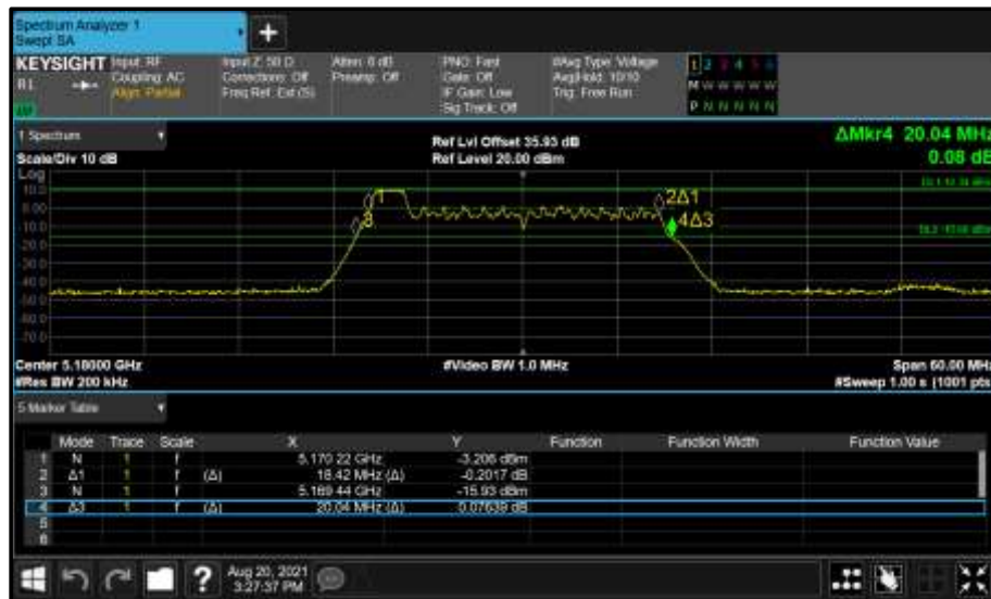
Figure 181 - Core 0 (A) 5180 MHz (CH36) 26 dB and 99% Bandwidth
