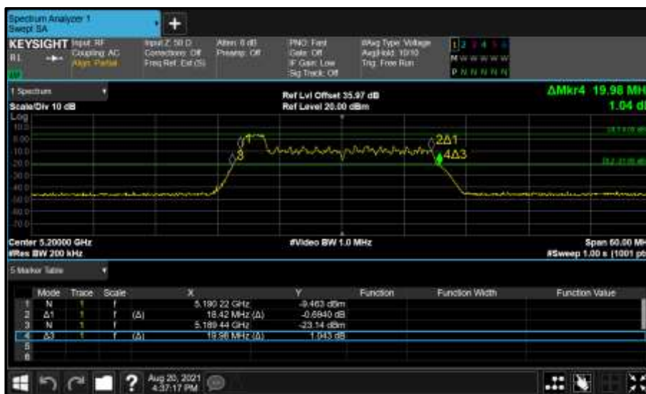
Figure 185 - Core 0 (A) 5200 MHz (CH40) 26 dB and 99% Bandwidth
