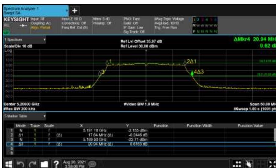
Figure 99 - Core 0 (A) 5200 MHz (CH40) 26 dB and 99% Bandwidth
