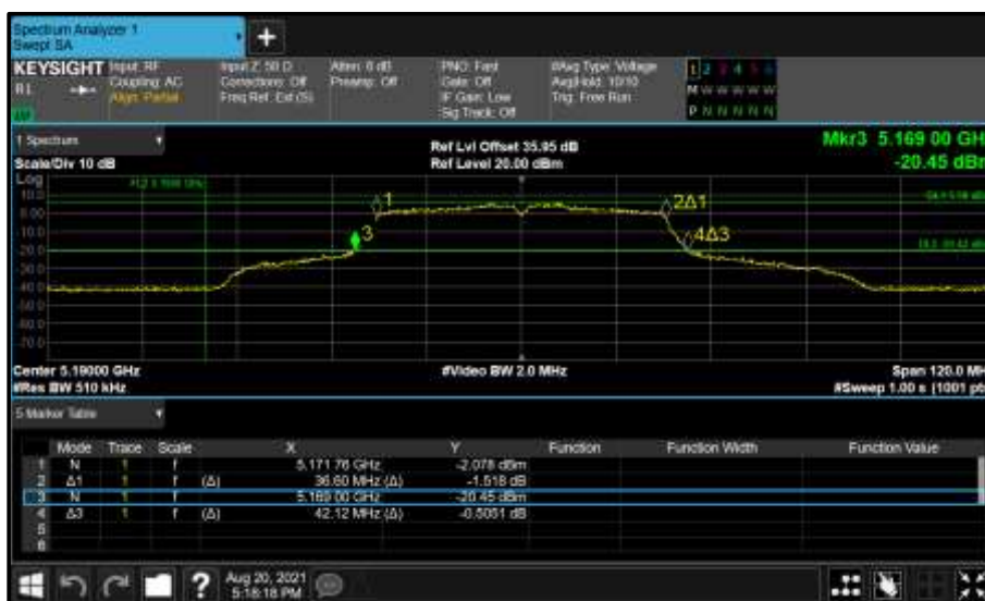
Figure 137 - Core 0 (A) 5190 MHz (CH38) 26 dB and 99% Bandwidth
