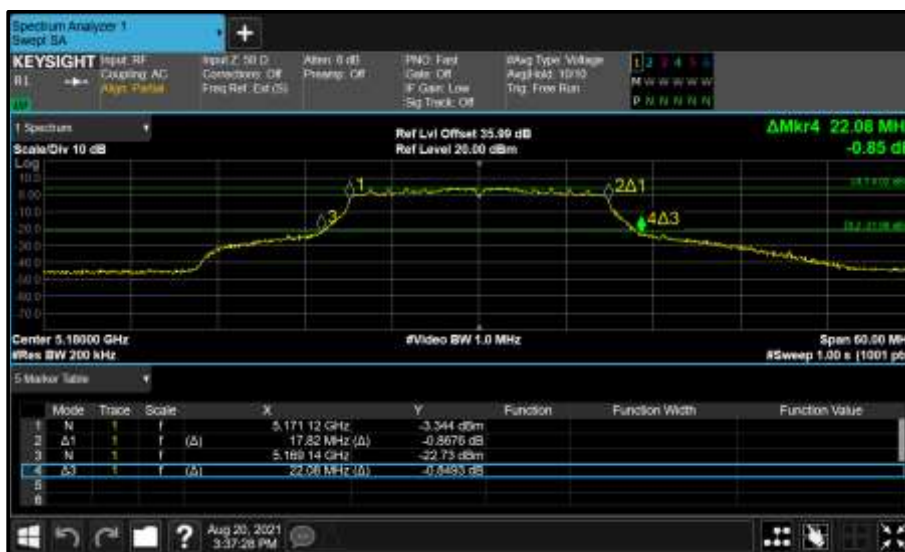
Figure 98 - Core 1 (B) 5180 MHz (CH36) 26 dB and 99% Bandwidth
