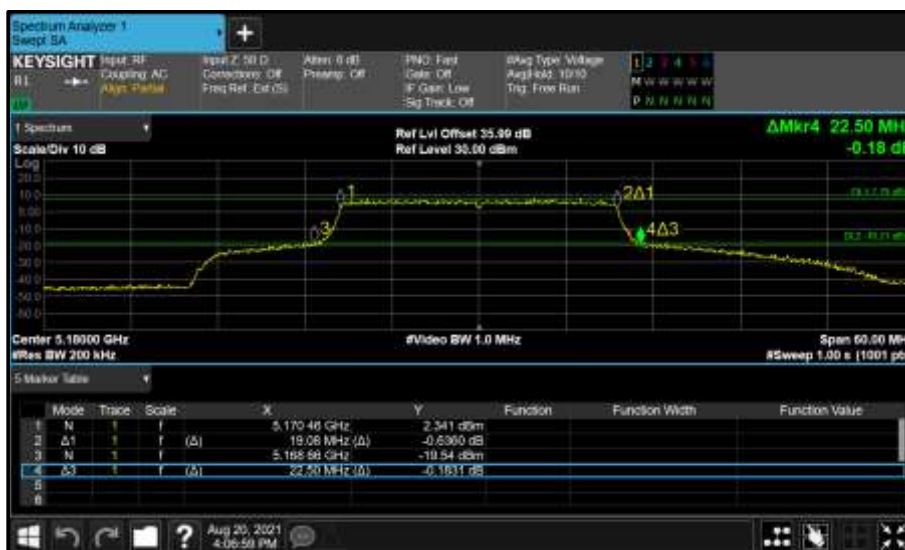
Figure 170 - Core 1 (B) 5180 MHz (CH36) 26 dB and 99% Bandwidth
