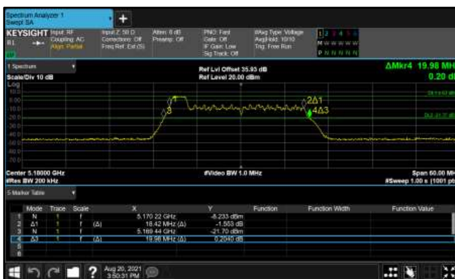
Figure 187 - Core 0 (A) 5180 MHz (CH36) 26 dB and 99% Bandwidth
