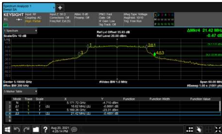
Figure 88 - Core 0 (A) 5180 MHz (CH36) 26 dB and 99% Bandwidth
