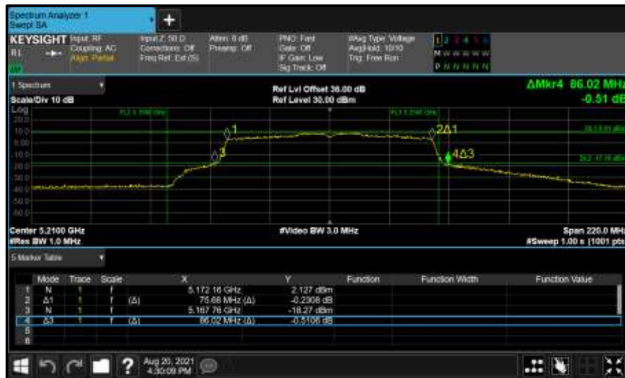
Figure 142 - Core 0 (A) 5210 MHz (CH42) 26 dB and 99% Bandwidth
