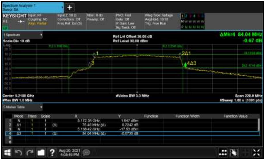
Figure 148 - Core 1 (B) 5210 MHz (CH42) 26 dB and 99% Bandwidth
