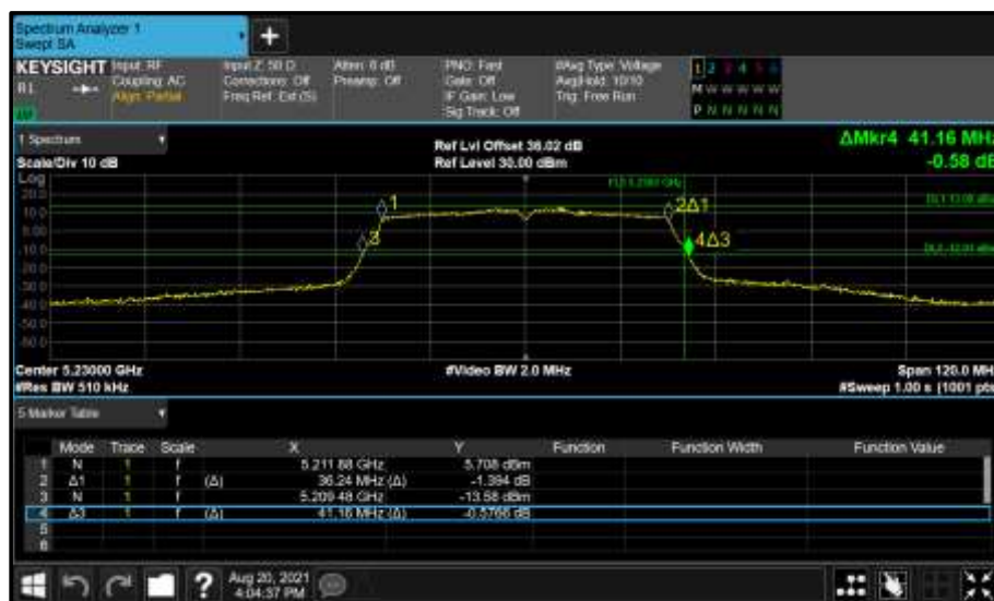
Figure 135 - Core 0 (A) 5230 MHz (CH46) 26 dB and 99% Bandwidth
