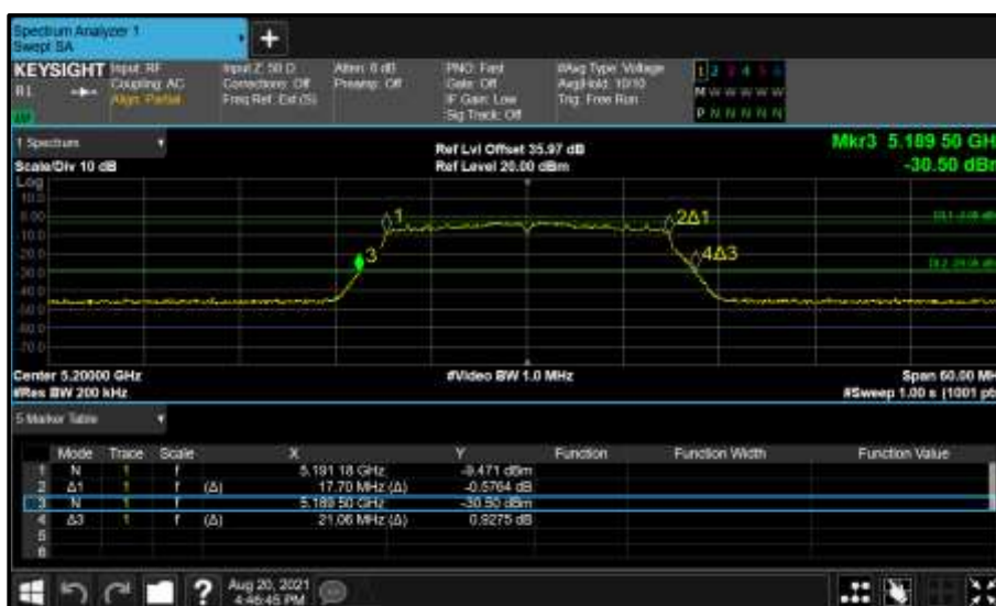
Figure 105 - Core 0 (A) 5200 MHz (CH40) 26 dB and 99% Bandwidth
