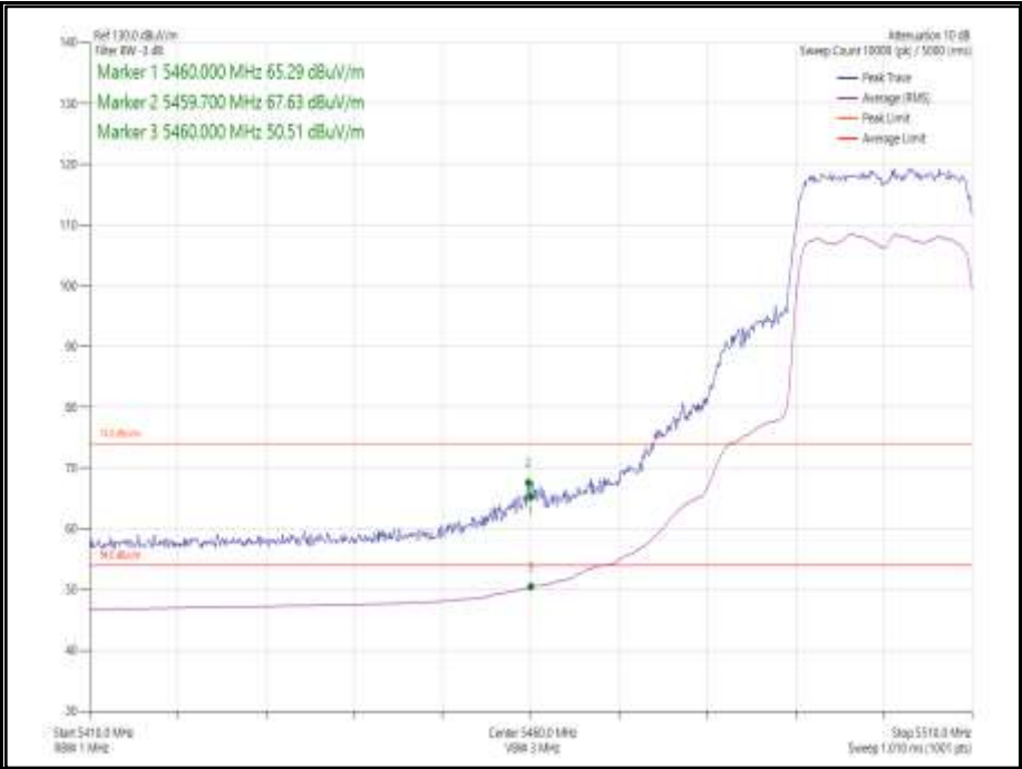
Figure 29 - 802.11ax HE20 SDM, Cores 0-1, SU- 5500 MHz Band Edge Frequency 5460 MHz
