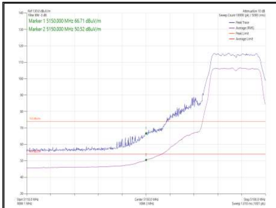
Figure 1 - 802.11a, Core 0 - 5180 MHz, Band Edge Frequency 5150 MHz
