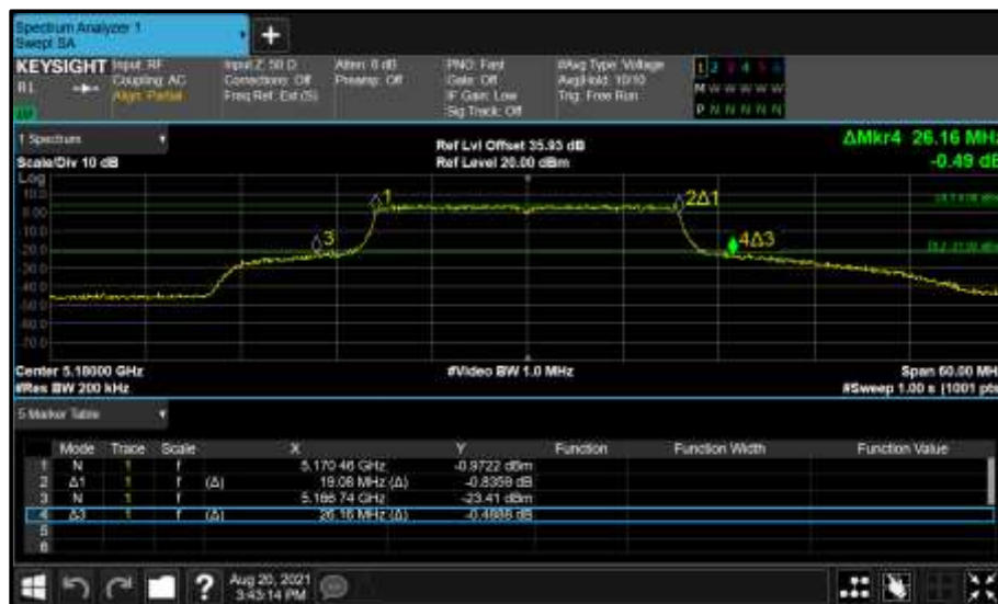
Figure 157 - Core 0 (A) 5180 MHz (CH36) 26 dB and 99% Bandwidth
