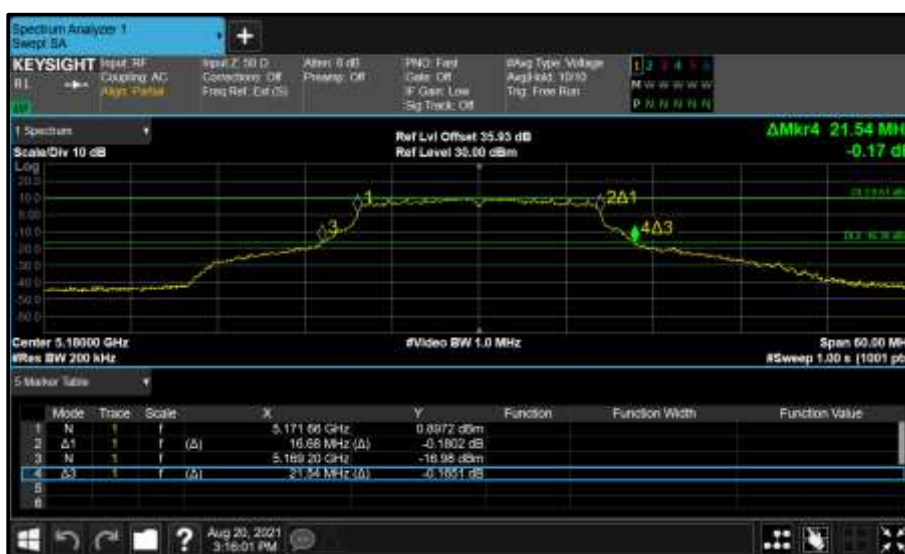
Figure 85 - Core 0 (A) 5180 MHz (CH36) 26 dB and 99% Bandwidth
