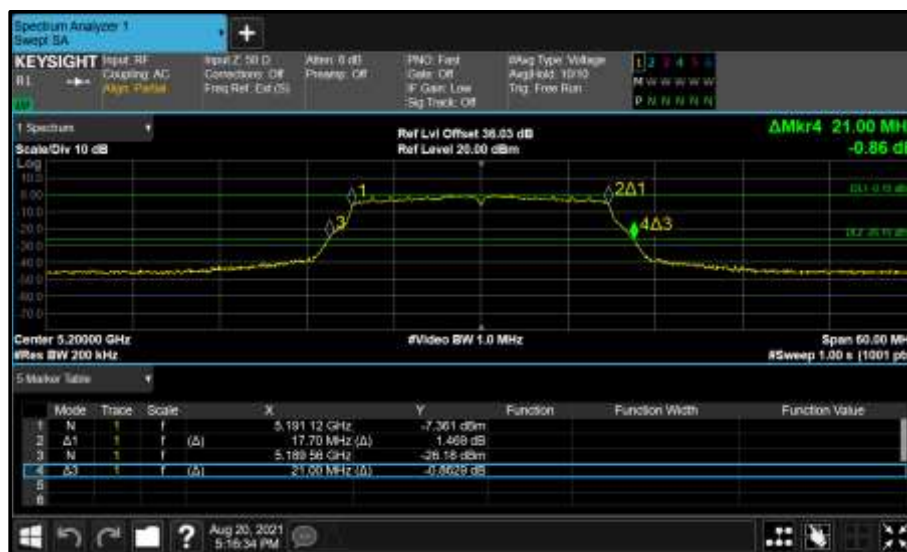
Figure 118 - Core 1 (B) 5200 MHz (CH40) 26 dB and 99% Bandwidth
