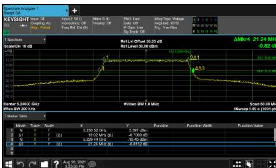
Figure 153 - Core 0 (A) 5240 MHz (CH48) 26 dB and 99% Bandwidth
