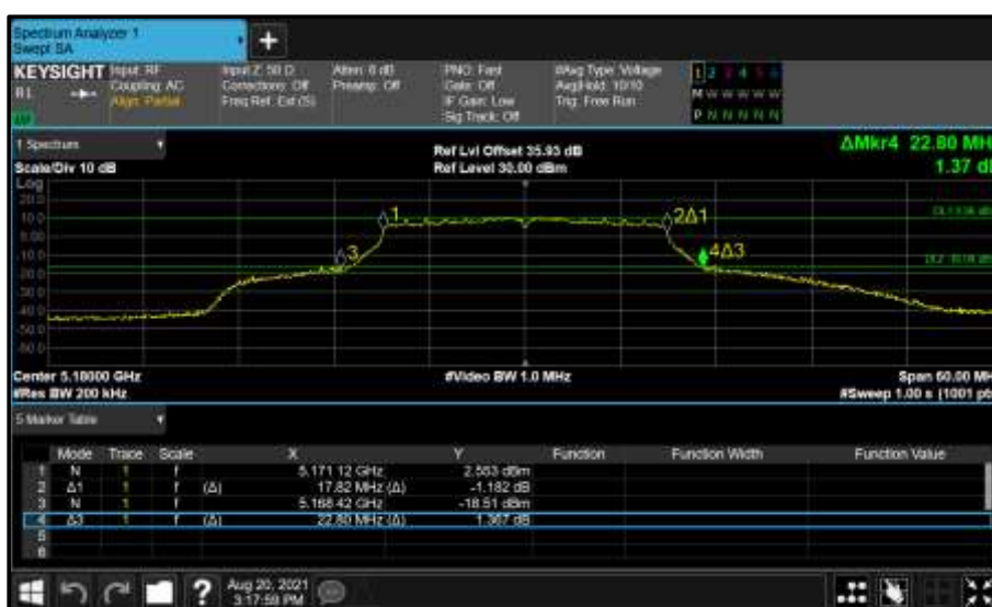
Figure 91 - Core 0 (A) 5180 MHz (CH36) 26 dB and 99% Bandwidth
