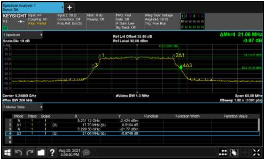
Figure 102 - Core 1 (B) 5240 MHz (CH48) 26 dB and 99% Bandwidth
