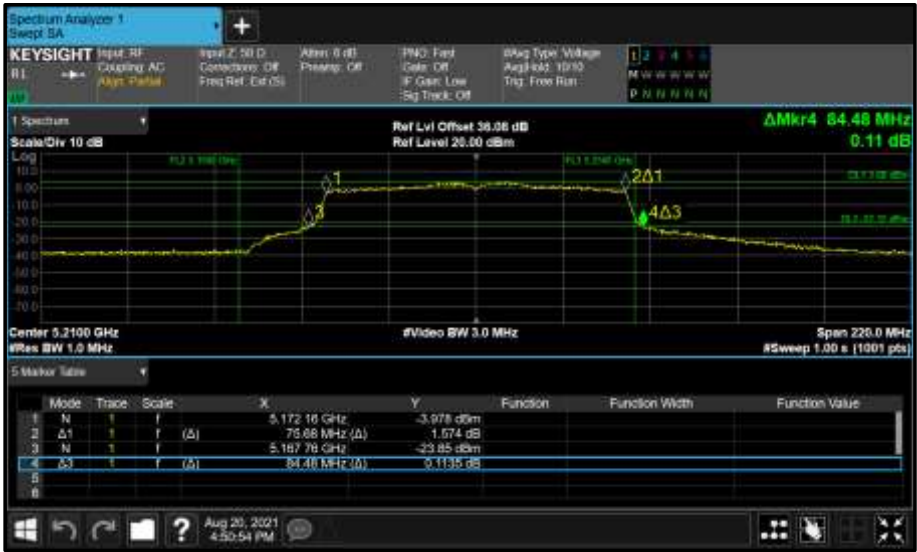
Figure 146 - Core 1 (B) 5210 MHz (CH42) 26 dB and 99% Bandwidth
