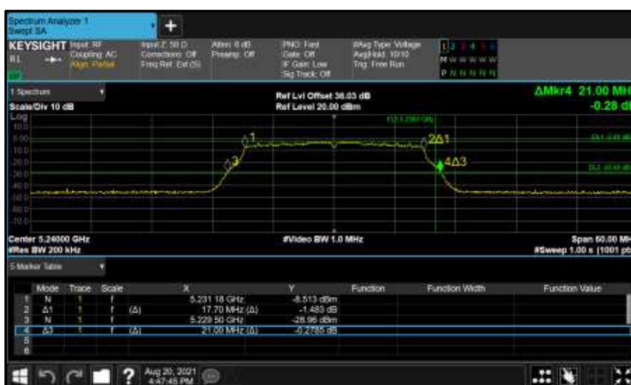
Figure 107 - Core 0 (A) 5240 MHz (CH48) 26 dB and 99% Bandwidth
