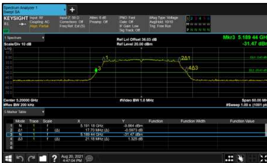
Figure 106 - Core 1 (B) 5200 MHz (CH40) 26 dB and 99% Bandwidth
