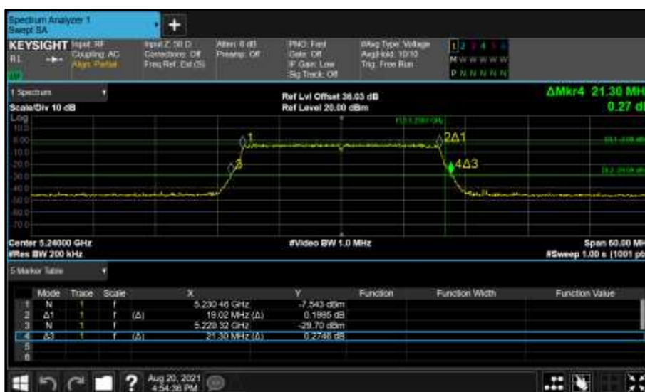
Figure 167 - Core 0 (A) 5240 MHz (CH48) 26 dB and 99% Bandwidth
