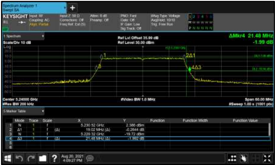
Figure 174 - Core 1 (B) 5240 MHz (CH48) 26 dB and 99% Bandwidth
