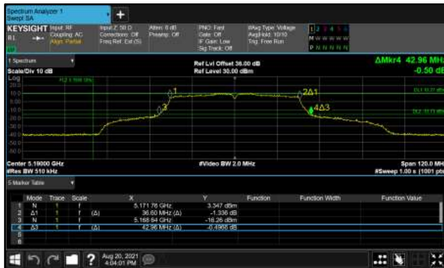
Figure 134 - Core 1 (B) 5190 MHz (CH38) 26 dB and 99% Bandwidth
