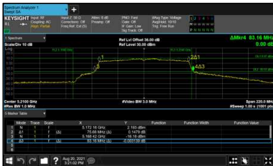
Figure 141 - Core 0 (A) 5210 MHz (CH42) 26 dB and 99% Bandwidth
