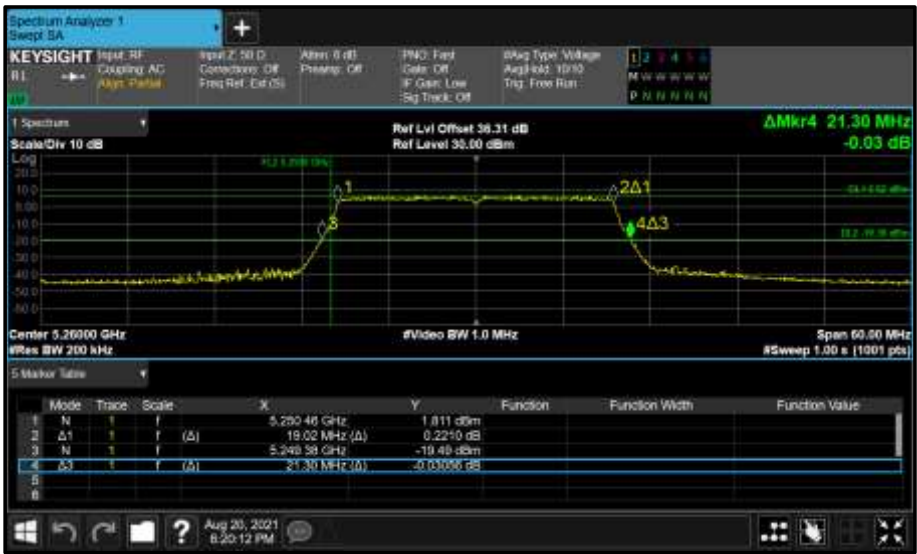
Figure 367 - Core 0 (A) 5260 MHz (CH52) 26 dB and 99% Bandwidth
