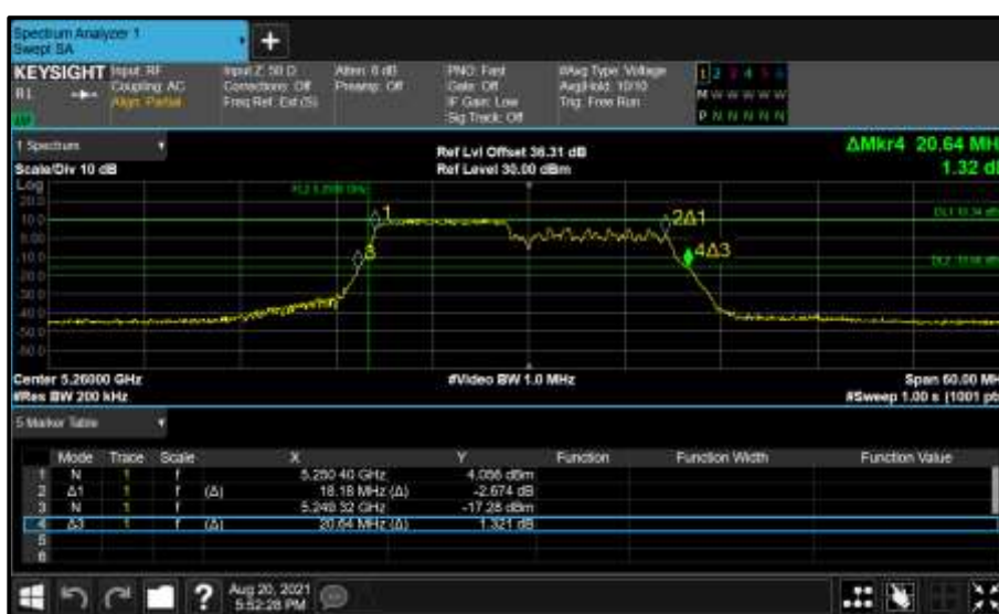
Figure 388 - Core 0 (A) 5260 MHz (CH52) 26 dB and 99% Bandwidth
