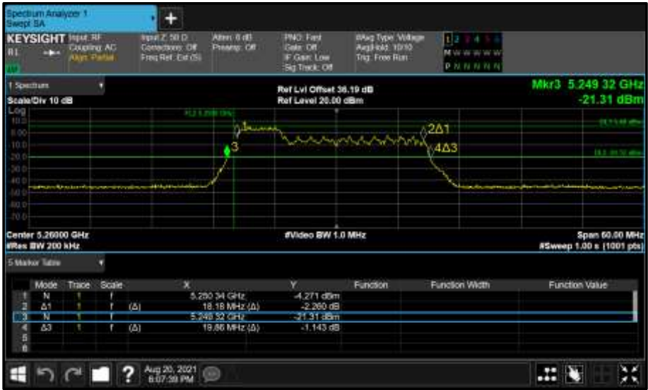
Figure 377 - Core 1 (B) 5260 MHz (CH52) 26 dB and 99% Bandwidth
