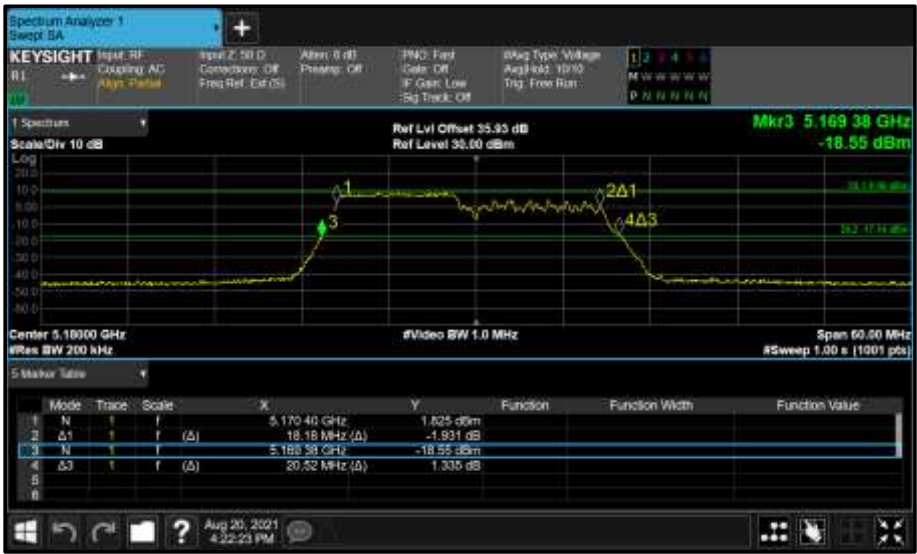
Figure 259 - Core 0 (A) 5180 MHz (CH36) 26 dB and 99% Bandwidth
