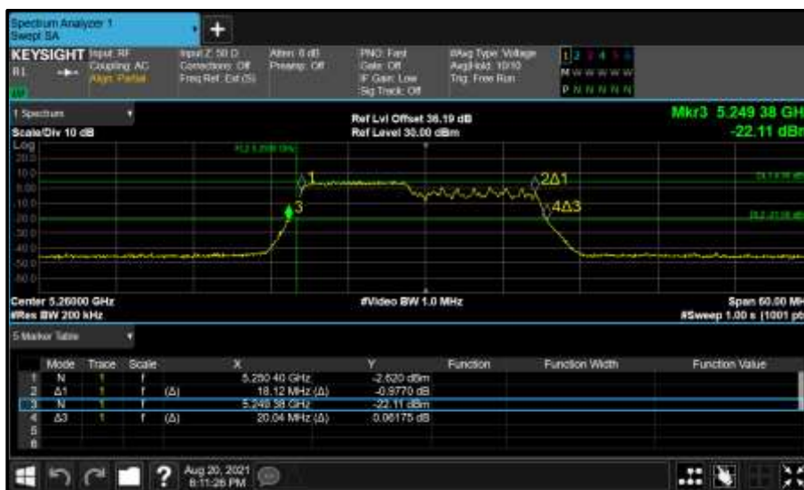
Figure 392 - Core 1 (B) 5260 MHz (CH52) 26 dB and 99% Bandwidth
