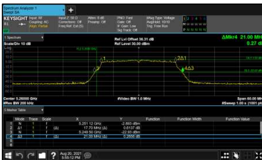
Figure 331 - Core 0 (A) 5260 MHz (CH52) 26 dB and 99% Bandwidth
