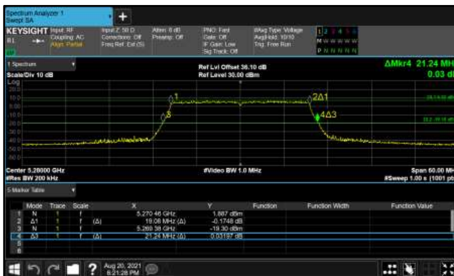
Figure 370 - Core 1 (B) 5280 MHz (CH56) 26 dB and 99% Bandwidth
