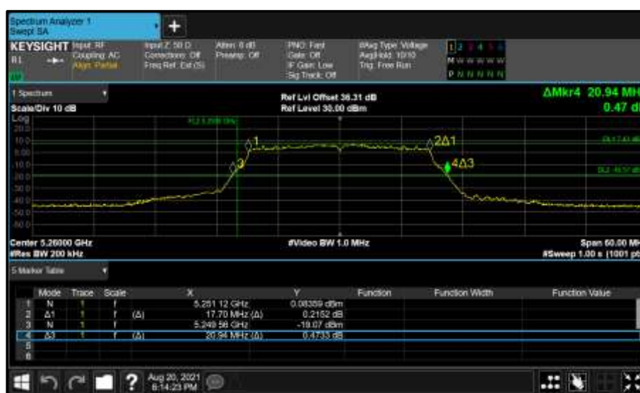
Figure 337 - Core 0 (A) 5260 MHz (CH52) 26 dB and 99% Bandwidth
