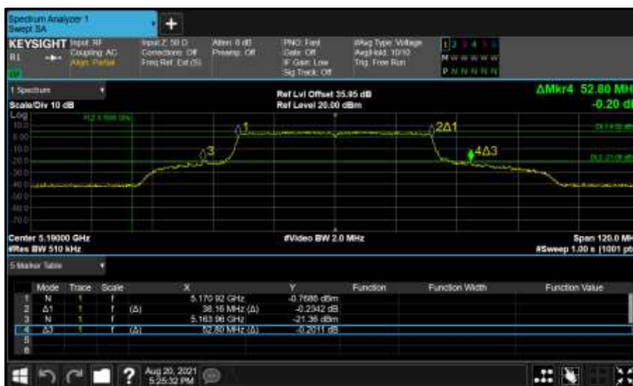
Figure 287 - Core 0 (A) 5190 MHz (CH38) 26 dB and 99% Bandwidth
