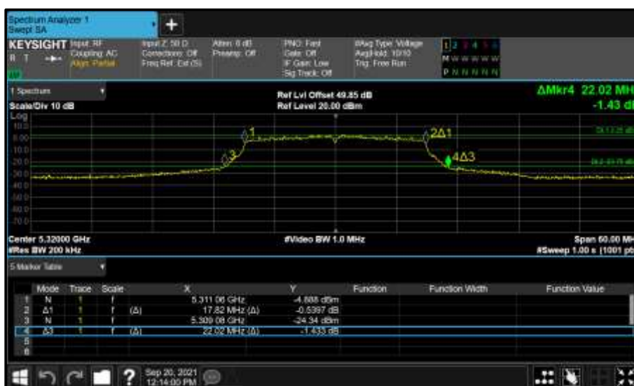
Figure 422 - Core 0 (A) 5320 MHz (CH64) 26 dB and 99% Bandwidth
