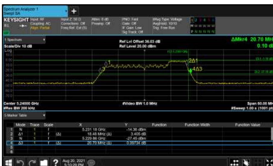
Figure 227 - Core 0 (A) 5240 MHz (CH48) 26 dB and 99% Bandwidth
