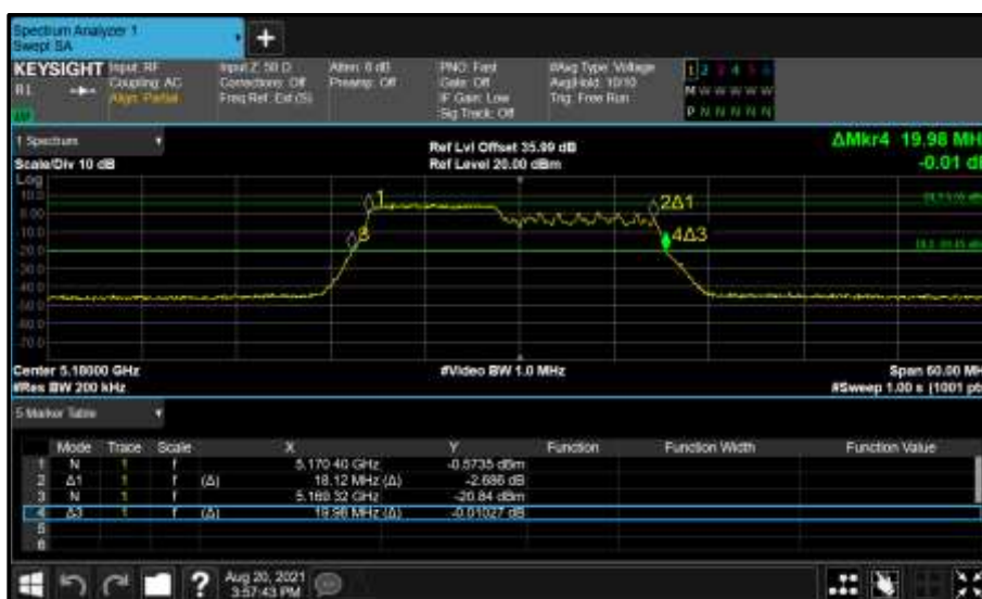
Figure 248 - Core 1 (B) 5180 MHz (CH36) 26 dB and 99% Bandwidth
