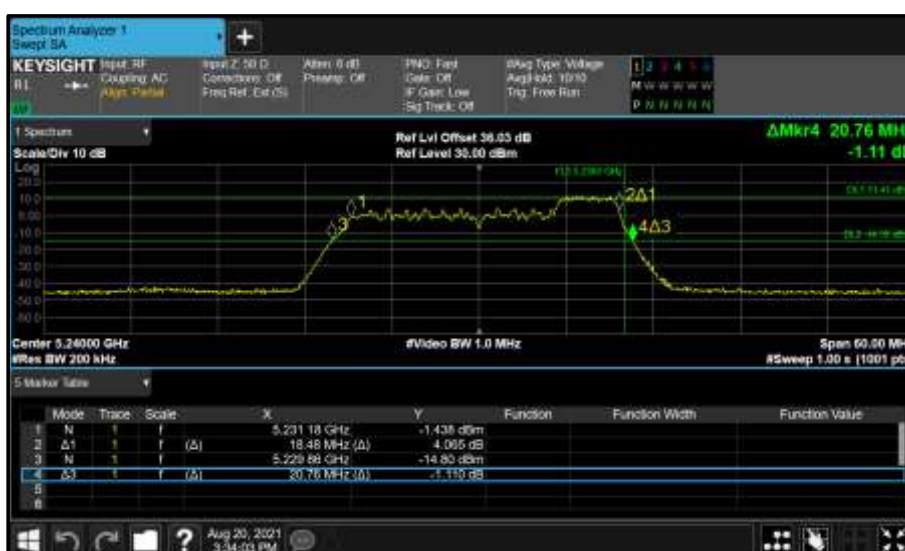
Figure 213 - Core 0 (A) 5240 MHz (CH48) 26 dB and 99% Bandwidth
