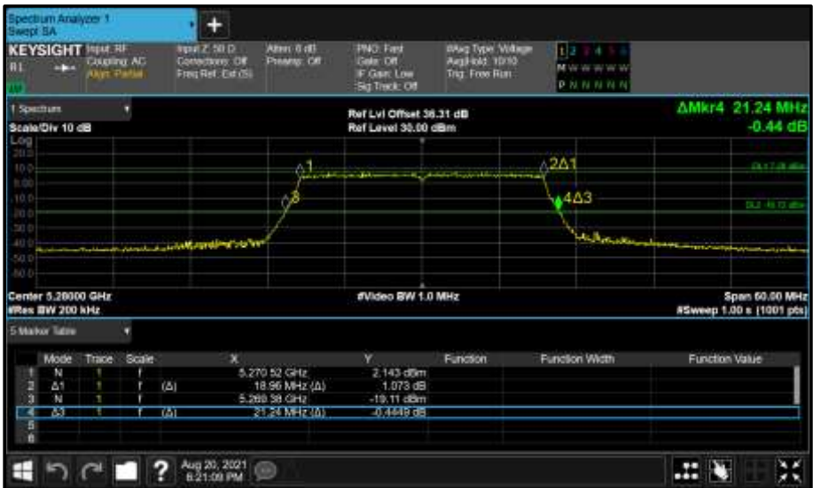
Figure 369 - Core 0 (A) 5280 MHz (CH56) 26 dB and 99% Bandwidth
