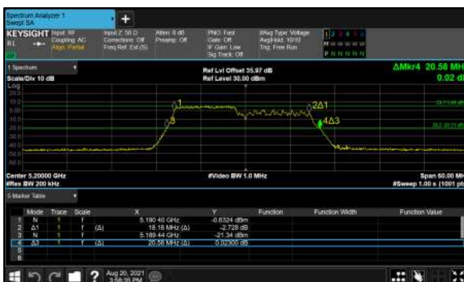
Figure 249 - Core 0 (A) 5200 MHz (CH40) 26 dB and 99% Bandwidth
