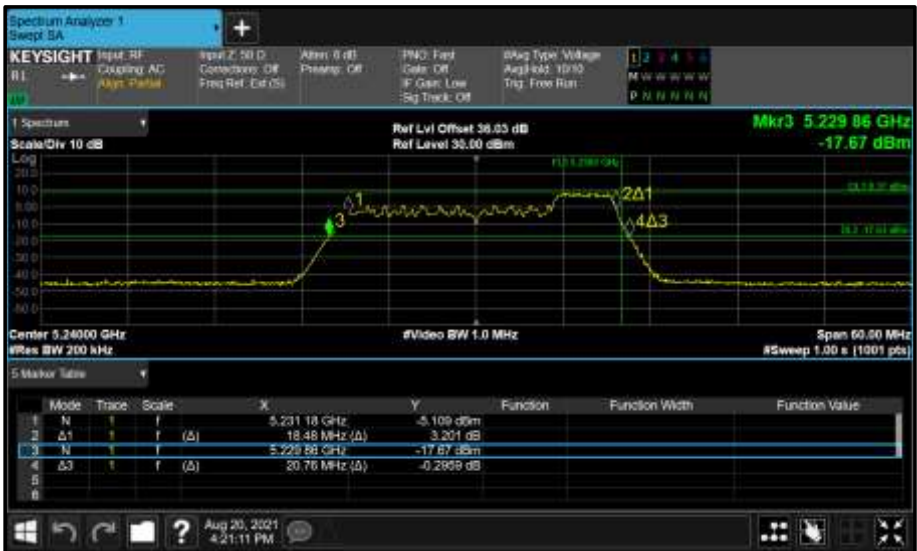
Figure 233 - Core 0 (A) 5240 MHz (CH48) 26 dB and 99% Bandwidth
