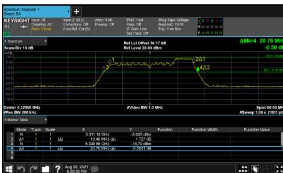
Figure 386 - Core 0 (A) 5320 MHz (CH64) 26 dB and 99% Bandwidth
