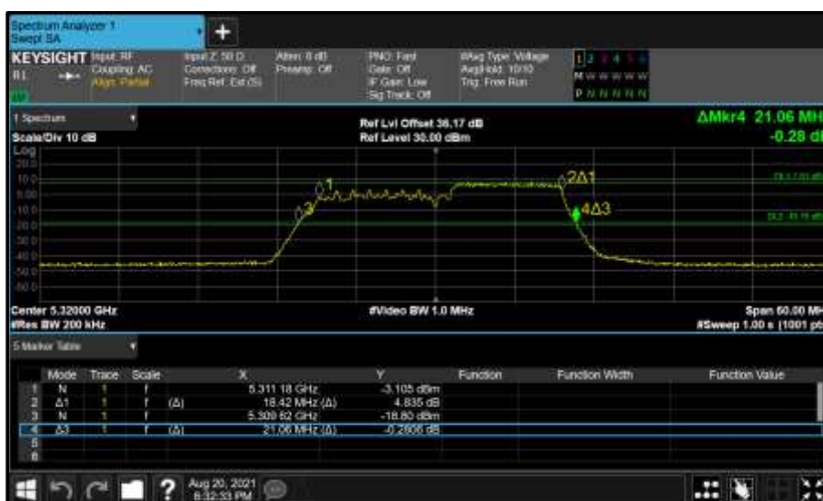
Figure 401 - Core 0 (A) 5320 MHz (CH64) 26 dB and 99% Bandwidth
