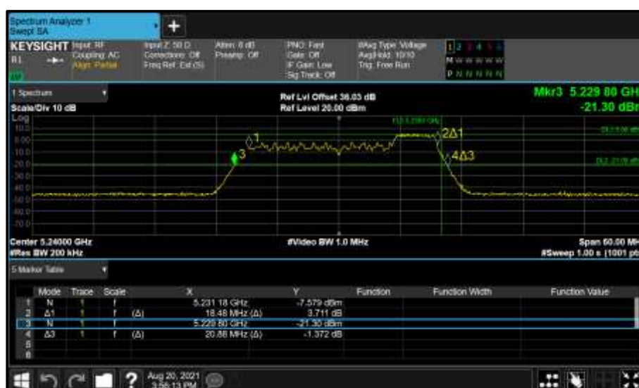
Figure 221 - Core 0 (A) 5240 MHz (CH48) 26 dB and 99% Bandwidth
