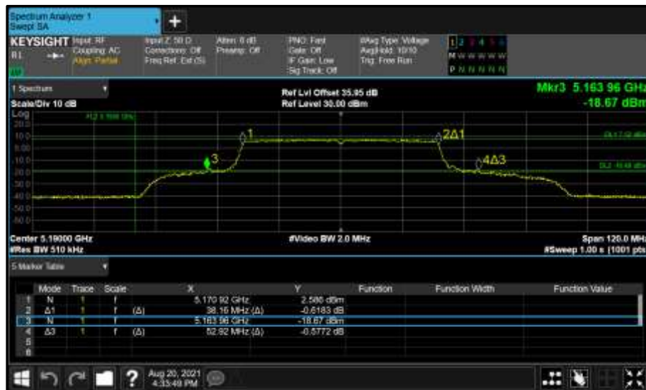
Figure 273 - Core 0 (A) 5190 MHz (CH38) 26 dB and 99% Bandwidth
