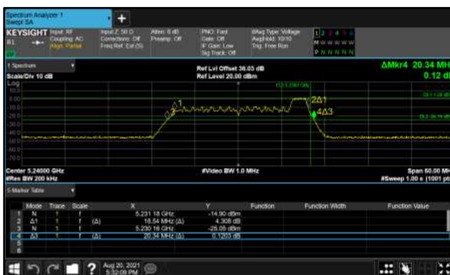
Figure 209 - Core 0 (A) 5240 MHz (CH48) 26 dB and 99% Bandwidth
