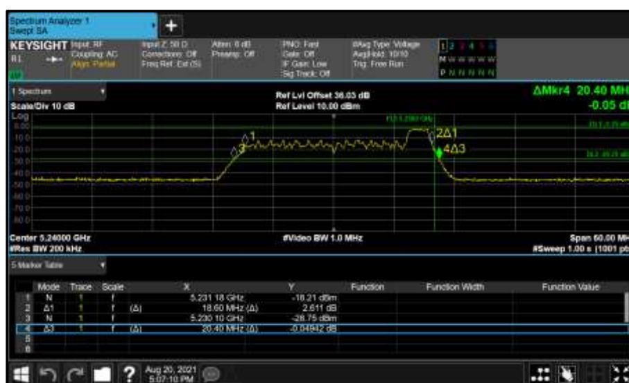
Figure 197 - Core 0 (A) 5240 MHz (CH48) 26 dB and 99% Bandwidth
