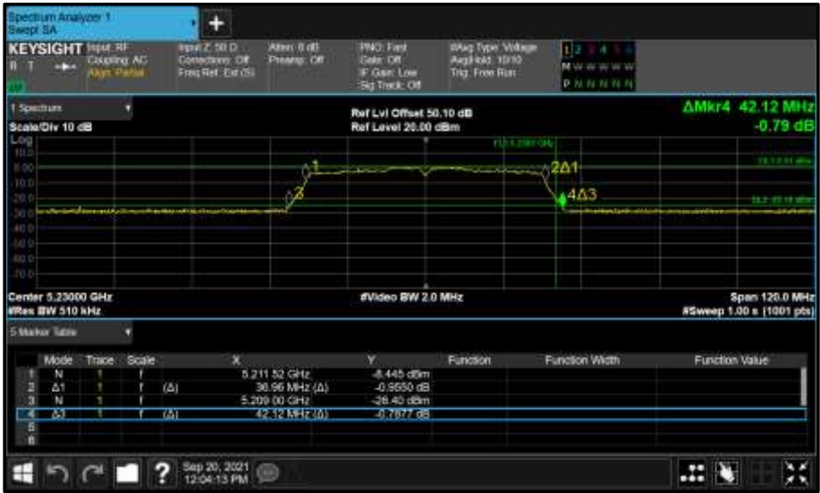
Figure 320 - Core 1 (B) 5230 MHz (CH46) 26 dB and 99% Bandwidth
