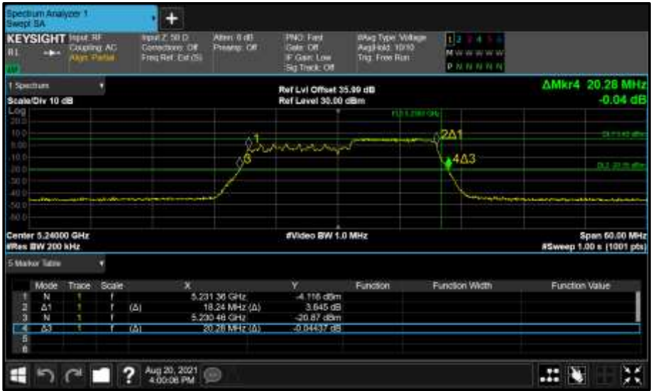
Figure 252 - Core 1 (B) 5240 MHz (CH48) 26 dB and 99% Bandwidth
