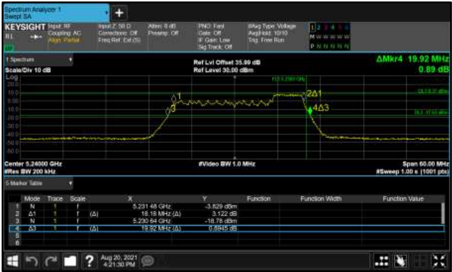
Figure 234 - Core 1 (B) 5240 MHz (CH48) 26 dB and 99% Bandwidth
