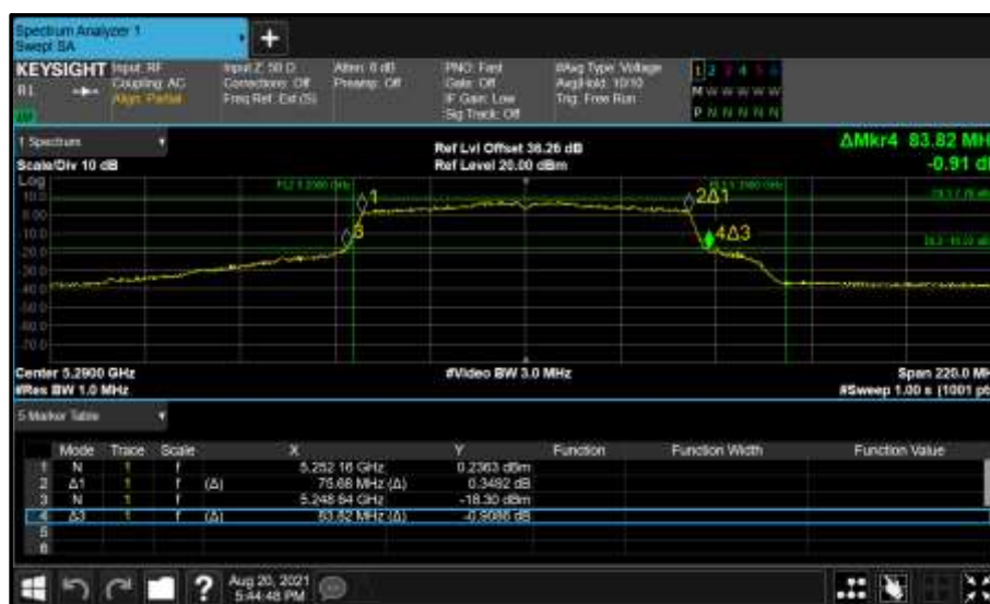
Figure 353 - Core 0 (A) 5290 MHz (CH58) 26 dB and 99% Bandwidth
