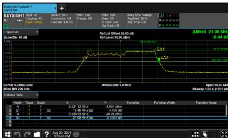
Figure 251 - Core 0 (A) 5240 MHz (CH48) 26 dB and 99% Bandwidth
