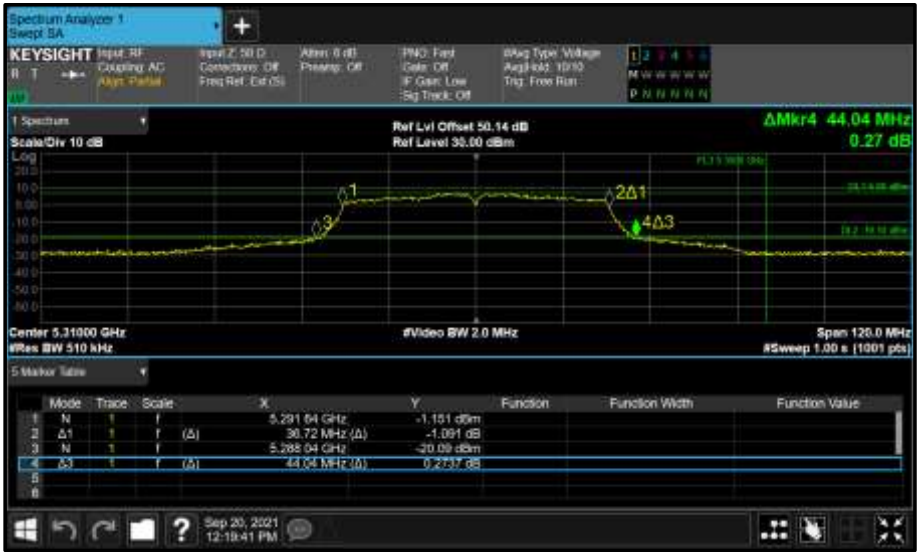
Figure 427 - Core 1 (B) 5310 MHz (CH62) 26 dB and 99% Bandwidth
