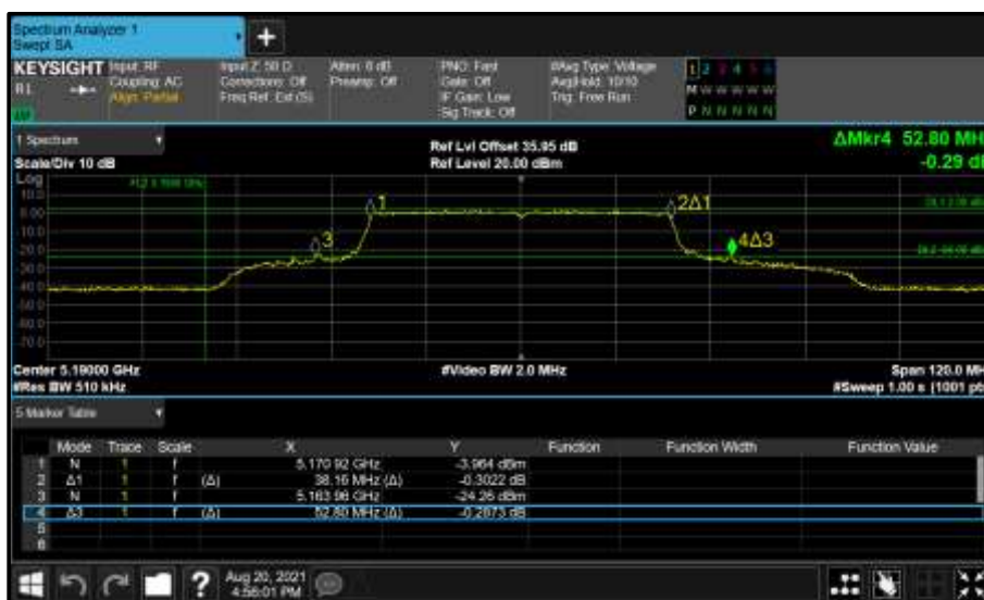
Figure 279 - Core 0 (A) 5190 MHz (CH38) 26 dB and 99% Bandwidth
