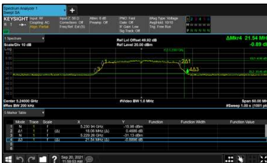
Figure 311 - Core 0 (A) 5240 MHz (CH48) 26 dB and 99% Bandwidth
