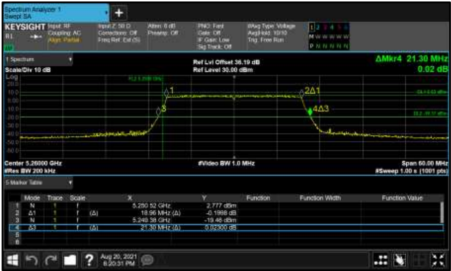
Figure 368 - Core 1 (B) 5260 MHz (CH52) 26 dB and 99% Bandwidth
