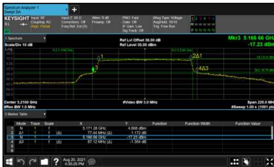
Figure 292 - Core 0 (A) 5210 MHz (CH42) 26 dB and 99% Bandwidth
