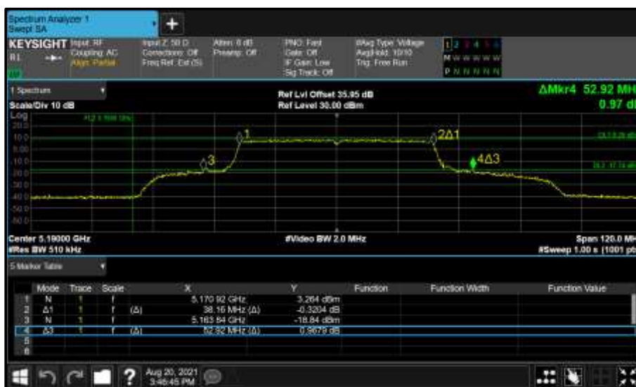
Figure 275 - Core 0 (A) 5190 MHz (CH38) 26 dB and 99% Bandwidth
