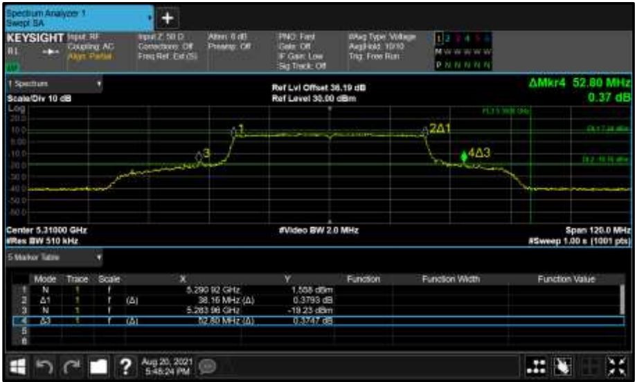
Figure 404 - Core 0 (A) 5310 MHz (CH62) 26 dB and 99% Bandwidth
