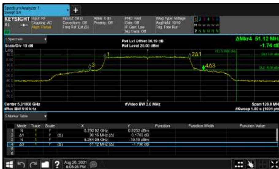
Figure 407 - Core 0 (A) 5310 MHz (CH62) 26 dB and 99% Bandwidth
