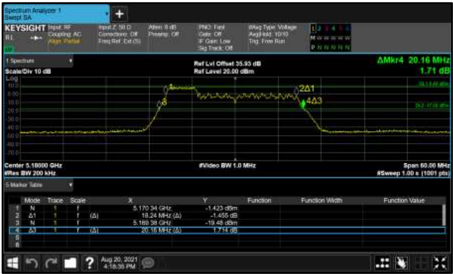
Figure 229 - Core 0 (A) 5180 MHz (CH36) 26 dB and 99% Bandwidth
