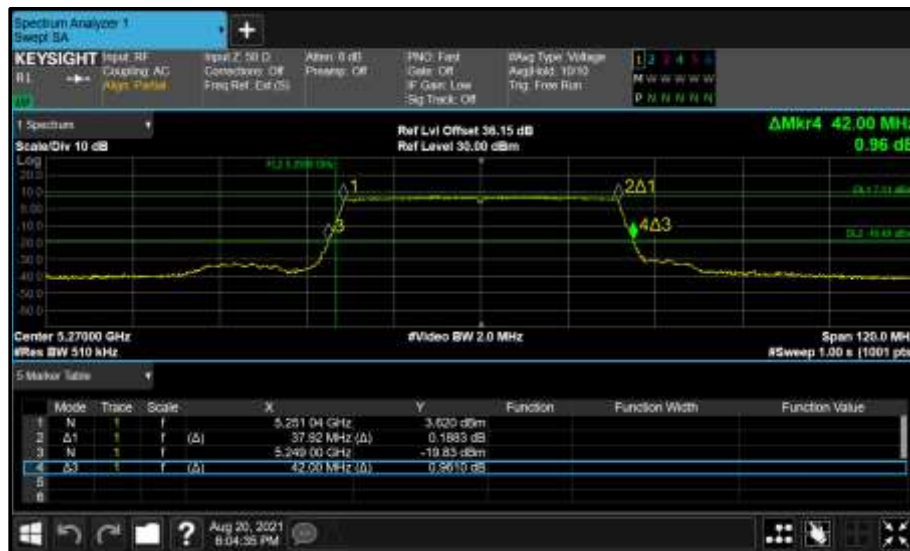
Figure 406 - Core 1 (B) 5270 MHz (CH54) 26 dB and 99% Bandwidth
