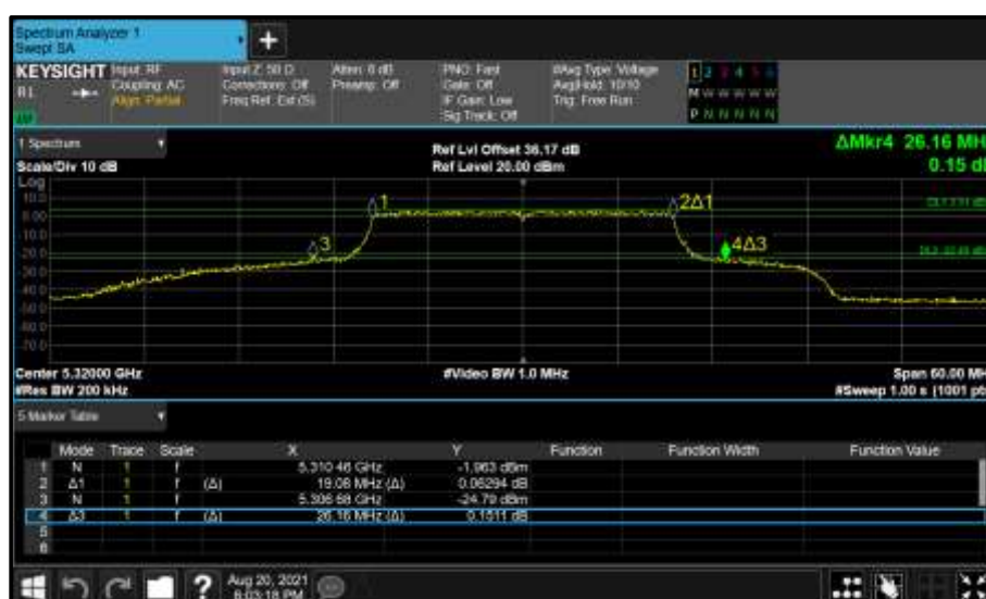
Figure 365 - Core 0 (A) 5320 MHz (CH64) 26 dB and 99% Bandwidth
