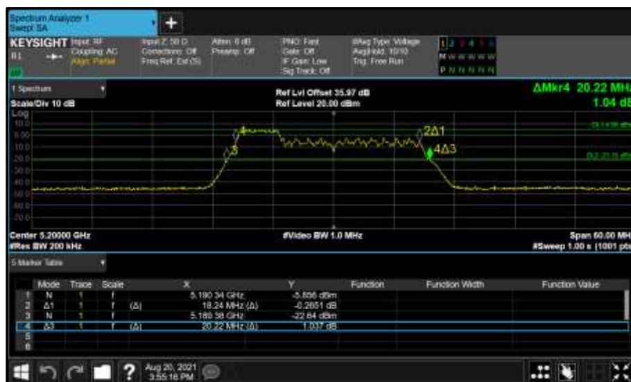
Figure 219 - Core 0 (A) 5200 MHz (CH40) 26 dB and 99% Bandwidth
