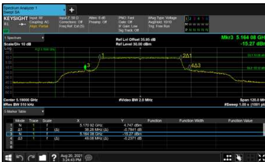
Figure 271 - Core 0 (A) 5190 MHz (CH38) 26 dB and 99% Bandwidth
