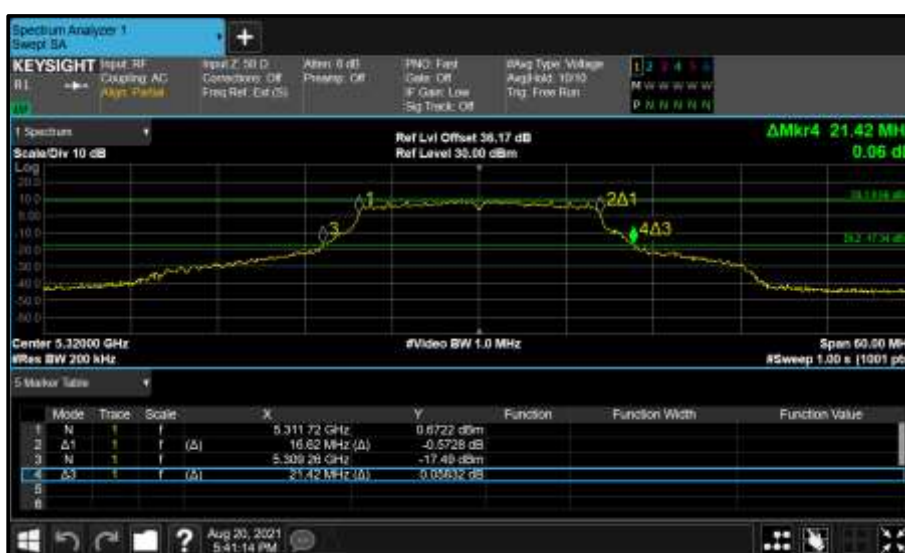
Figure 327 - Core 0 (A) 5320 MHz (CH64) 26 dB and 99% Bandwidth
