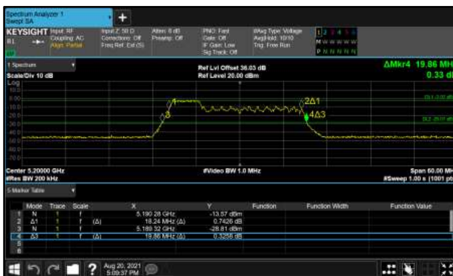
Figure 226 - Core 1 (B) 5200 MHz (CH40) 26 dB and 99% Bandwidth
