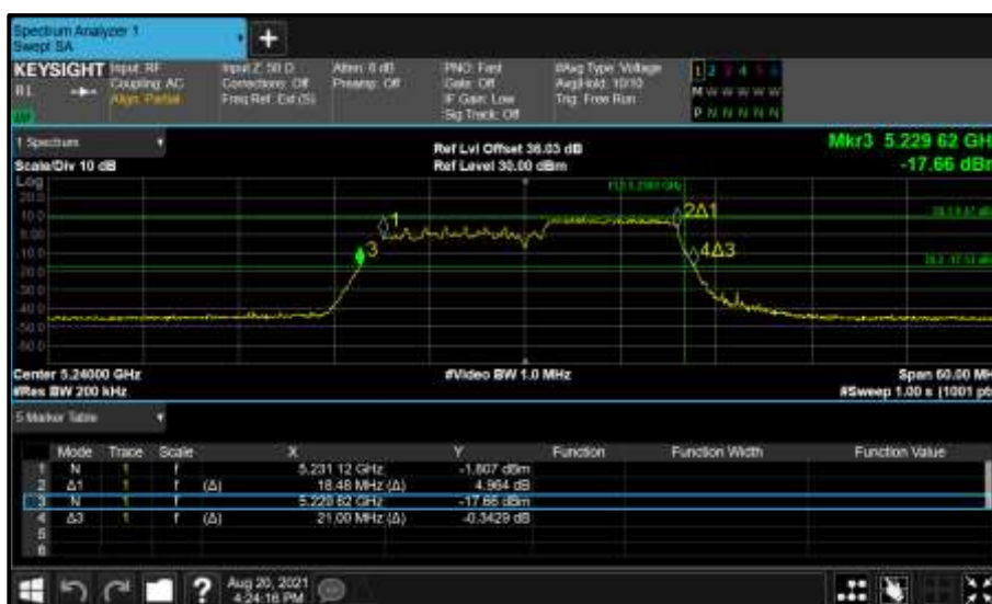
Figure 263 - Core 0 (A) 5240 MHz (CH48) 26 dB and 99% Bandwidth
