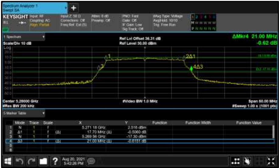
Figure 329 - Core 0 (A) 5280 MHz (CH56) 26 dB and 99% Bandwidth
