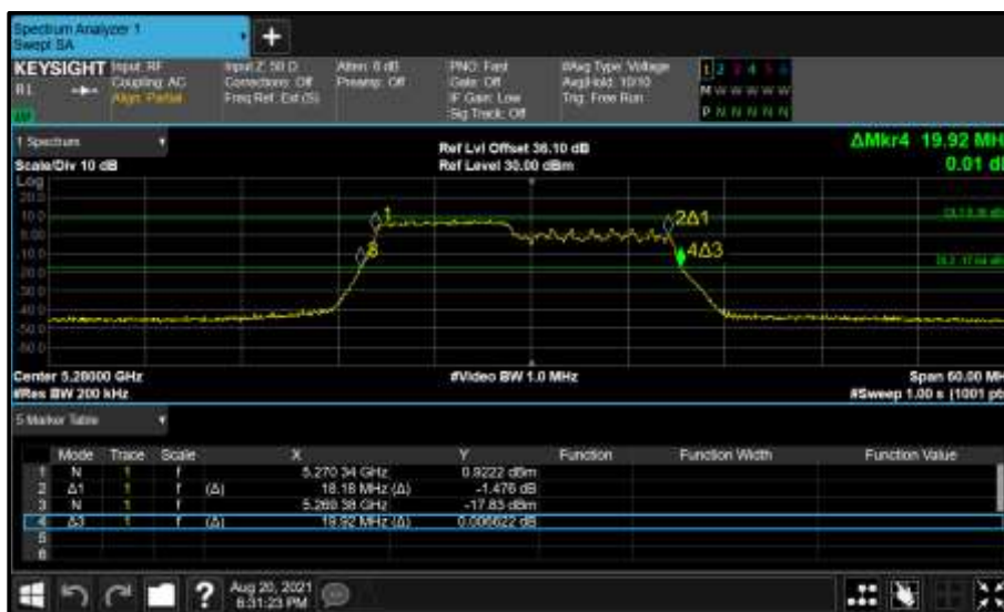
Figure 400 - Core 1 (B) 5280 MHz (CH56) 26 dB and 99% Bandwidth
