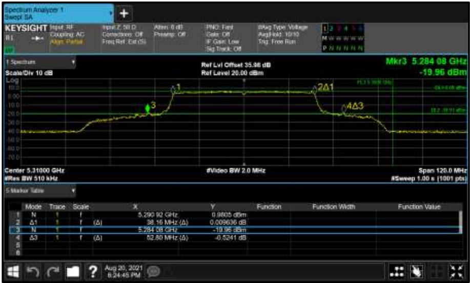
Figure 412 - Core 1 (B) 5310 MHz (CH62) 26 dB and 99% Bandwidth
