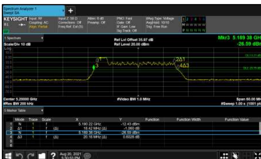
Figure 207 - Core 0 (A) 5200 MHz (CH40) 26 dB and 99% Bandwidth
