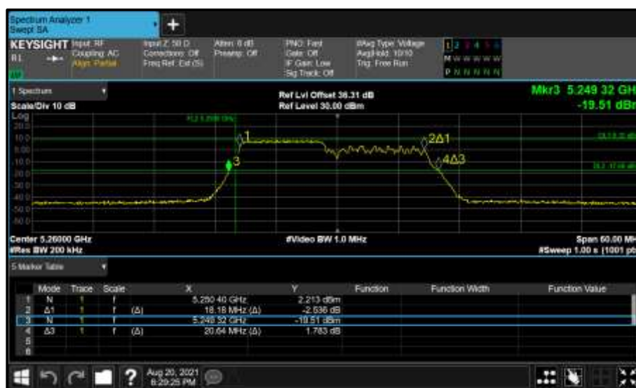
Figure 397 - Core 0 (A) 5260 MHz (CH52) 26 dB and 99% Bandwidth
