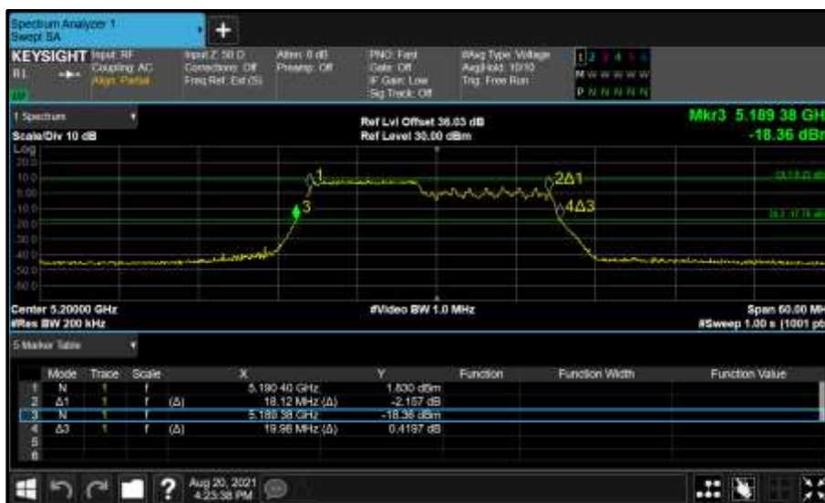
Figure 262 - Core 1 (B) 5200 MHz (CH40) 26 dB and 99% Bandwidth
