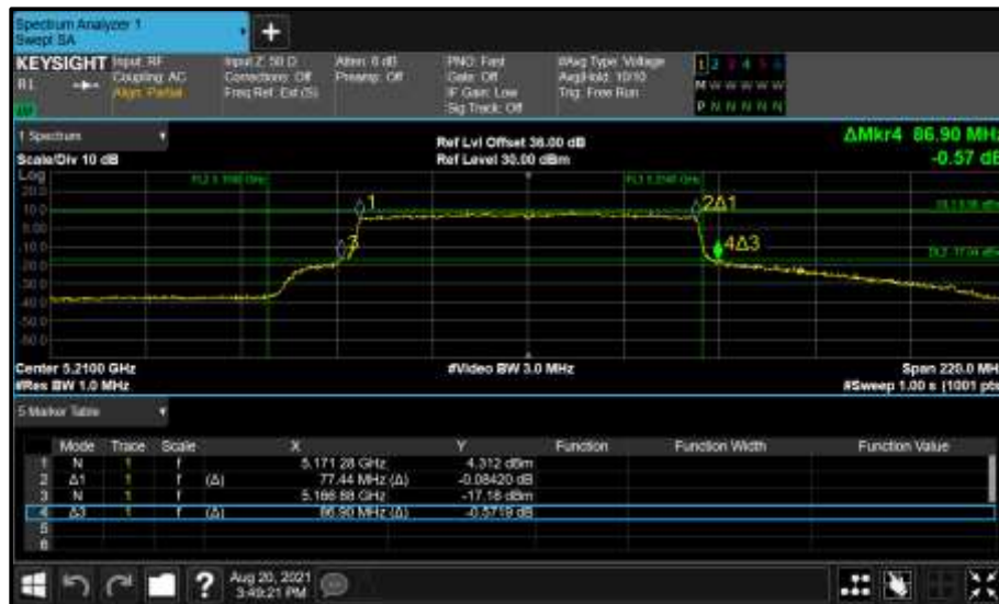
Figure 293 - Core 0 (A) 5210 MHz (CH42) 26 dB and 99% Bandwidth
