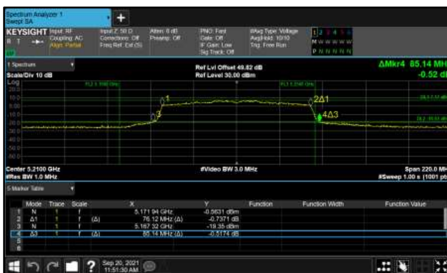
Figure 321 - Core 0 (A) 5210 MHz (CH42) 26 dB and 99% Bandwidth
