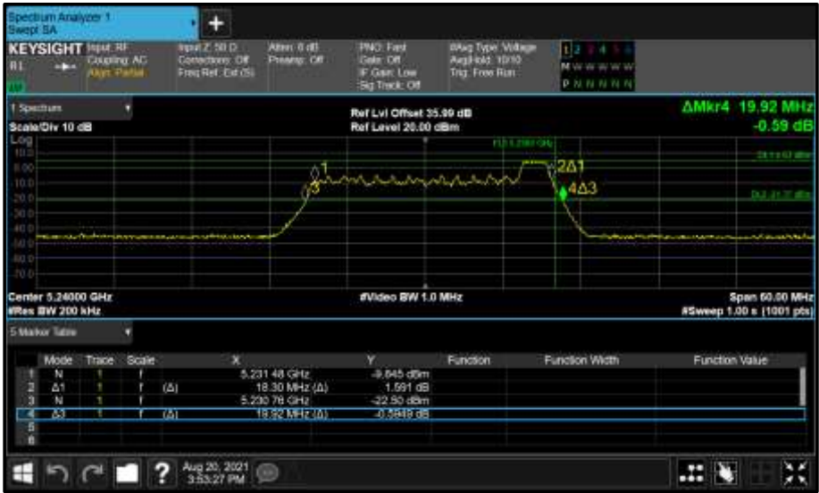
Figure 192 - Core 1 (B) 5240 MHz (CH48) 26 dB and 99% Bandwidth
