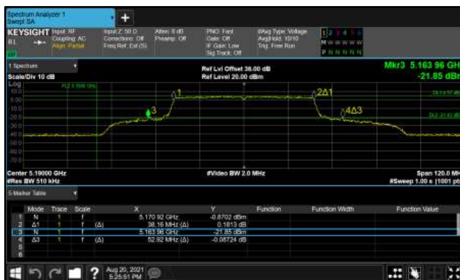
Figure 288 - Core 1 (B) 5190 MHz (CH38) 26 dB and 99% Bandwidth
