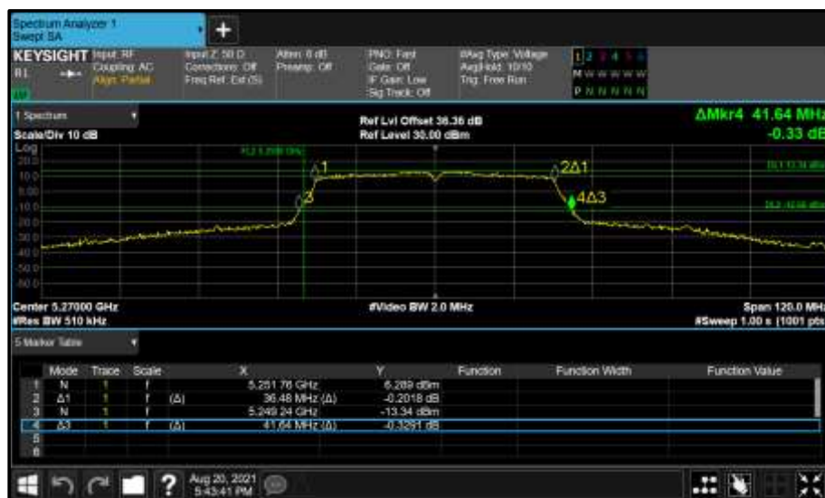
Figure 343 - Core 0 (A) 5270 MHz (CH54) 26 dB and 99% Bandwidth
