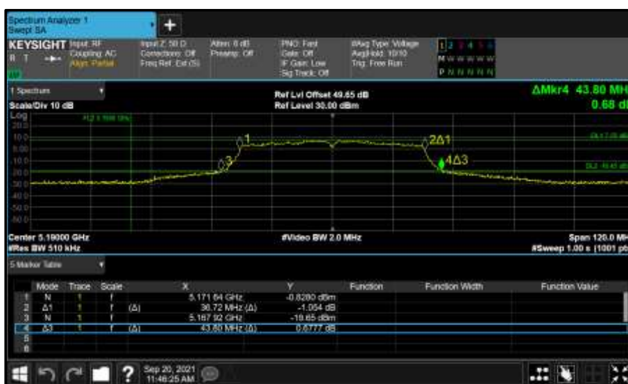
Figure 313 - Core 0 (A) 5190 MHz (CH38) 26 dB and 99% Bandwidth
