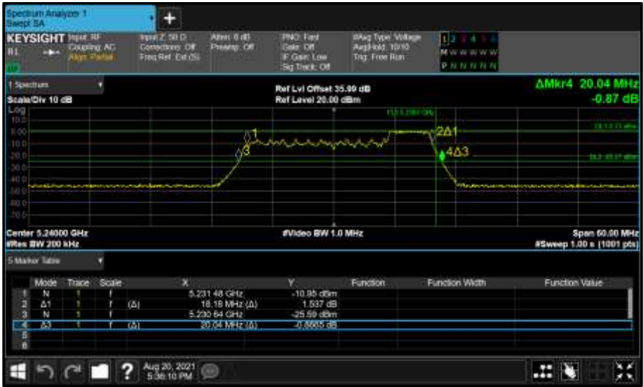
Figure 240 - Core 1 (B) 5240 MHz (CH48) 26 dB and 99% Bandwidth
