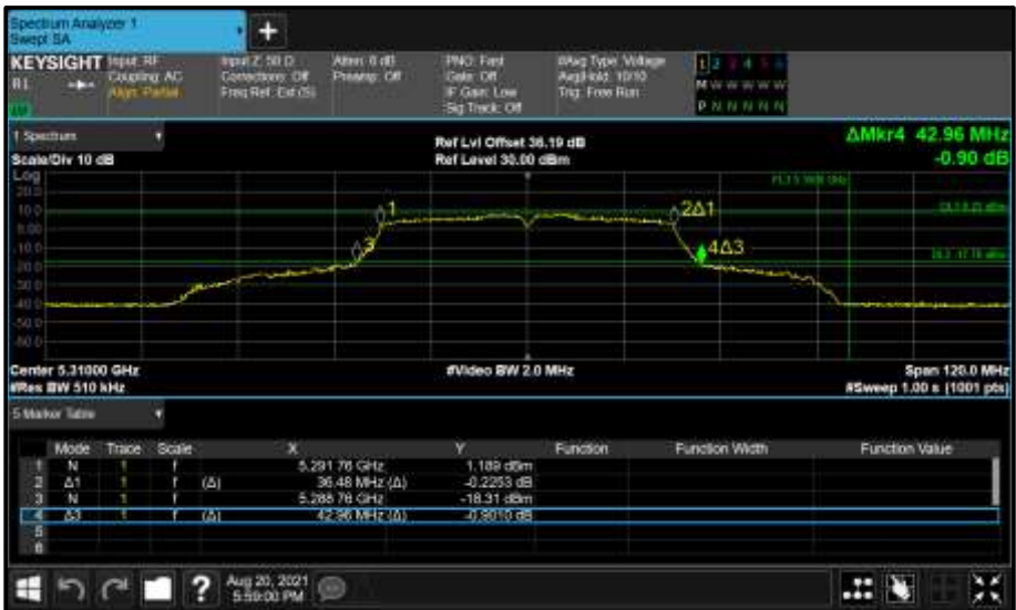
Figure 347 - Core 0 (A) 5310 MHz (CH62) 26 dB and 99% Bandwidth
