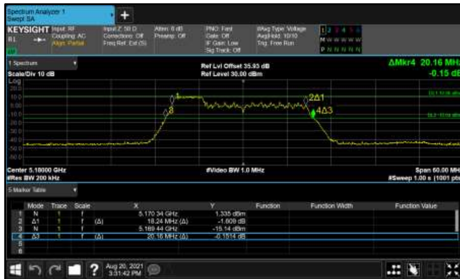
Figure 211 - Core 0 (A) 5180 MHz (CH36) 26 dB and 99% Bandwidth
