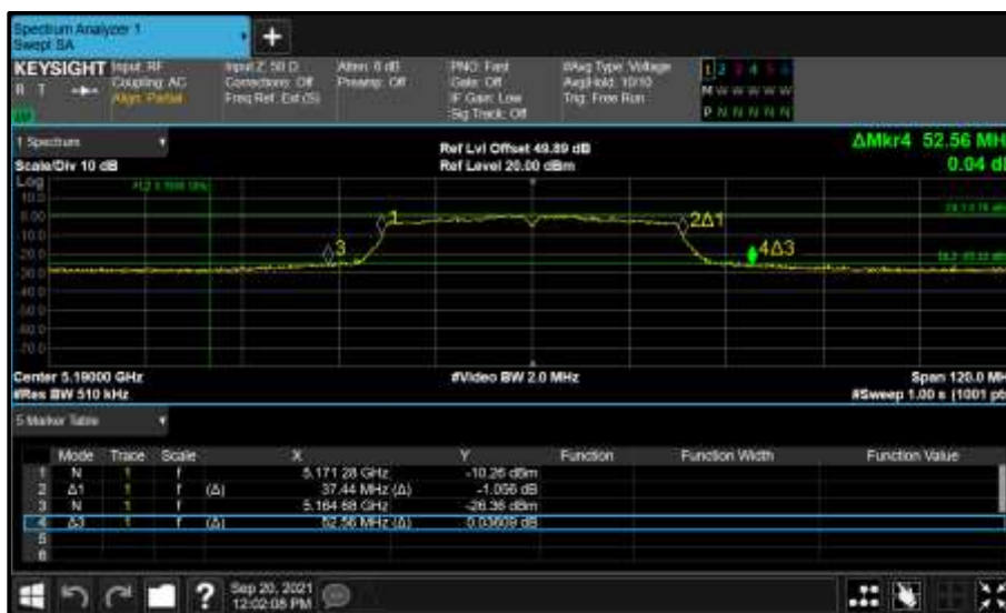
Figure 318 - Core 1 (B) 5190 MHz (CH38) 26 dB and 99% Bandwidth
