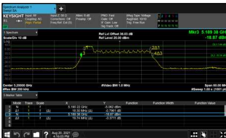
Figure 202 - Core 1 (B) 5200 MHz (CH40) 26 dB and 99% Bandwidth
