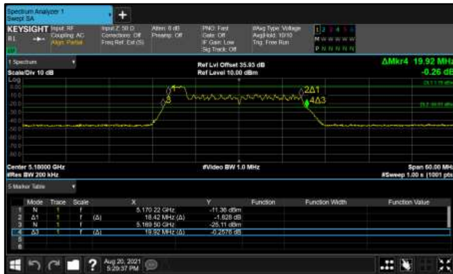
Figure 205 - Core 0 (A) 5180 MHz (CH36) 26 dB and 99% Bandwidth
