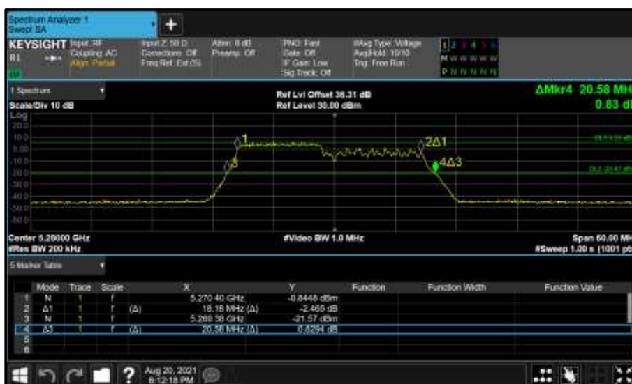
Figure 393 - Core 0 (A) 5280 MHz (CH56) 26 dB and 99% Bandwidth
