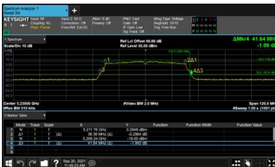
Figure 315 - Core 0 (A) 5230 MHz (CH46) 26 dB and 99% Bandwidth
