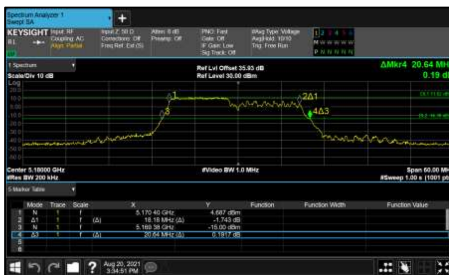
Figure 241 - Core 0 (A) 5180 MHz (CH36) 26 dB and 99% Bandwidth
