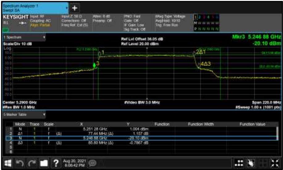
Figure 415 - Core 1 (B) 5290 MHz (CH58) 26 dB and 99% Bandwidth
