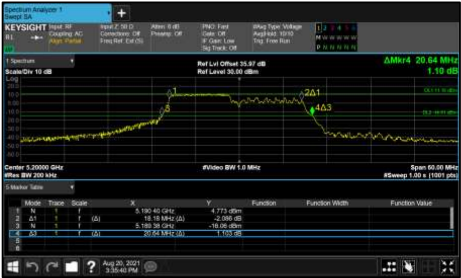
Figure 242 - Core 0 (A) 5200 MHz (CH40) 26 dB and 99% Bandwidth
