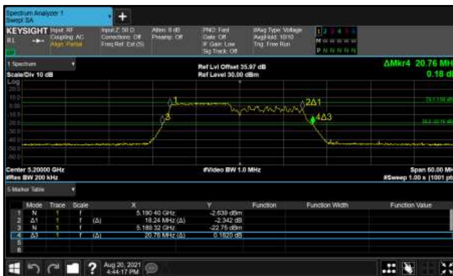
Figure 245 - Core 0 (A) 5200 MHz (CH40) 26 dB and 99% Bandwidth
