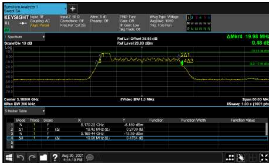
Figure 199 - Core 0 (A) 5180 MHz (CH36) 26 dB and 99% Bandwidth
