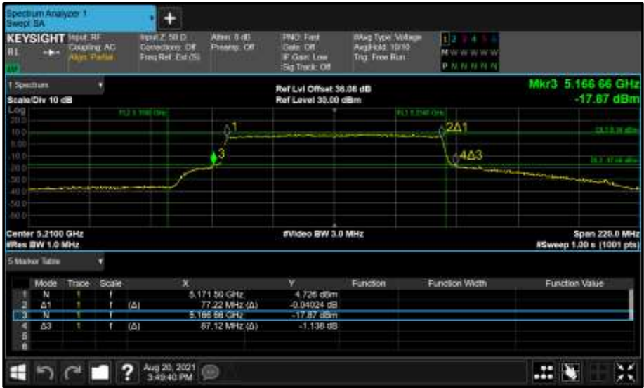
Figure 294 - Core 1 (B) 5210 MHz (CH42) 26 dB and 99% Bandwidth
