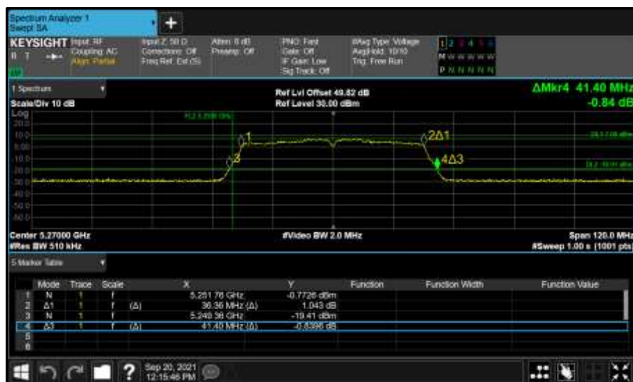
Figure 424 - Core 0 (A) 5270 MHz (CH54) 26 dB and 99% Bandwidth
