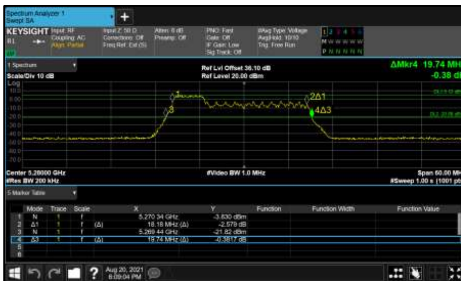
Figure 379 - Core 1 (B) 5280 MHz (CH56) 26 dB and 99% Bandwidth
