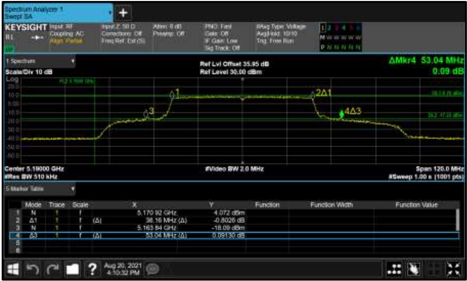
Figure 283 - Core 0 (A) 5190 MHz (CH38) 26 dB and 99% Bandwidth
