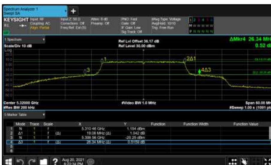
Figure 371 - Core 0 (A) 5320 MHz (CH64) 26 dB and 99% Bandwidth
