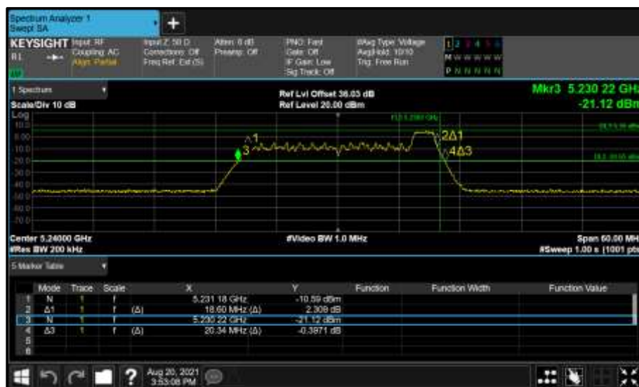
Figure 191 - Core 0 (A) 5240 MHz (CH48) 26 dB and 99% Bandwidth
