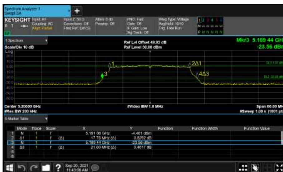
Figure 304 - Core 1 (B) 5200 MHz (CH40) 26 dB and 99% Bandwidth
