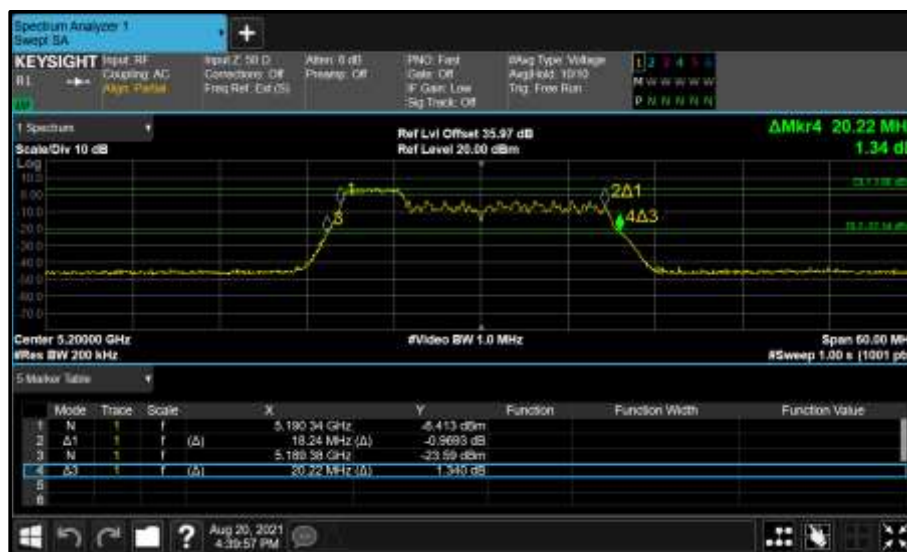
Figure 215 - Core 0 (A) 5200 MHz (CH40) 26 dB and 99% Bandwidth
