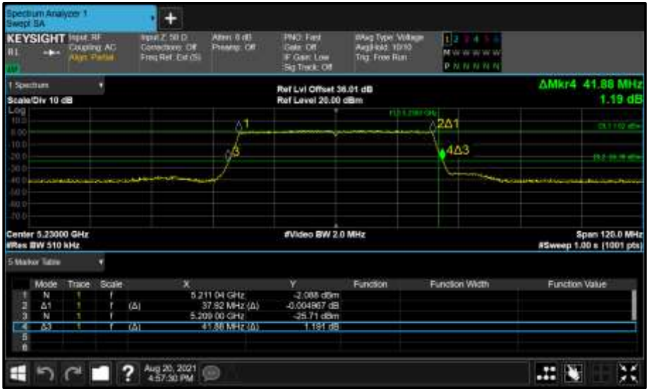
Figure 282 - Core 1 (B) 5230 MHz (CH46) 26 dB and 99% Bandwidth
