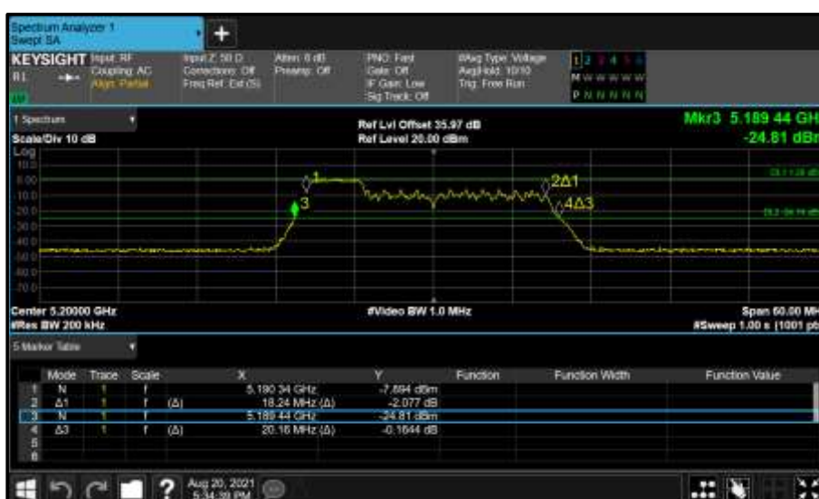
Figure 237 - Core 0 (A) 5200 MHz (CH40) 26 dB and 99% Bandwidth
