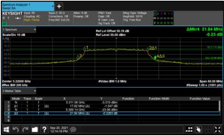
Figure 423 - Core 1 (B) 5320 MHz (CH64) 26 dB and 99% Bandwidth
