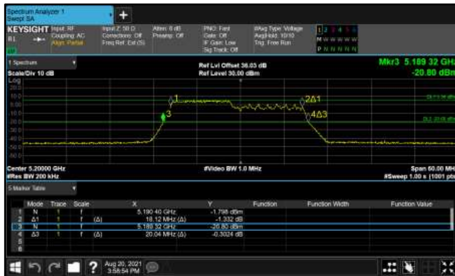
Figure 250 - Core 1 (B) 5200 MHz (CH40) 26 dB and 99% Bandwidth
