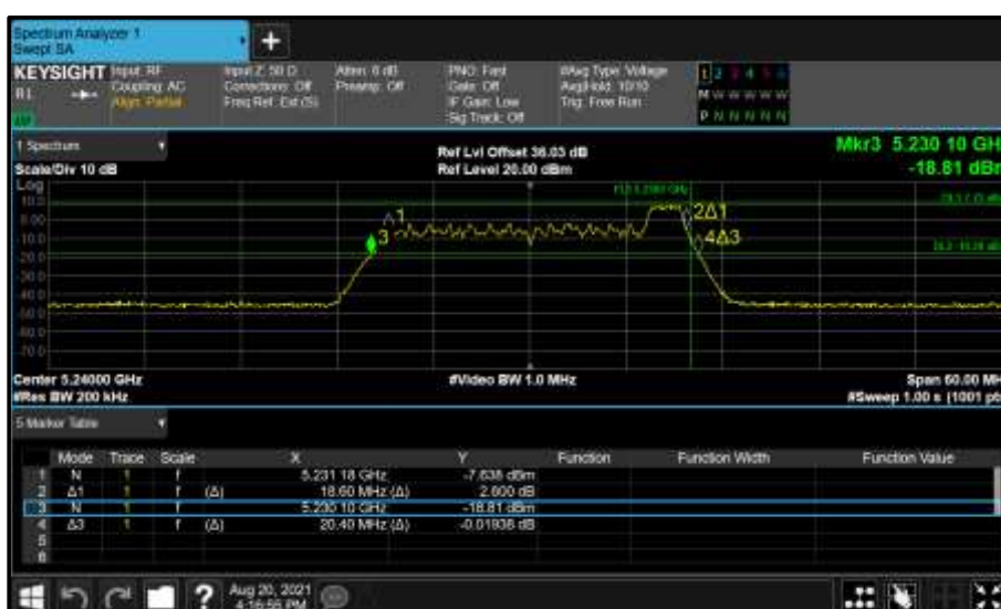
Figure 203 - Core 0 (A) 5240 MHz (CH48) 26 dB and 99% Bandwidth
