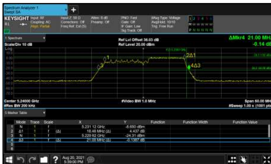
Figure 269 - Core 0 (A) 5240 MHz (CH48) 26 dB and 99% Bandwidth
