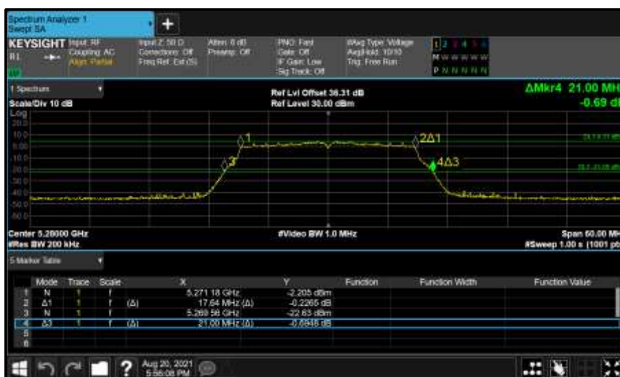
Figure 333 - Core 0 (A) 5280 MHz (CH56) 26 dB and 99% Bandwidth
