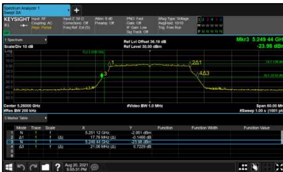
Figure 332 - Core 1 (B) 5260 MHz (CH52) 26 dB and 99% Bandwidth
