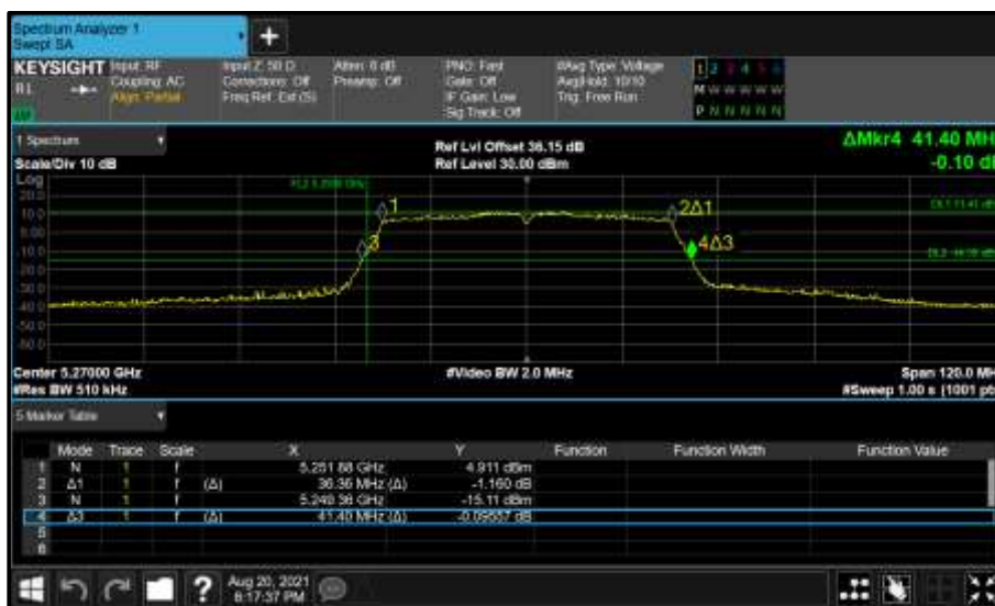
Figure 350 - Core 1 (B) 5270 MHz (CH54) 26 dB and 99% Bandwidth
