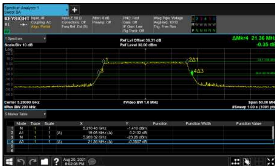
Figure 363 - Core 0 (A) 5280 MHz (CH56) 26 dB and 99% Bandwidth
