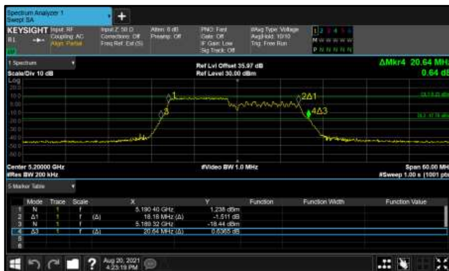
Figure 261 - Core 0 (A) 5200 MHz (CH40) 26 dB and 99% Bandwidth
