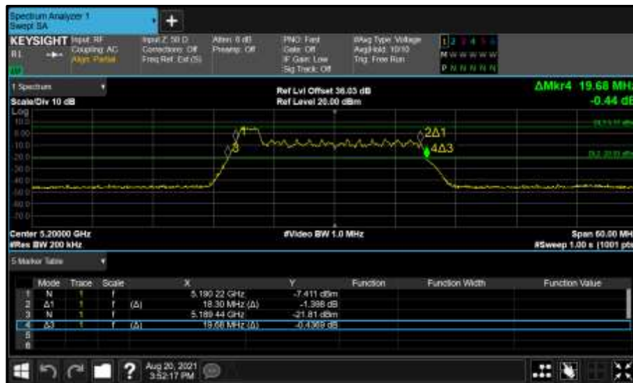
Figure 190 - Core 1 (B) 5200 MHz (CH40) 26 dB and 99% Bandwidth
