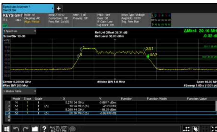
Figure 384 - Core 0 (A) 5280 MHz (CH56) 26 dB and 99% Bandwidth
