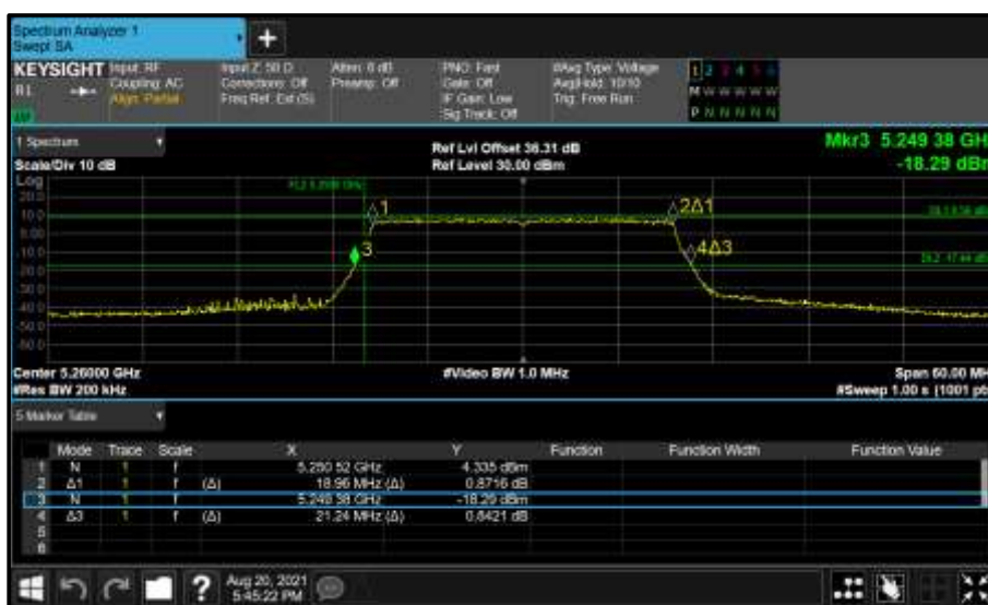
Figure 358 - Core 0 (A) 5260 MHz (CH52) 26 dB and 99% Bandwidth
