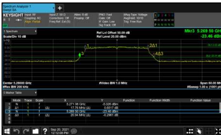
Figure 421 - Core 1 (B) 5280 MHz (CH56) 26 dB and 99% Bandwidth
