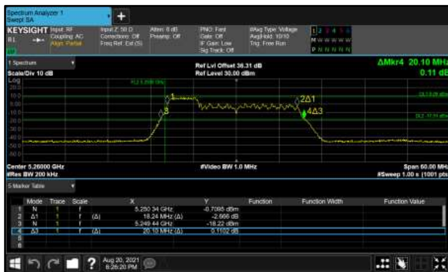
Figure 382 - Core 0 (A) 5260 MHz (CH52) 26 dB and 99% Bandwidth
