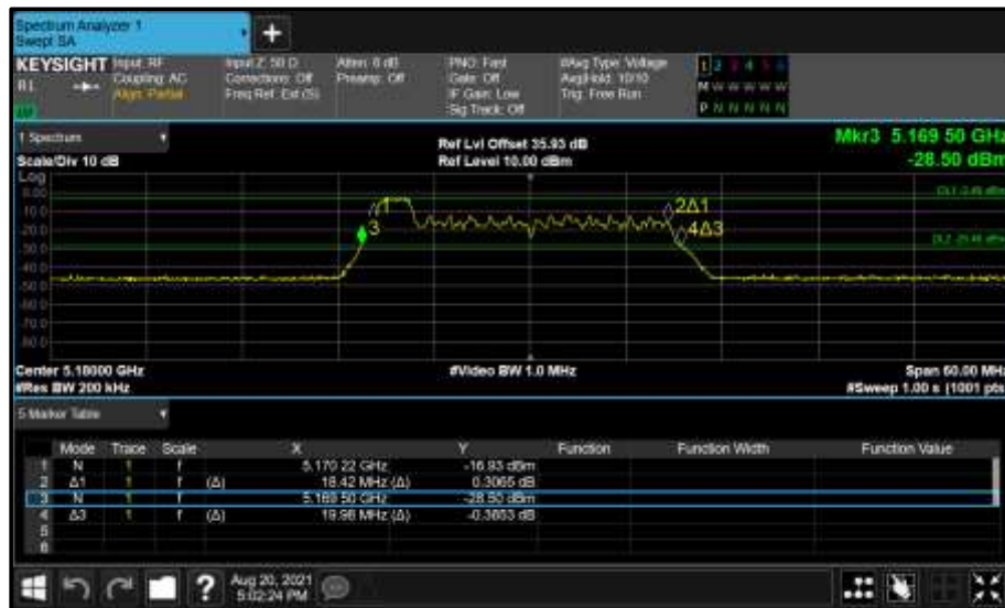
Figure 193 - Core 0 (A) 5180 MHz (CH36) 26 dB and 99% Bandwidth
