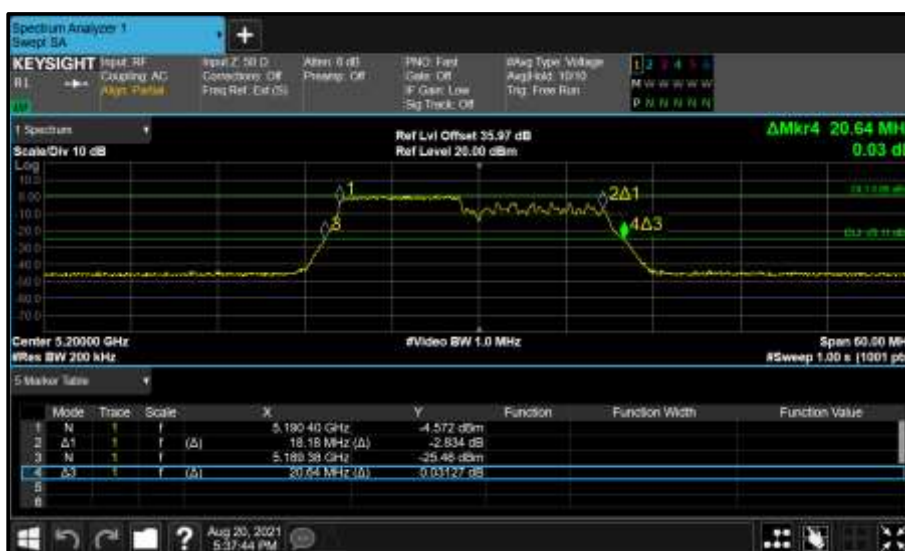
Figure 267 - Core 0 (A) 5200 MHz (CH40) 26 dB and 99% Bandwidth
