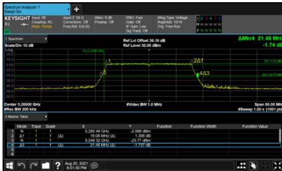
Figure 362 - Core 1 (B) 5260 MHz (CH52) 26 dB and 99% Bandwidth
