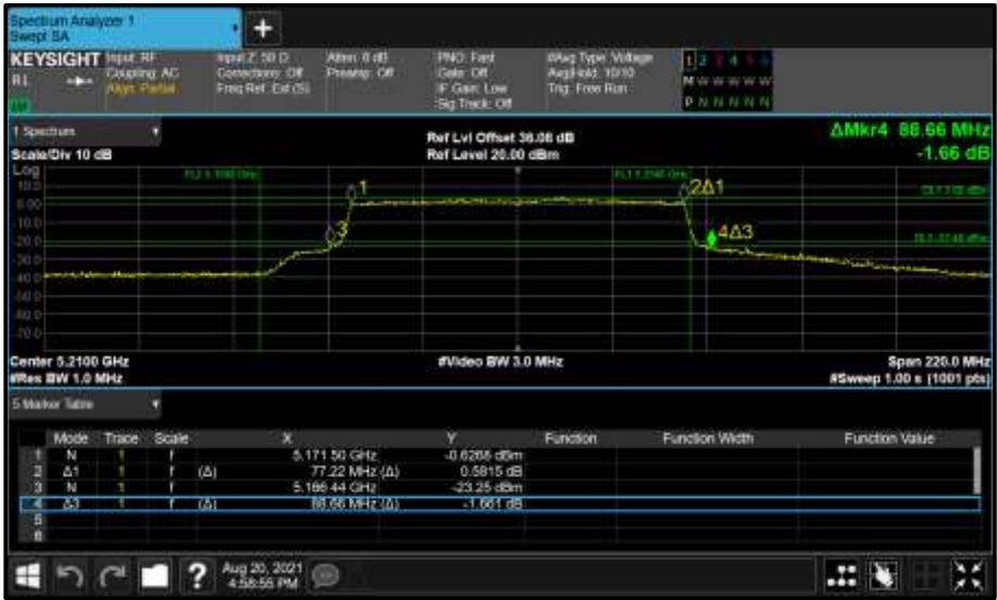
Figure 296 - Core 1 (B) 5210 MHz (CH42) 26 dB and 99% Bandwidth
