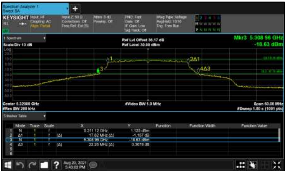
Figure 330 - Core 0 (A) 5320 MHz (CH64) 26 dB and 99% Bandwidth
