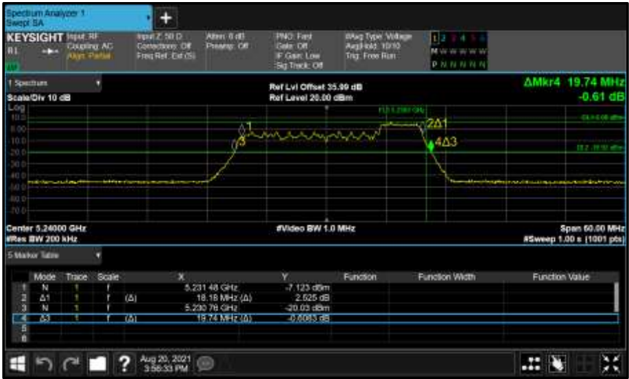
Figure 222 - Core 1 (B) 5240 MHz (CH48) 26 dB and 99% Bandwidth
