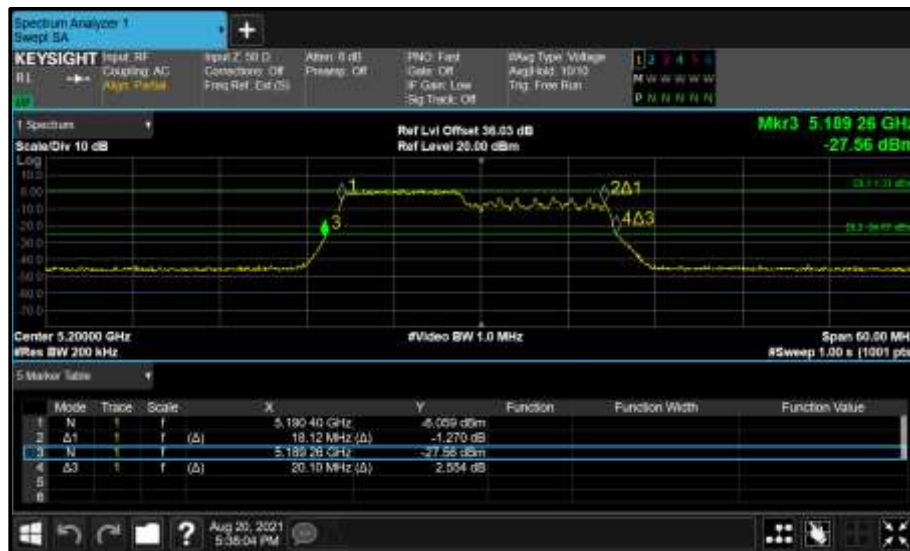
Figure 268 - Core 1 (B) 5200 MHz (CH40) 26 dB and 99% Bandwidth
