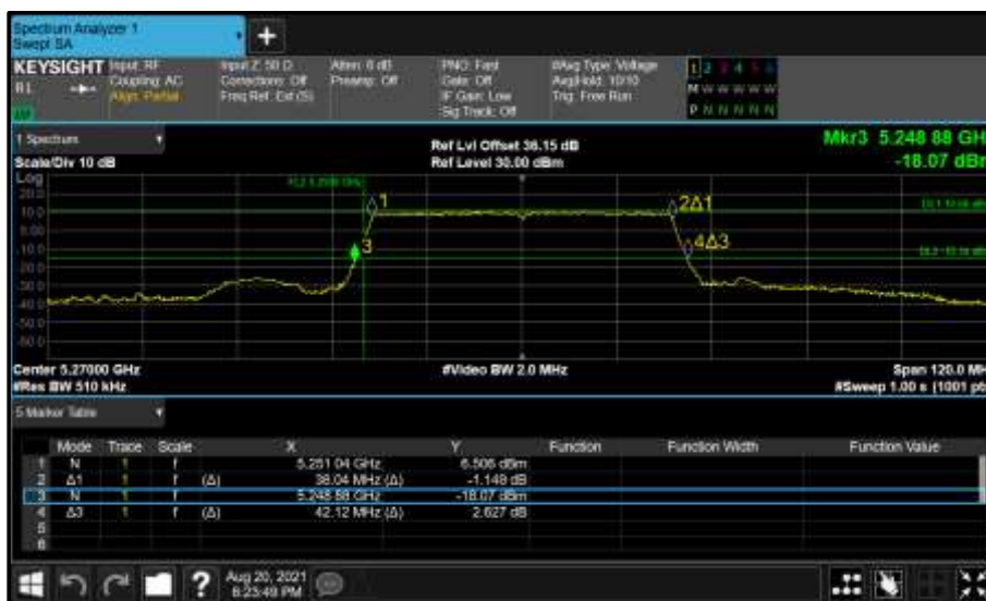
Figure 410 - Core 1 (B) 5270 MHz (CH54) 26 dB and 99% Bandwidth
