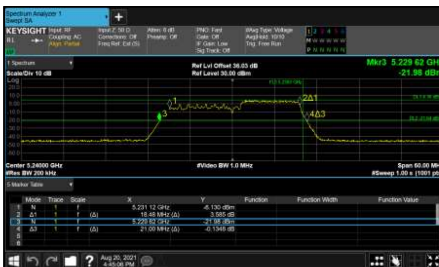
Figure 246 - Core 0 (A) 5240 MHz (CH48) 26 dB and 99% Bandwidth
