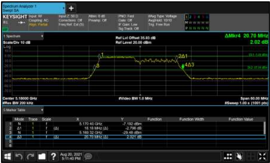
Figure 253 - Core 0 (A) 5180 MHz (CH36) 26 dB and 99% Bandwidth
