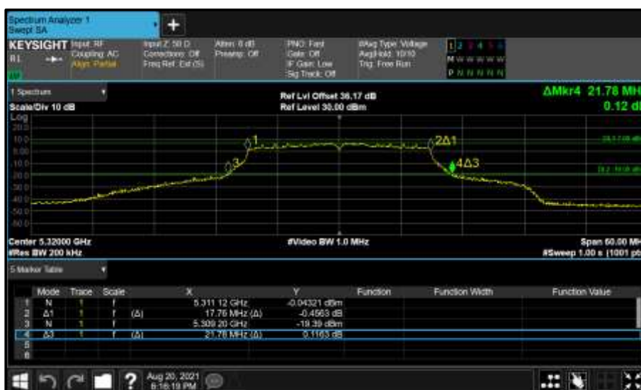
Figure 341 - Core 0 (A) 5320 MHz (CH64) 26 dB and 99% Bandwidth
