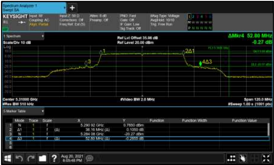
Figure 408 - Core 1 (B) 5310 MHz (CH62) 26 dB and 99% Bandwidth
