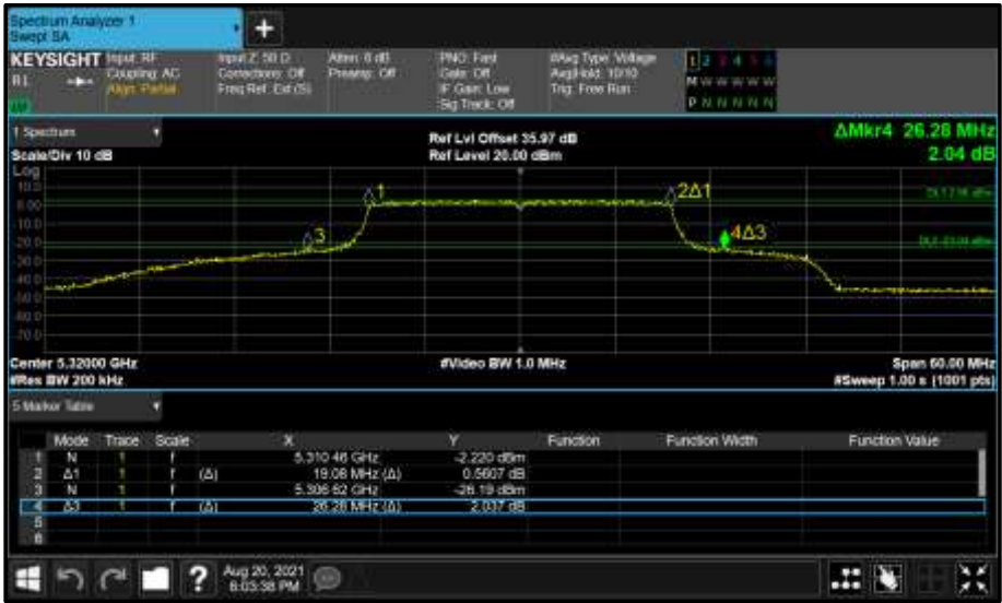
Figure 366 - Core 1 (B) 5320 MHz (CH64) 26 dB and 99% Bandwidth
