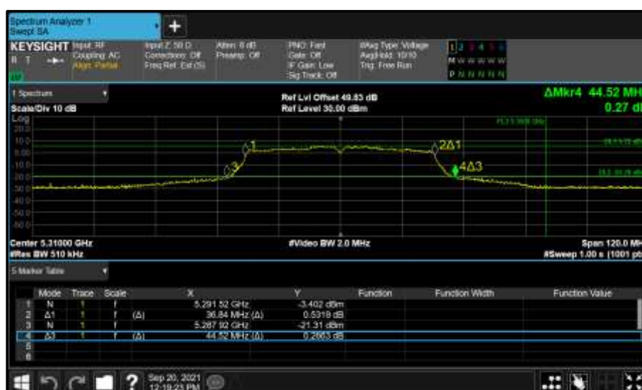
Figure 426 - Core 0 (A) 5310 MHz (CH62) 26 dB and 99% Bandwidth
