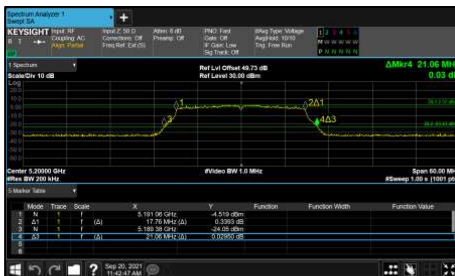
Figure 303 - Core 0 (A) 5200 MHz (CH40) 26 dB and 99% Bandwidth
