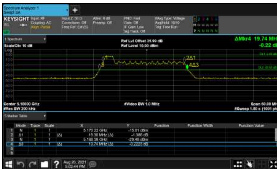
Figure 194 - Core 1 (B) 5180 MHz (CH36) 26 dB and 99% Bandwidth
