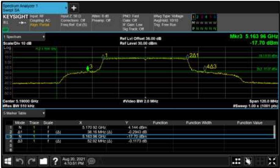
Figure 284 - Core 1 (B) 5190 MHz (CH38) 26 dB and 99% Bandwidth
