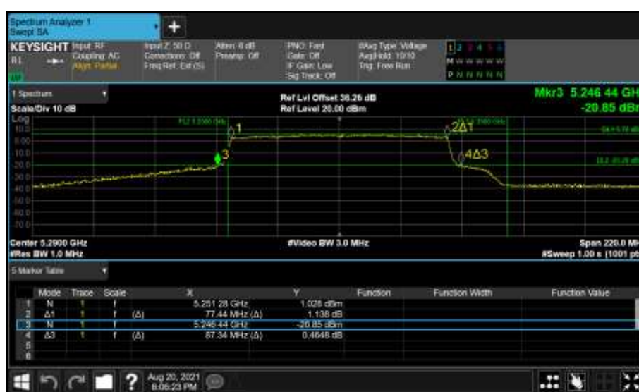
Figure 414 - Core 0 (A) 5290 MHz (CH58) 26 dB and 99% Bandwidth
