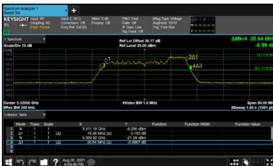
Figure 380 - Core 0 (A) 5320 MHz (CH64) 26 dB and 99% Bandwidth
