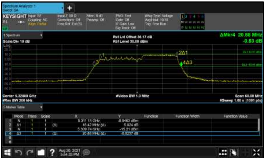
Figure 390 - Core 0 (A) 5320 MHz (CH64) 26 dB and 99% Bandwidth
