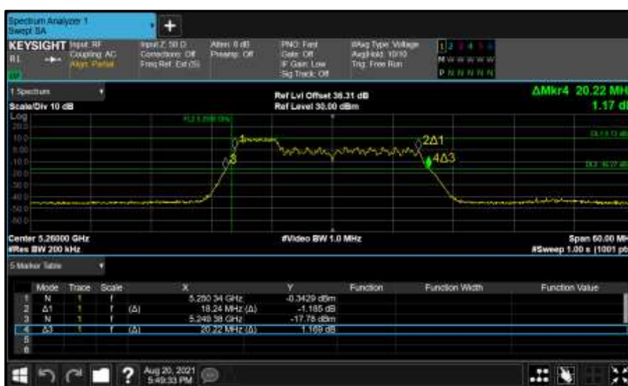
Figure 373 - Core 0 (A) 5260 MHz (CH52) 26 dB and 99% Bandwidth
