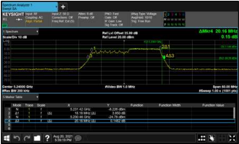
Figure 270 - Core 1 (B) 5240 MHz (CH48) 26 dB and 99% Bandwidth
