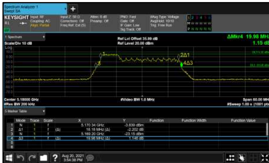
Figure 218 - Core 1 (B) 5180 MHz (CH36) 26 dB and 99% Bandwidth
