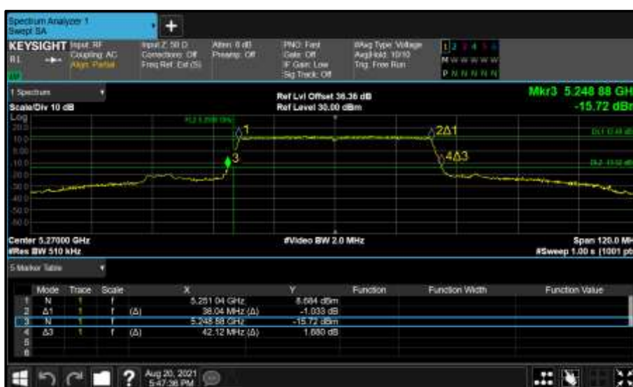
Figure 403 - Core 0 (A) 5270 MHz (CH54) 26 dB and 99% Bandwidth
