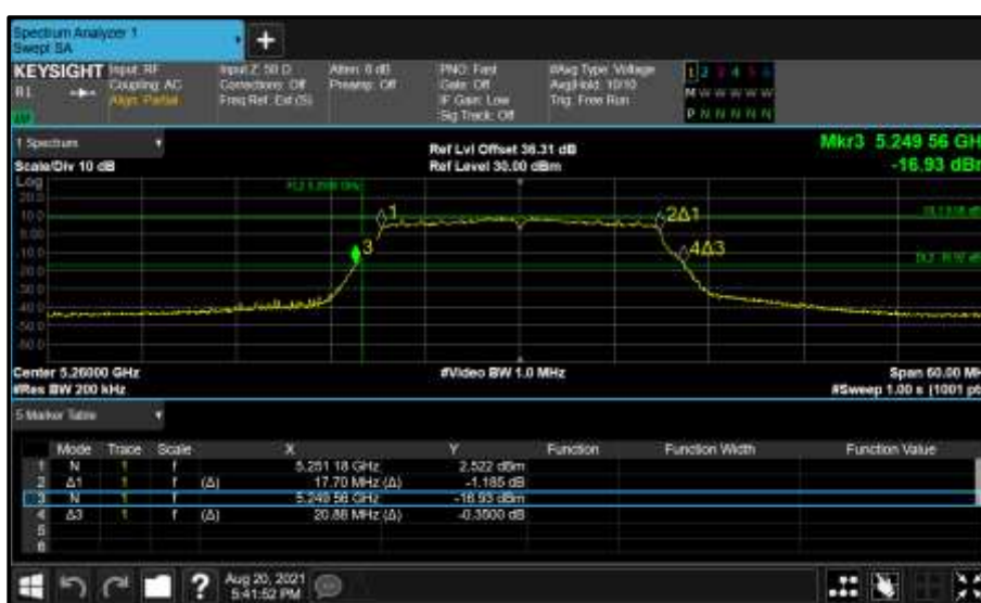
Figure 328 - Core 0 (A) 5260 MHz (CH52) 26 dB and 99% Bandwidth
