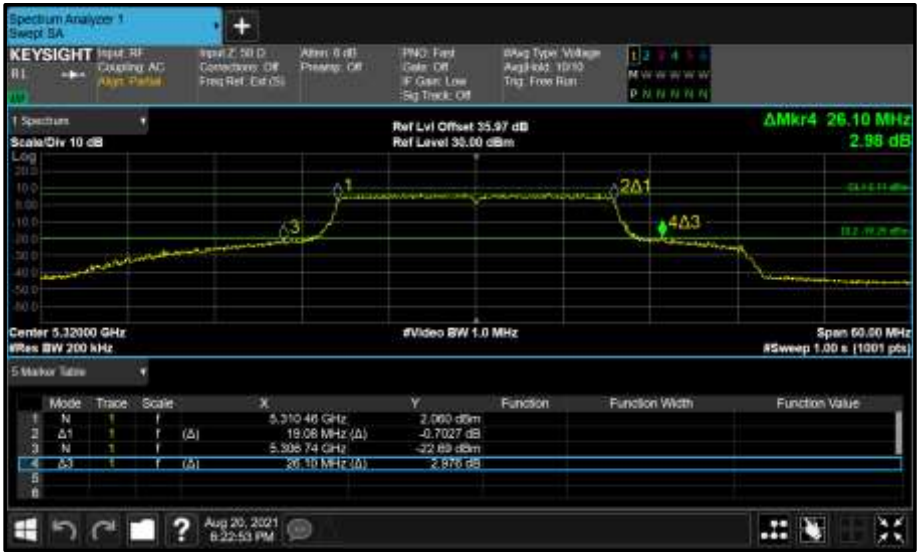
Figure 372 - Core 1 (B) 5320 MHz (CH64) 26 dB and 99% Bandwidth
