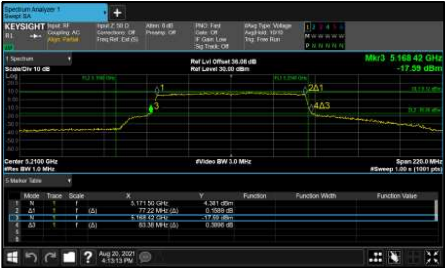
Figure 298 - Core 1 (B) 5210 MHz (CH42) 26 dB and 99% Bandwidth
