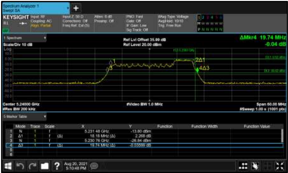
Figure 228 - Core 1 (B) 5240 MHz (CH48) 26 dB and 99% Bandwidth
