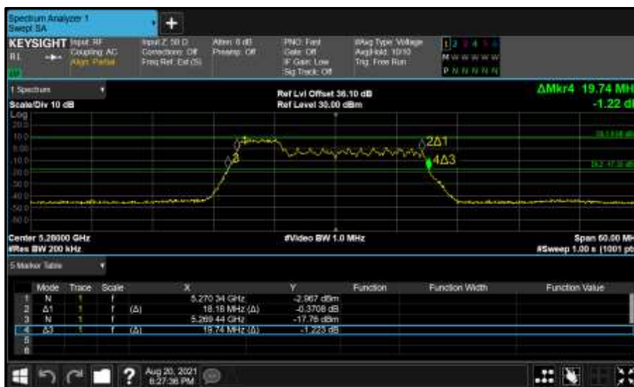
Figure 385 - Core 1 (B) 5280 MHz (CH56) 26 dB and 99% Bandwidth
