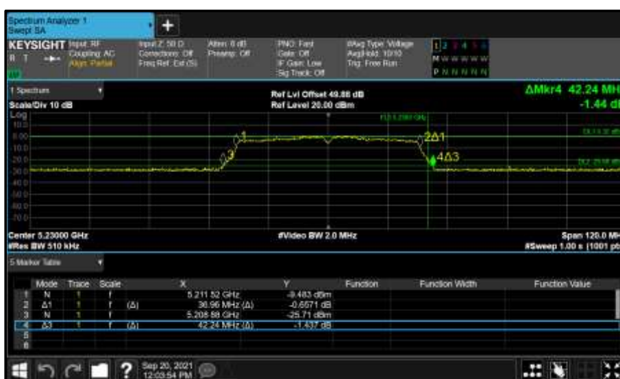
Figure 319 - Core 0 (A) 5230 MHz (CH46) 26 dB and 99% Bandwidth
