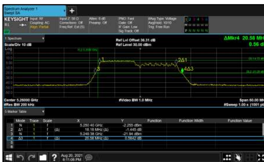
Figure 391 - Core 0 (A) 5260 MHz (CH52) 26 dB and 99% Bandwidth
