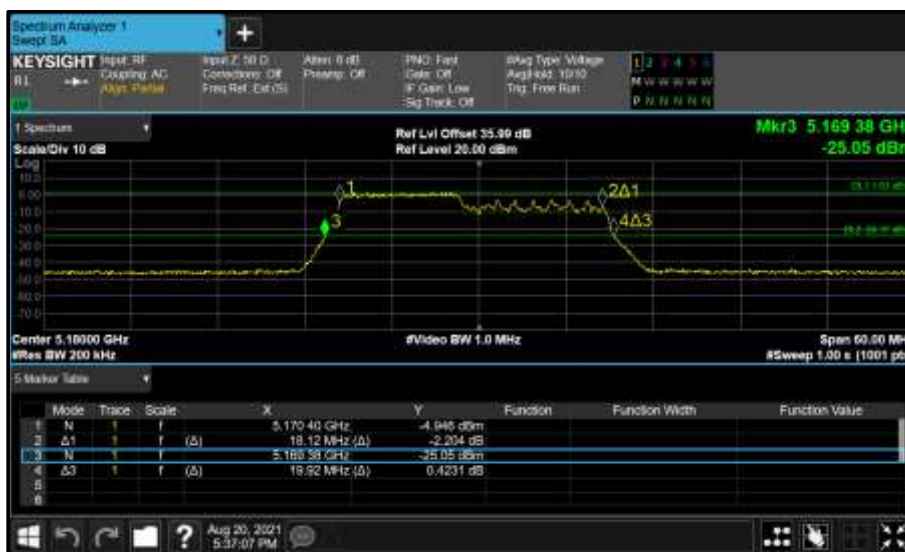
Figure 266 - Core 1 (B) 5180 MHz (CH36) 26 dB and 99% Bandwidth
