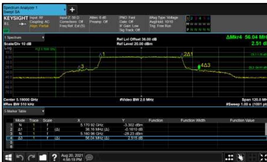
Figure 280 - Core 1 (B) 5190 MHz (CH38) 26 dB and 99% Bandwidth
