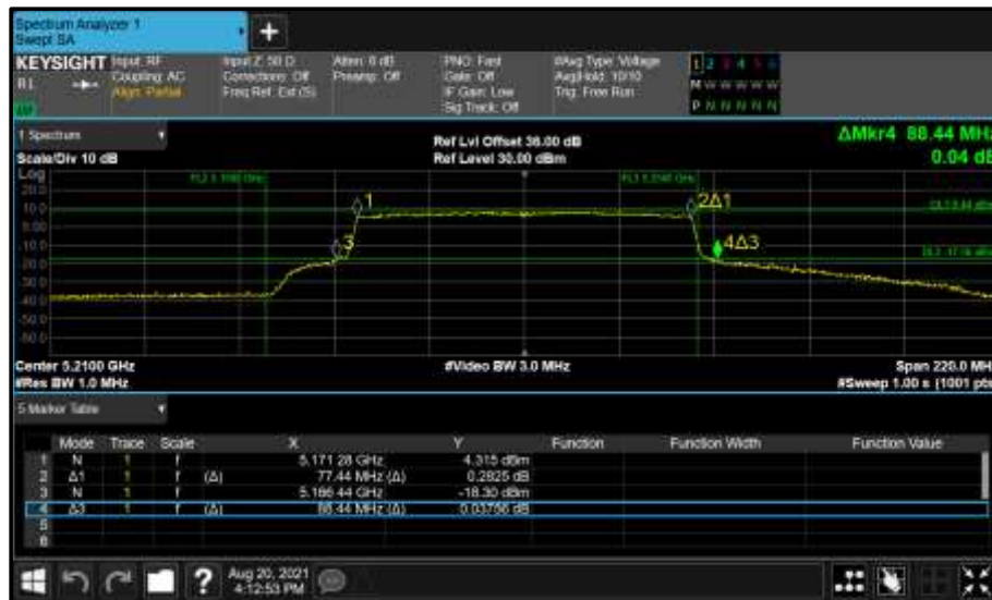
Figure 297 - Core 0 (A) 5210 MHz (CH42) 26 dB and 99% Bandwidth
