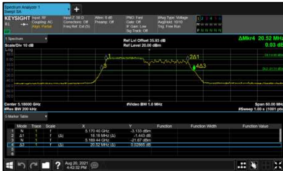
Figure 244 - Core 0 (A) 5180 MHz (CH36) 26 dB and 99% Bandwidth
