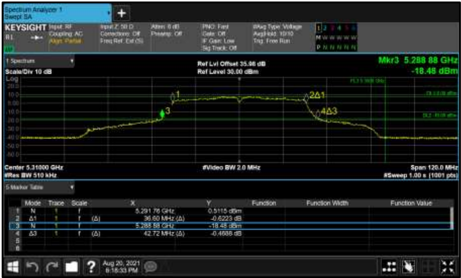
Figure 352 - Core 1 (B) 5310 MHz (CH62) 26 dB and 99% Bandwidth
