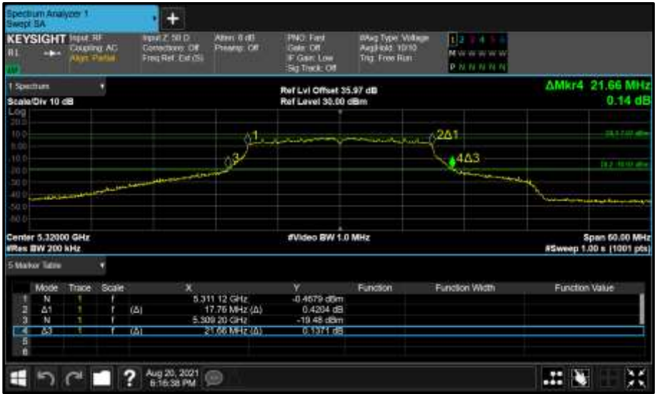
Figure 342 - Core 1 (B) 5320 MHz (CH64) 26 dB and 99% Bandwidth
