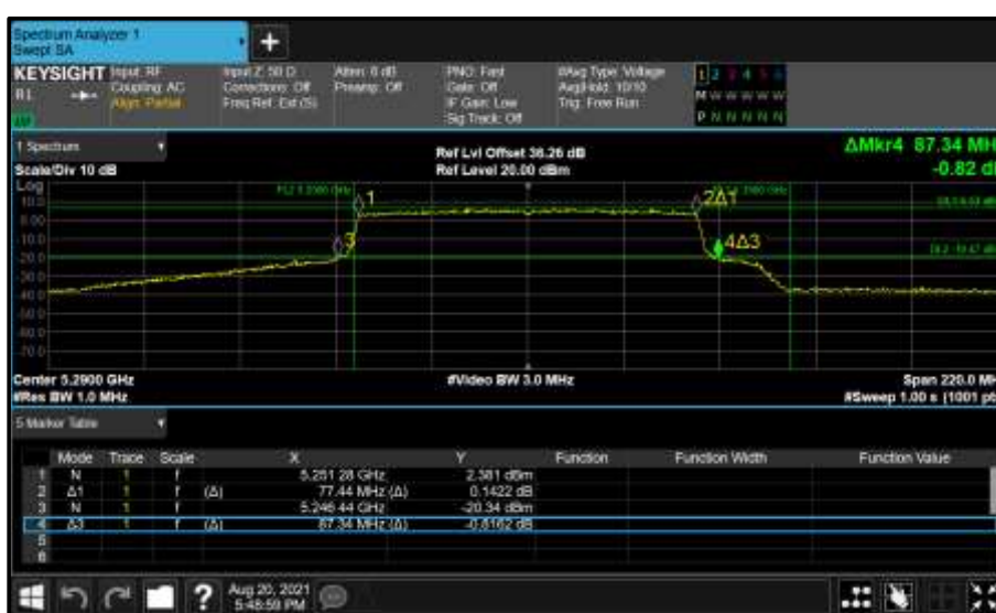
Figure 413 - Core 0 (A) 5290 MHz (CH58) 26 dB and 99% Bandwidth
