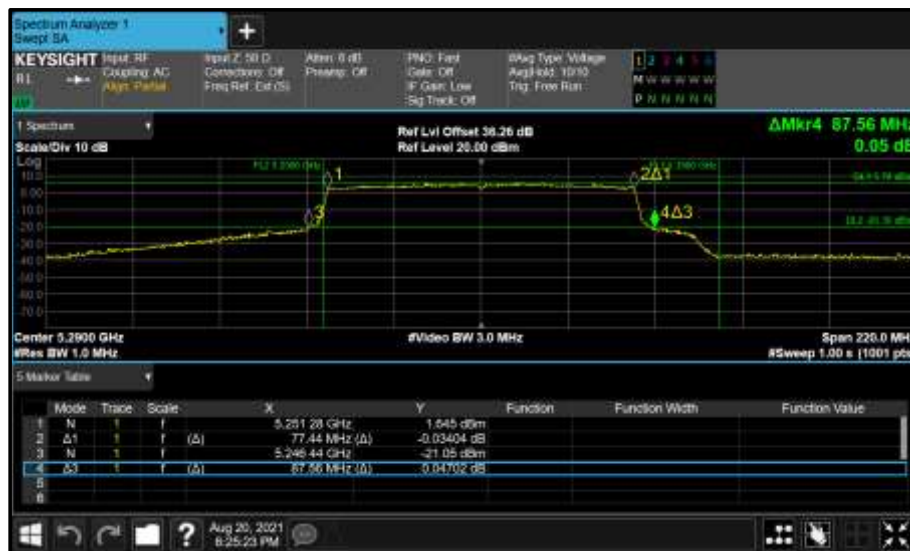
Figure 416 - Core 0 (A) 5290 MHz (CH58) 26 dB and 99% Bandwidth
