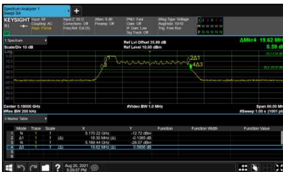
Figure 206 - Core 1 (B) 5180 MHz (CH36) 26 dB and 99% Bandwidth
