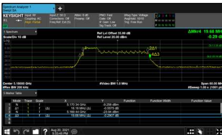
Figure 236 - Core 1 (B) 5180 MHz (CH36) 26 dB and 99% Bandwidth
