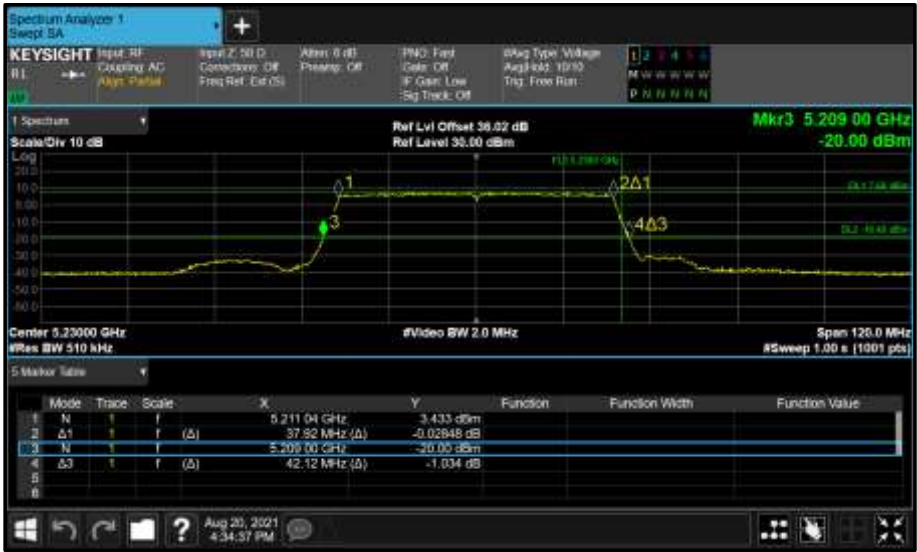
Figure 274 - Core 0 (A) 5230 MHz (CH46) 26 dB and 99% Bandwidth
