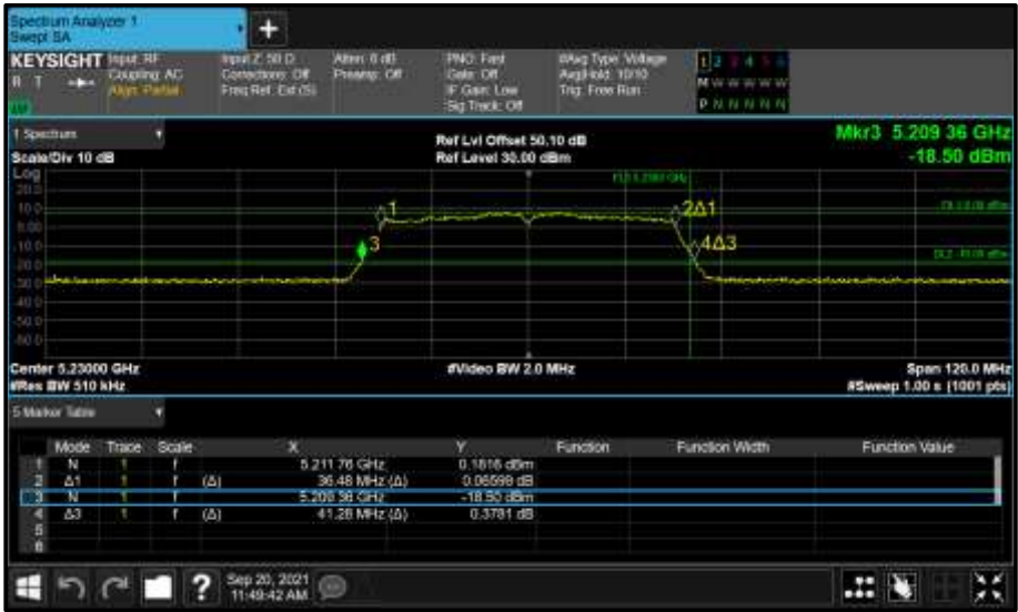
Figure 316 - Core 1 (B) 5230 MHz (CH46) 26 dB and 99% Bandwidth
