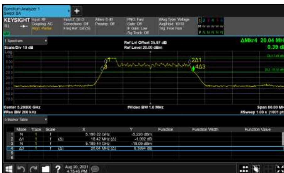
Figure 201 - Core 0 (A) 5200 MHz (CH40) 26 dB and 99% Bandwidth
