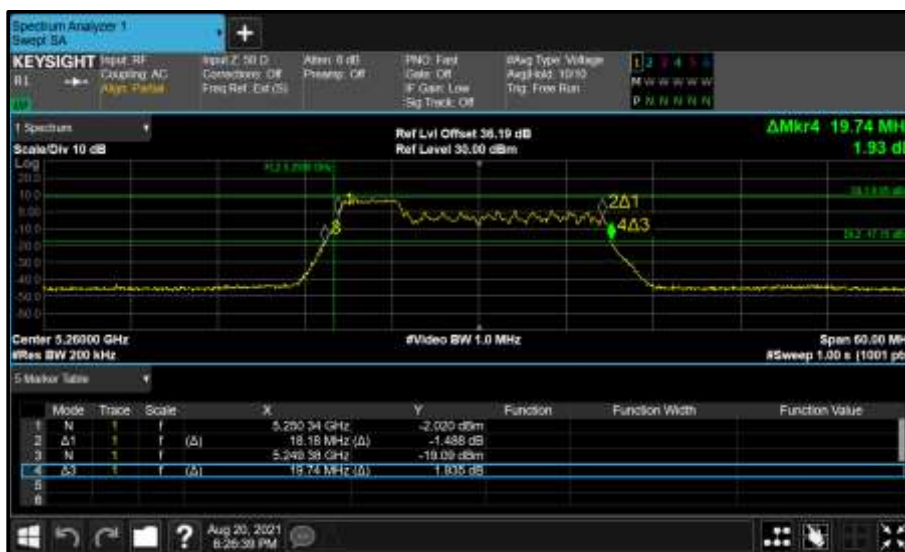
Figure 383 - Core 1 (B) 5260 MHz (CH52) 26 dB and 99% Bandwidth
