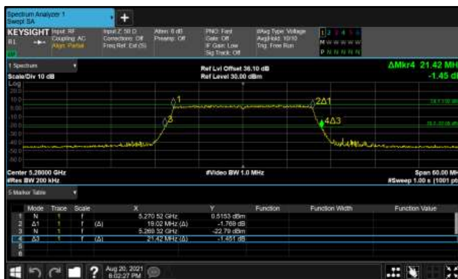
Figure 364 - Core 1 (B) 5280 MHz (CH56) 26 dB and 99% Bandwidth
