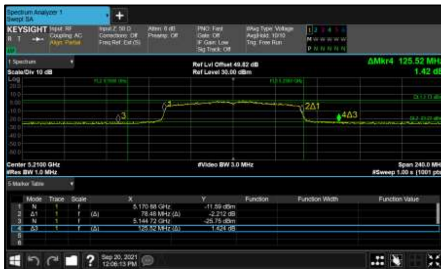
Figure 323 - Core 0 (A) 5210 MHz (CH42) 26 dB and 99% Bandwidth
