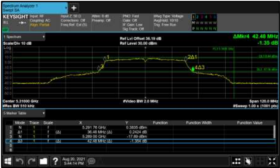
Figure 344 - Core 0 (A) 5310 MHz (CH62) 26 dB and 99% Bandwidth
