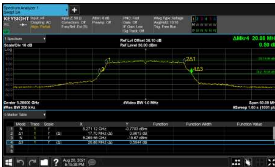
Figure 340 - Core 1 (B) 5280 MHz (CH56) 26 dB and 99% Bandwidth
