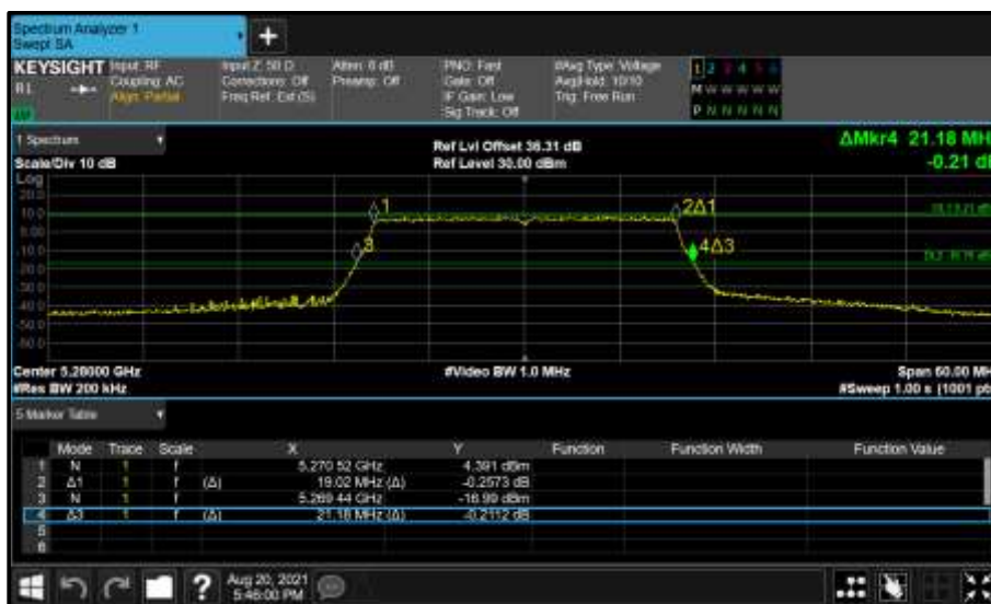
Figure 359 - Core 0 (A) 5280 MHz (CH56) 26 dB and 99% Bandwidth
