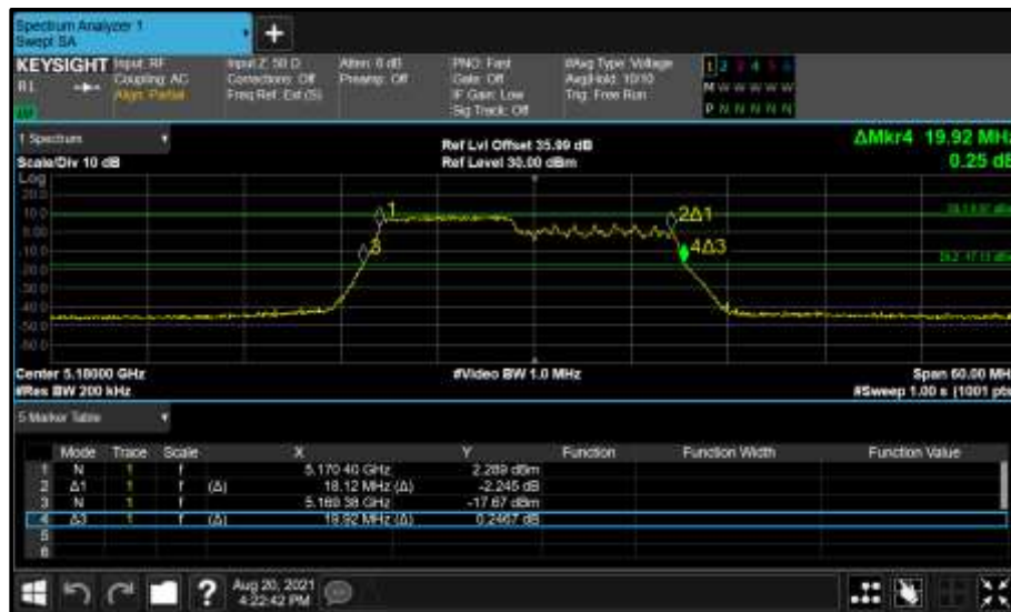
Figure 260 - Core 1 (B) 5180 MHz (CH36) 26 dB and 99% Bandwidth
