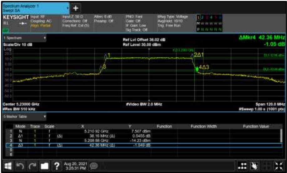
Figure 272 - Core 0 (A) 5230 MHz (CH46) 26 dB and 99% Bandwidth
