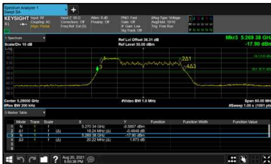
Figure 374 - Core 0 (A) 5280 MHz (CH56) 26 dB and 99% Bandwidth
