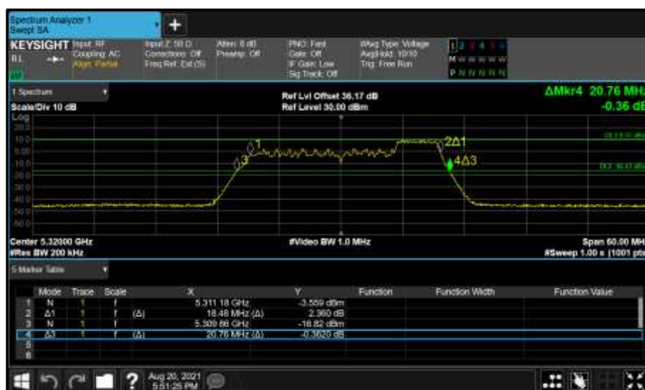
Figure 375 - Core 0 (A) 5320 MHz (CH64) 26 dB and 99% Bandwidth
