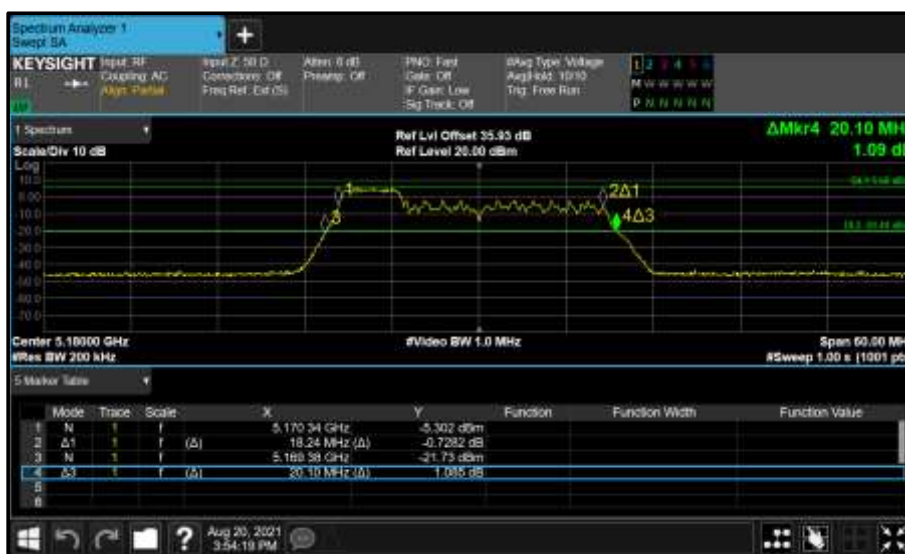
Figure 217 - Core 0 (A) 5180 MHz (CH36) 26 dB and 99% Bandwidth
