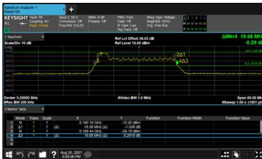
Figure 196 - Core 1 (B) 5200 MHz (CH40) 26 dB and 99% Bandwidth
