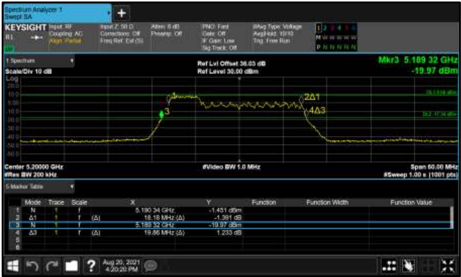
Figure 232 - Core 1 (B) 5200 MHz (CH40) 26 dB and 99% Bandwidth
