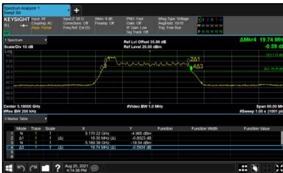
Figure 200 - Core 1 (B) 5180 MHz (CH36) 26 dB and 99% Bandwidth
