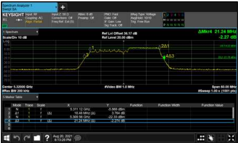
Figure 395 - Core 0 (A) 5320 MHz (CH64) 26 dB and 99% Bandwidth
