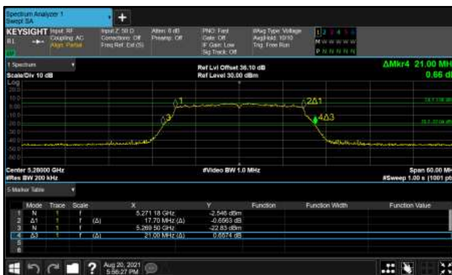
Figure 334 - Core 1 (B) 5280 MHz (CH56) 26 dB and 99% Bandwidth
