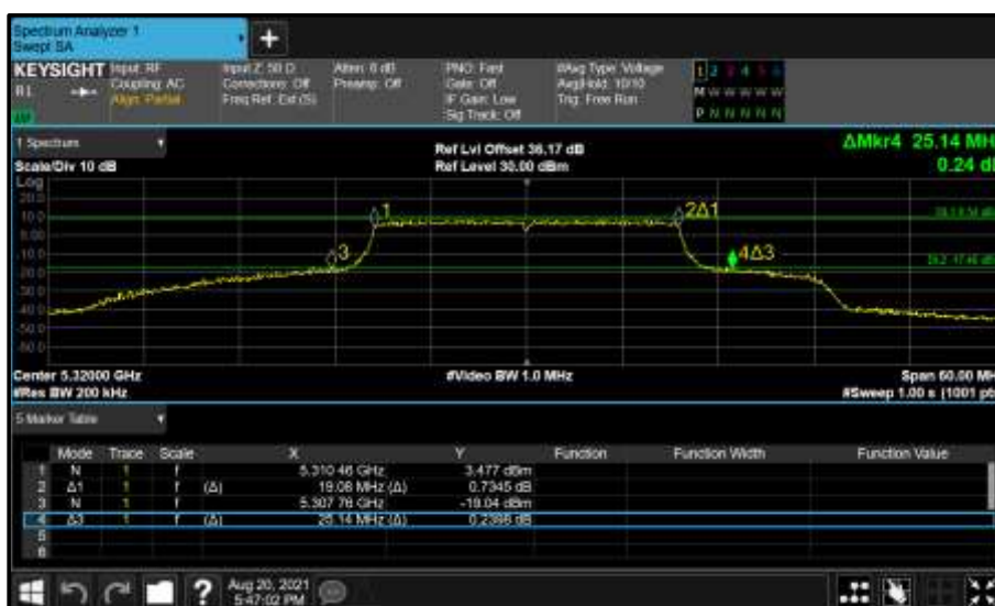
Figure 360 - Core 0 (A) 5320 MHz (CH64) 26 dB and 99% Bandwidth
