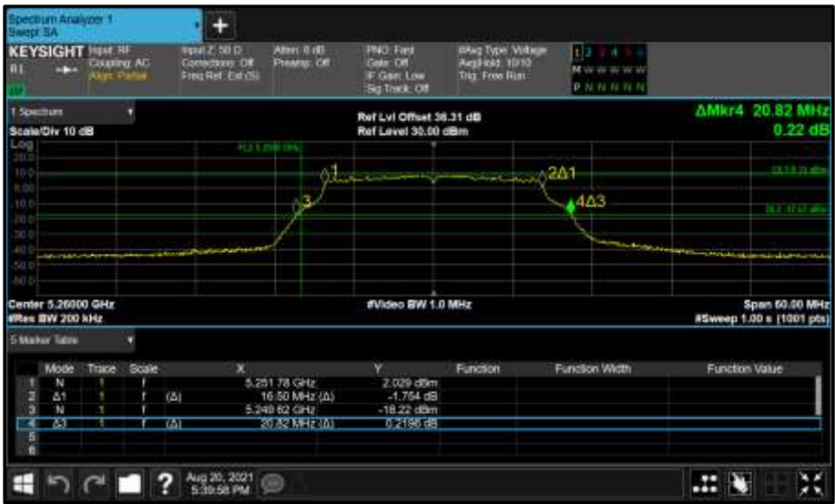
Figure 325 - Core 0 (A) 5260 MHz (CH52) 26 dB and 99% Bandwidth
