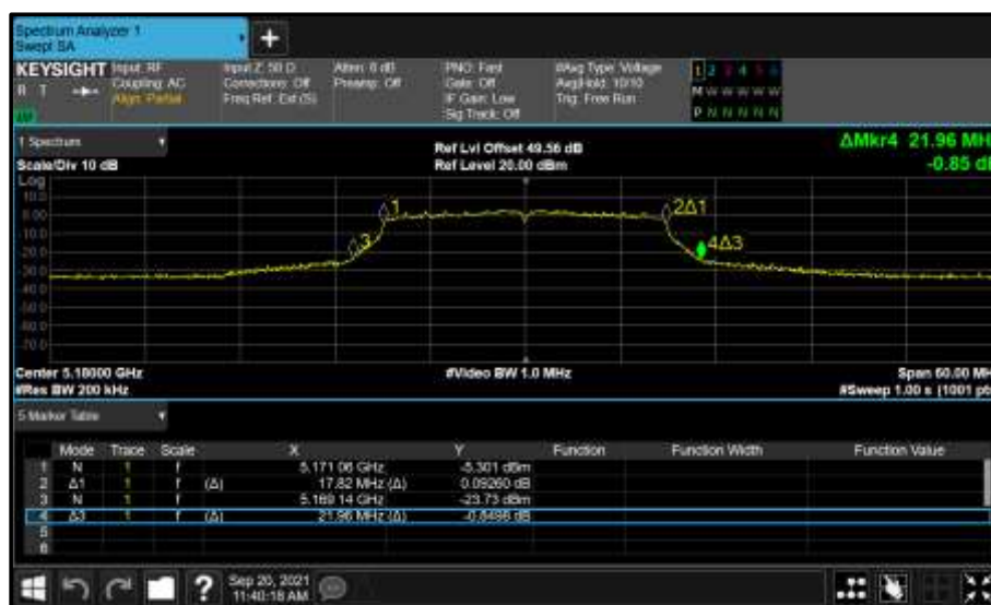
Figure 301 - Core 0 (A) 5180 MHz (CH36) 26 dB and 99% Bandwidth
