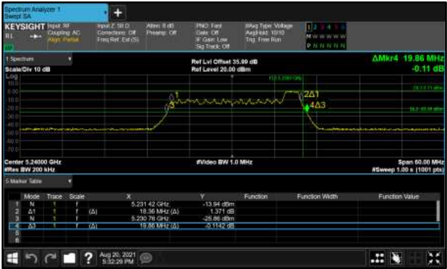
Figure 210 - Core 1 (B) 5240 MHz (CH48) 26 dB and 99% Bandwidth
