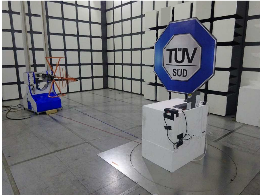
Figure 1 - Radiated Disturbance - Below 1 GHz
