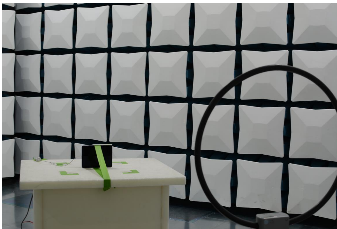
Figure 24: 9kHz-30MHz Test Setup (Front View)
