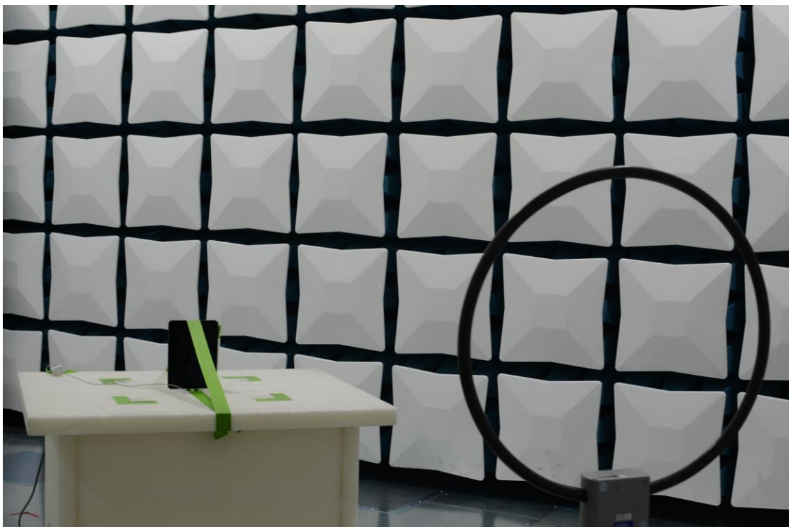
Figure 25: 9kHz-30MHz Test Setup (Front View)
