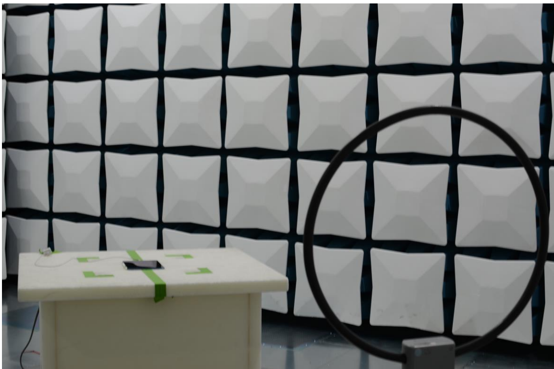
Figure 23: 9kHz-30MHz Test Setup (Front View)
