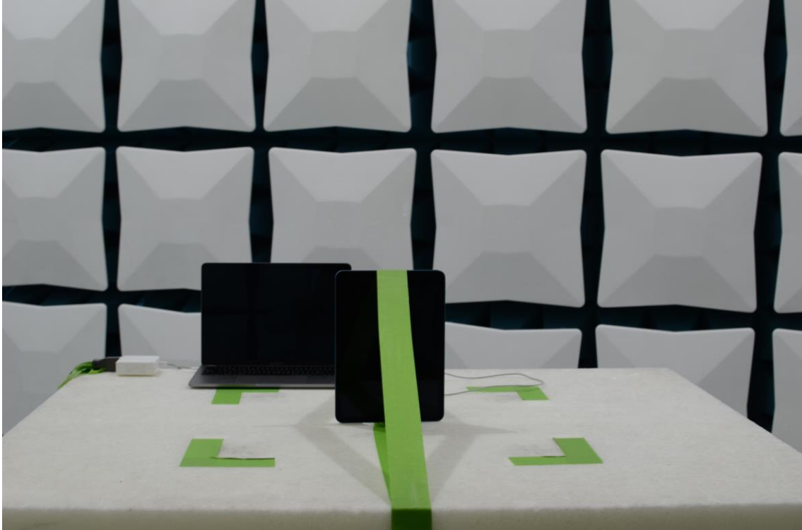
Figure 21: 30MHz-1GHz Test Setup (Front View)
