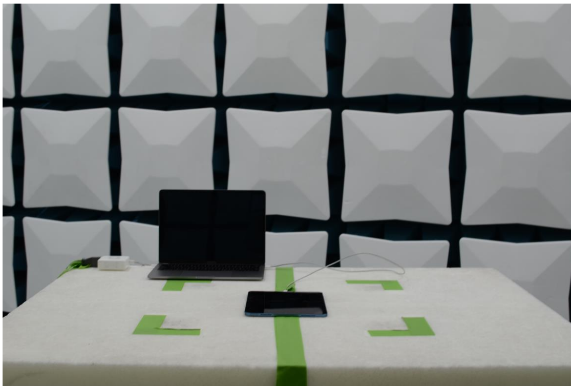
Figure 17: 30MHz-1GHz Test Setup (Front View)
