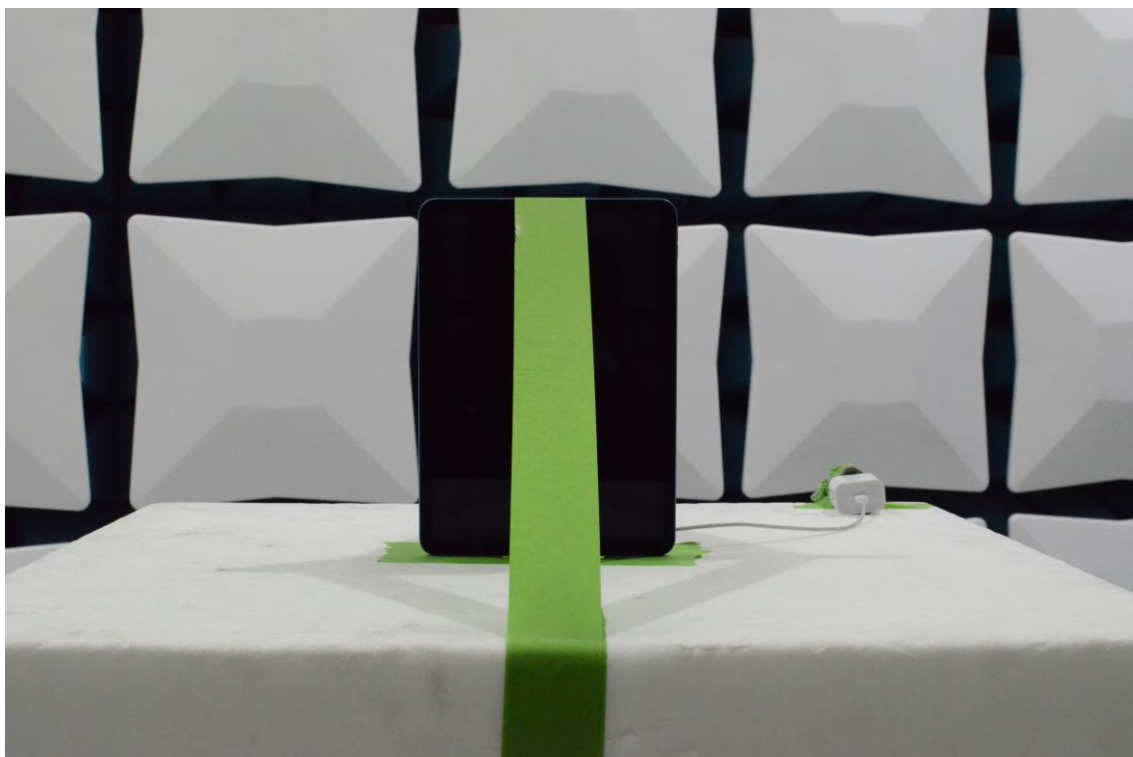
Figure 9: 1-18GHz Test Setup (Front View)
