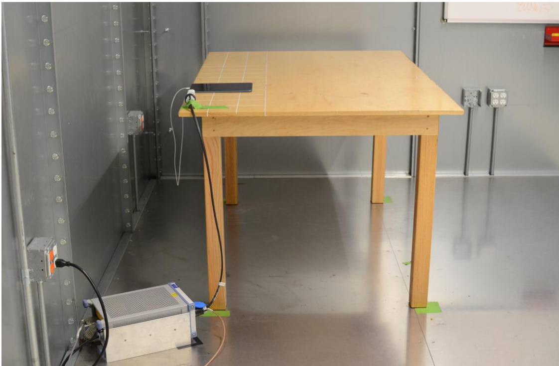
Figure 2: AC Line Conducted Emissions (Side View)
