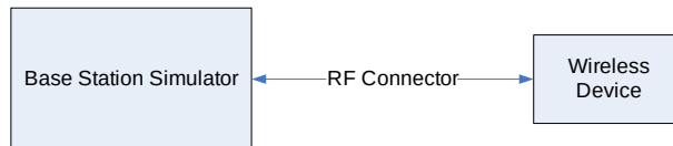
Figure 8-1 Power Measurement Setup
