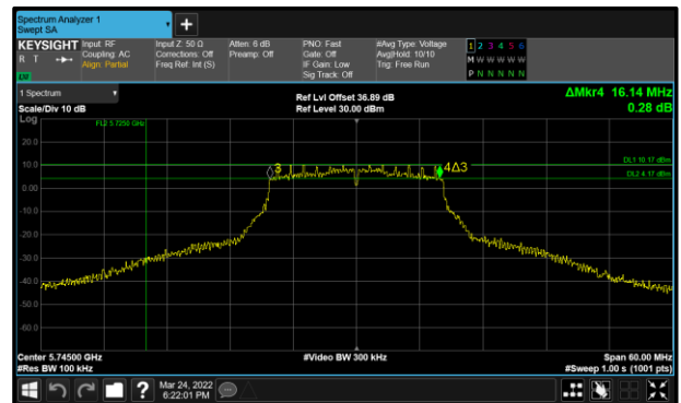
Figure 86 - 802.11a Maximum 6 dB EBW
