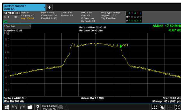
Figure 45 - 802.11n HT20 Minimum 99% OBW
