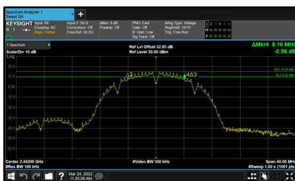
Figure 33 - 802.11b Minimum 6 dB EBW
