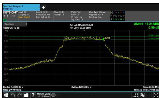
Figure 35 - 802.11g Minimum 6 dB EBW
