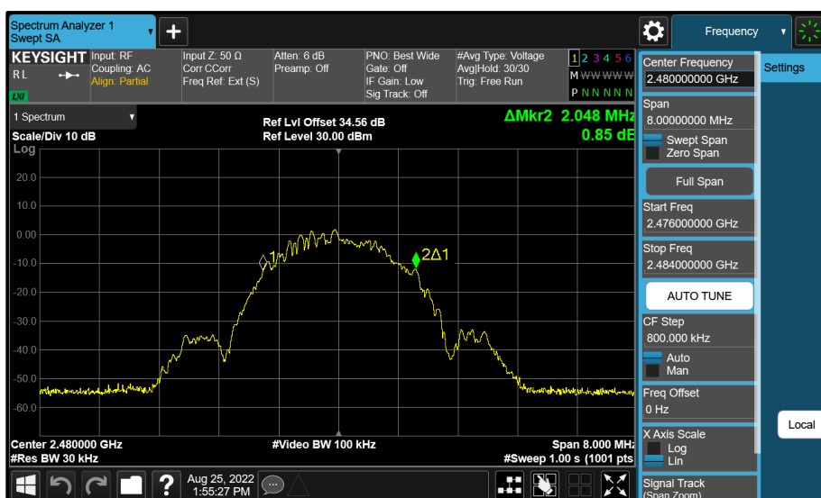
Figure 91 - BT Core 2 (C) 2480 MHz (CH39) 99% Bandwidth
