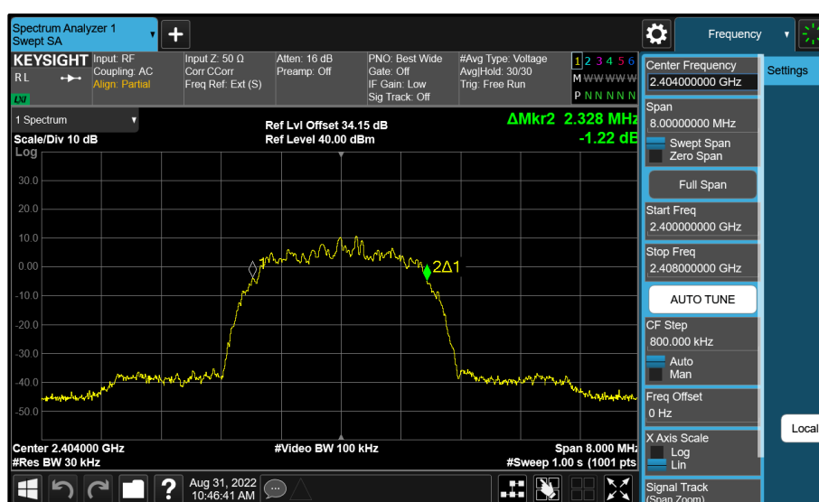
Figure 93 - Core 0 (A) 2404 MHz (CH2) 99% Bandwidth
