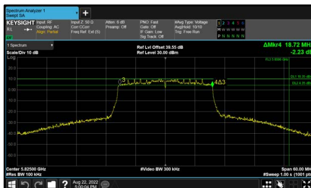
Figure 166 - 802.11ax HE20 SU Minimum 6 dB EBW
