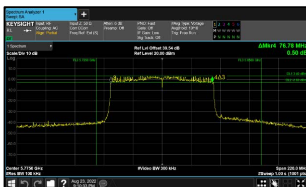
Figure 198 - 802.11ax HE80 SU Minimum 6 dB EBW
