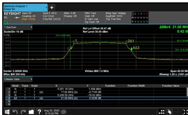
Figure 172 - 802.11n HT20 Minimum 99% OBW
