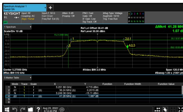
Figure 146 - 802.11n HT40 Minimum 99% OBW
