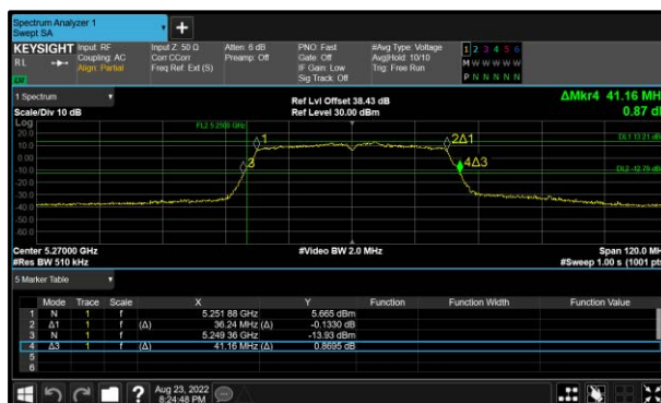
Figure 174 - 802.11n HT40 Minimum 99% OBW
