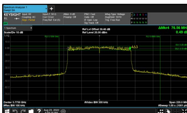
Figure 170 - 802.11ax HE80 SU Minimum 6 dB EBW
