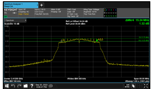
Figure 38 - 802.11n HT20 Maximum 6 dB EBW
