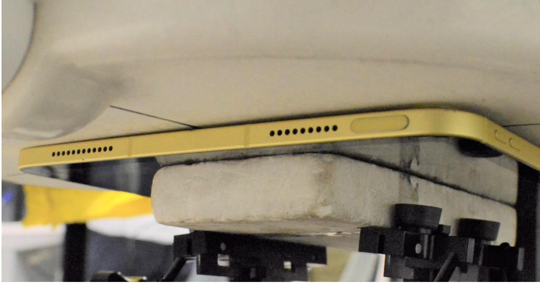
SAR Test Setup Photo 1: Body, Back Side at 0.0 cm – Antenna 3a/3b/3c/4
