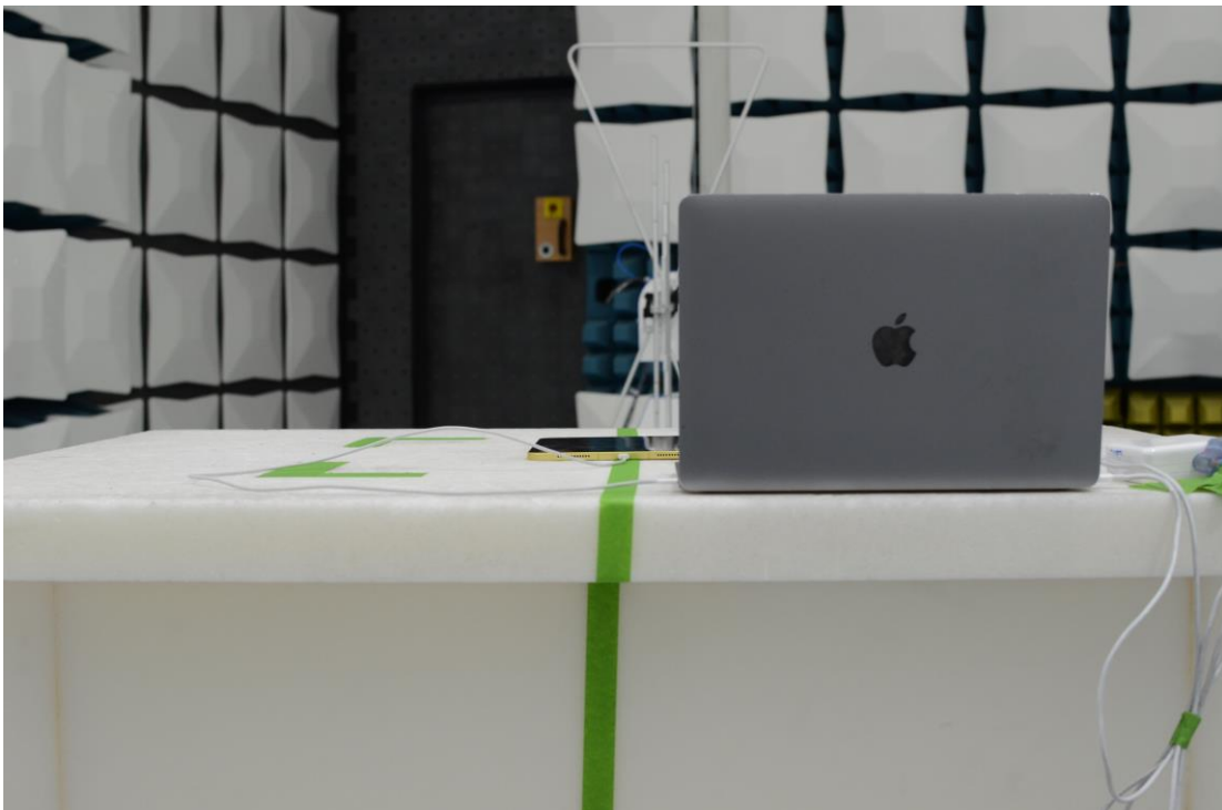
Figure 18: 30MHz-1GHz Test Setup (Rear View)
