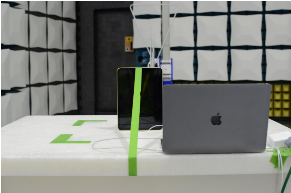
Figure 22: 30MHz-1GHz Test Setup (Rear View)
