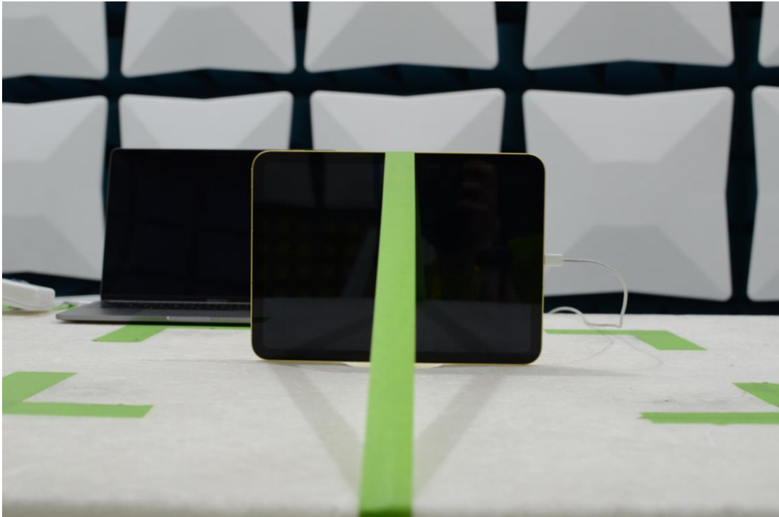
Figure 19: 30MHz-1GHz Test Setup (Front View)
