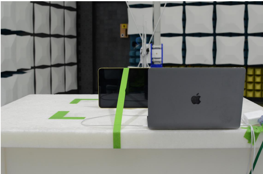
Figure 20: 30MHz-1GHz Test Setup (Rear View)
