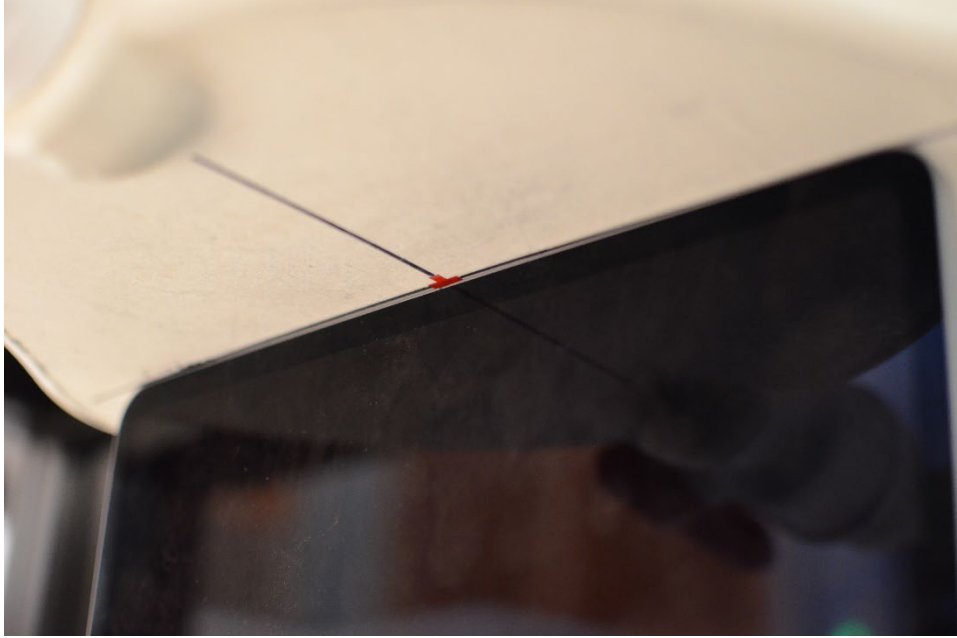
Figure F-7 SAR Test Setup Photo – Left Edge at 0mm
