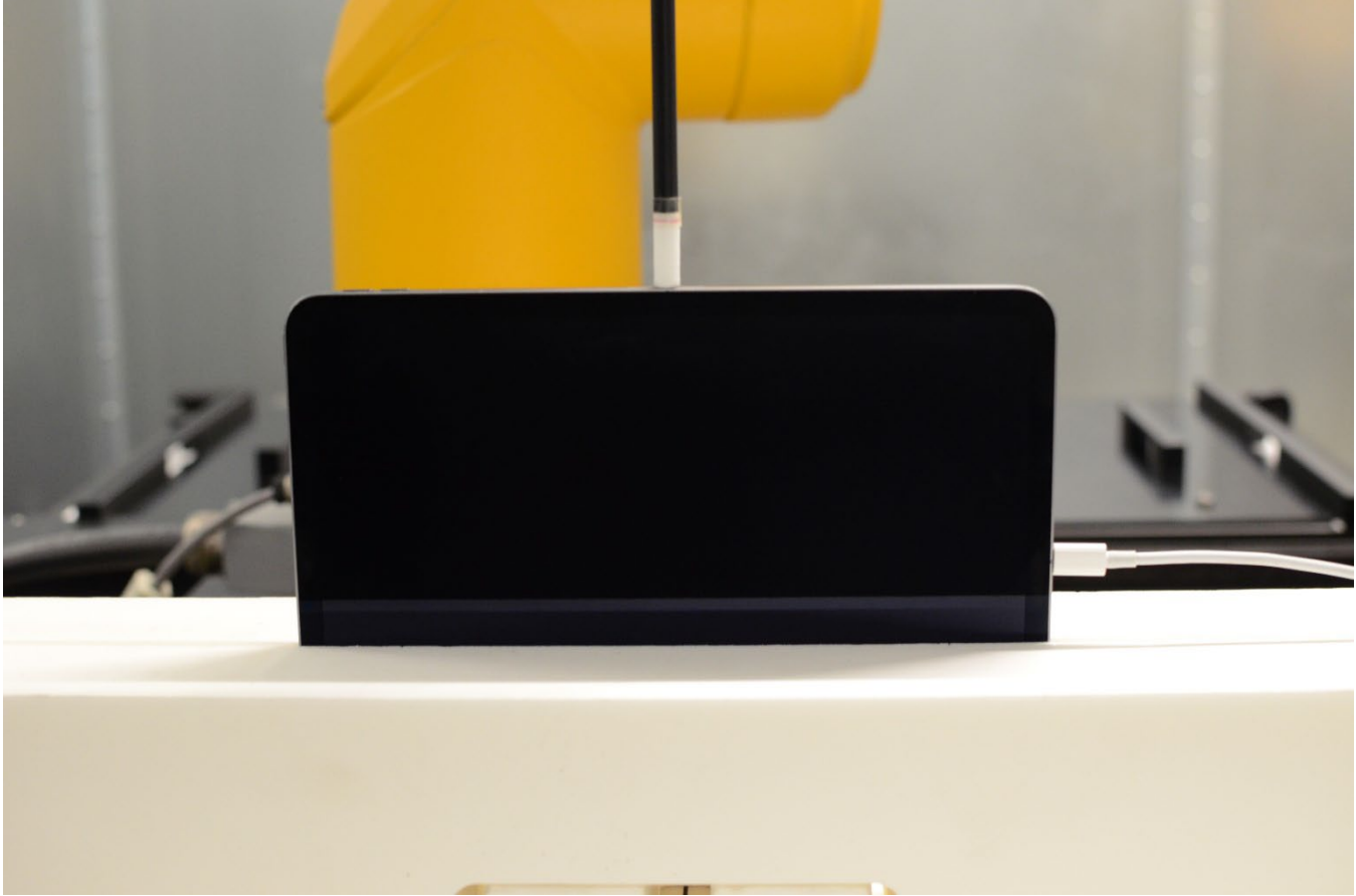
Figure F-9 Near Field Power Density Test Setup Photo – Right Edge at 2 mm
