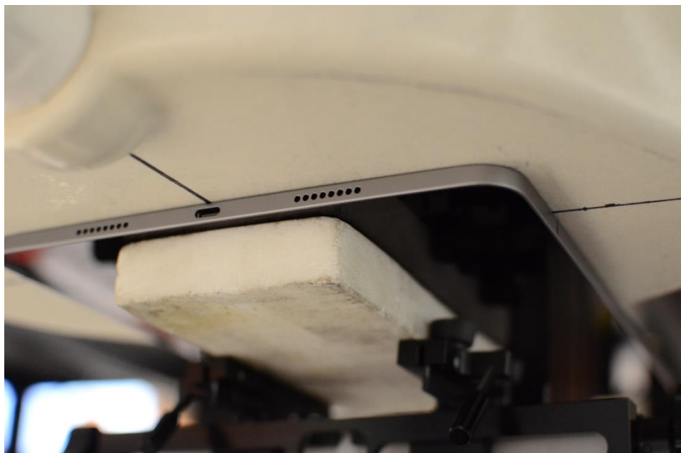
SAR Test Setup Photo 1 – Body, Back Side Antenna WF5B at 0mm
