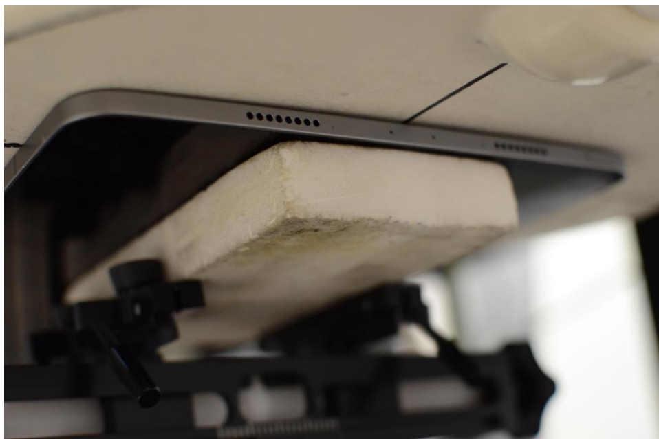
SAR Test Setup Photo 2 – Body, Back Side Antenna WF5T & WF8 & WF7 at 0mm
