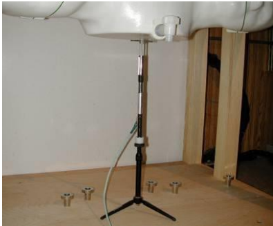
Figure 8-2 System Verification Setup Photo
