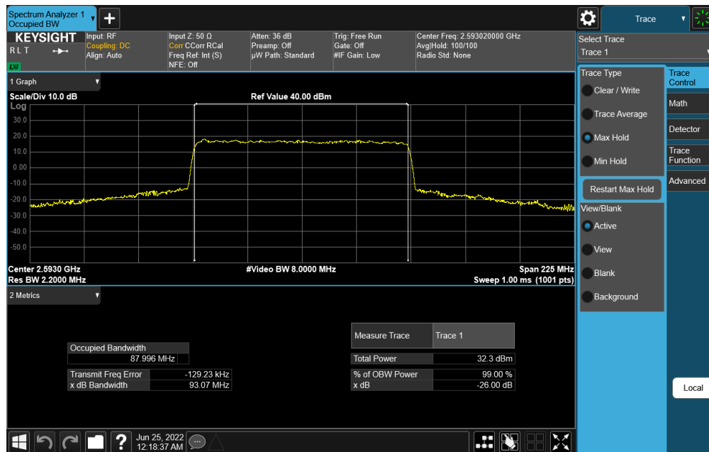
Plot 7-125. Occupied Bandwidth Plot (NR Band n41 - 90MHz CP-OFDM 256-QAM - Full RB)
