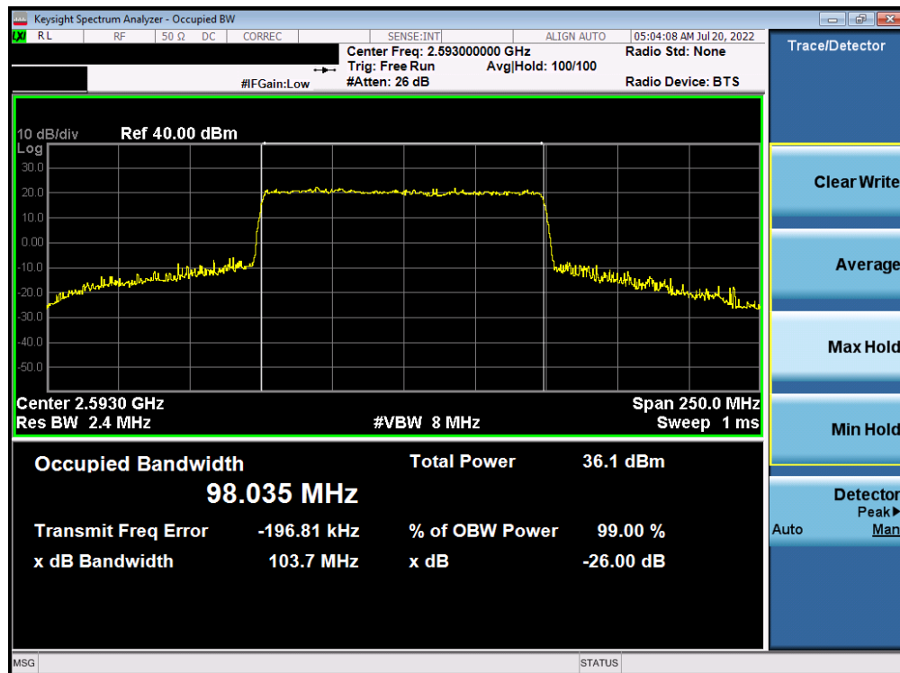
Plot 7-127. Occupied Bandwidth Plot (NR Band n41 - 100MHz CP-OFDM QPSK - Full RB)
