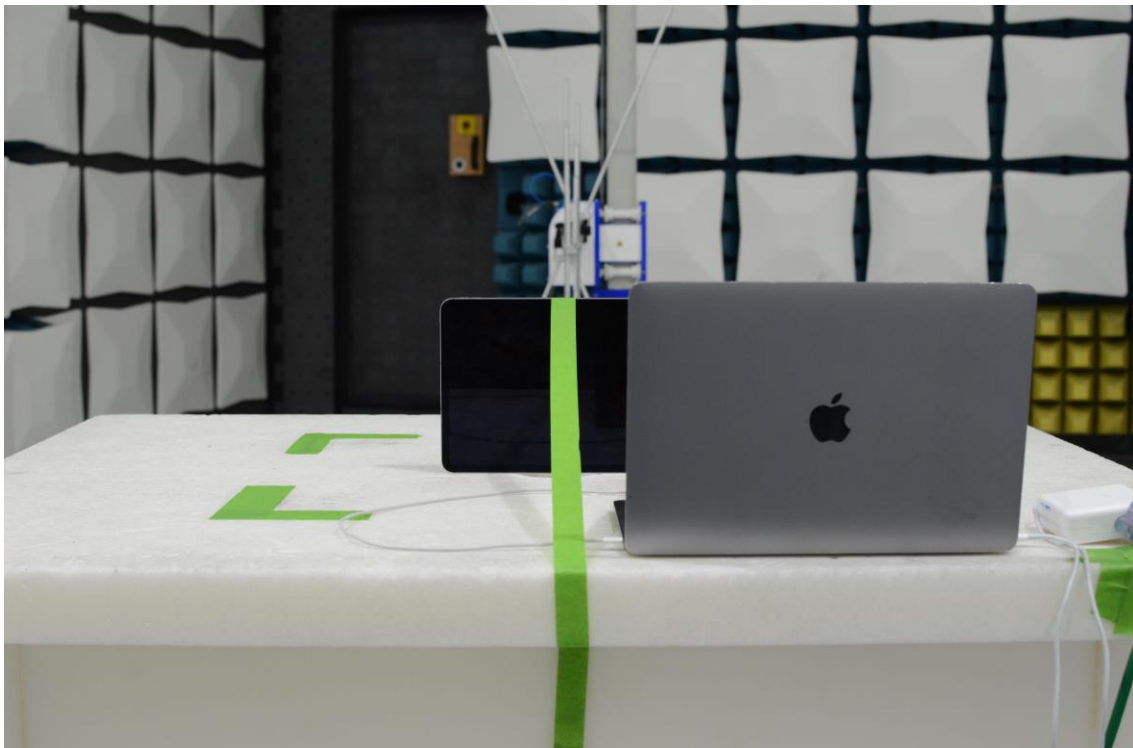
Figure 16: 30MHz-1GHz Test Setup (Rear View)
