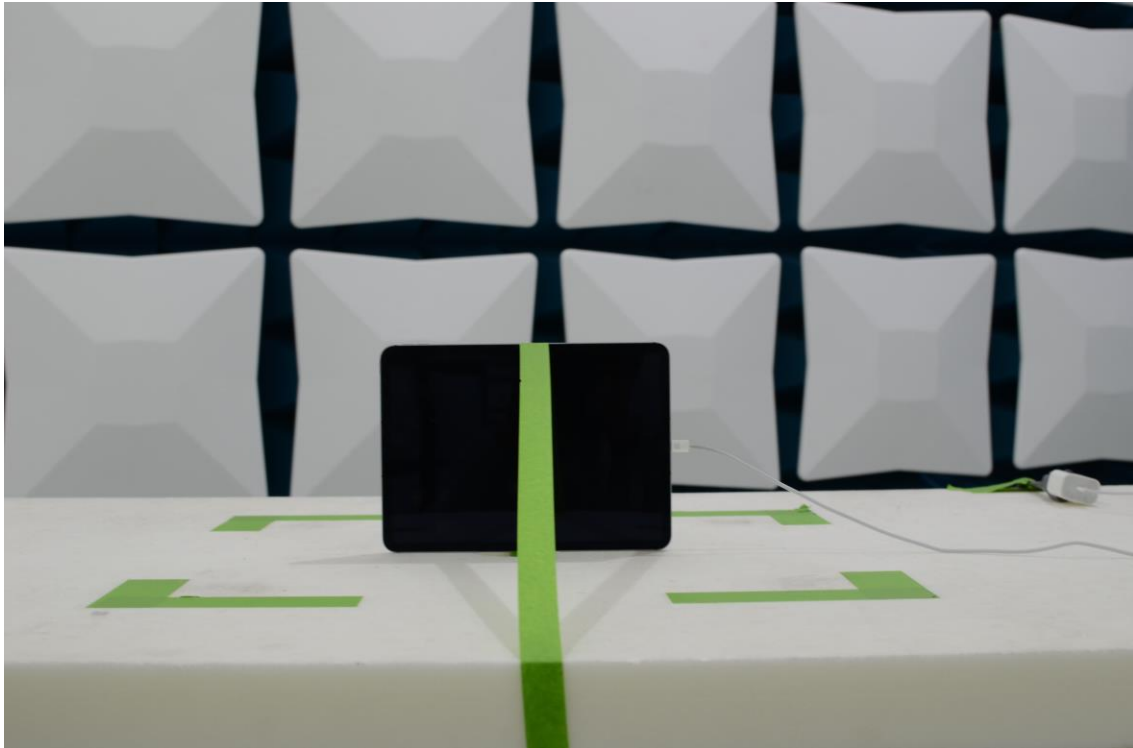
Figure 9: 30MHz-1GHz Test Setup (Front View)
