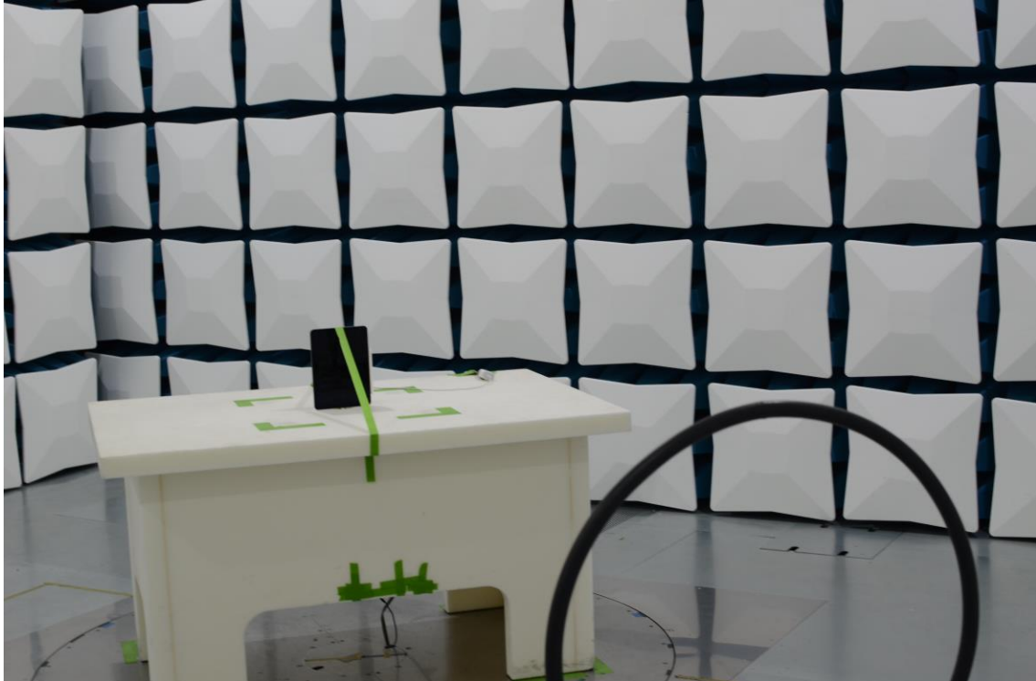
Figure 21: 9kHz-30MHz Test Setup (Front View)
