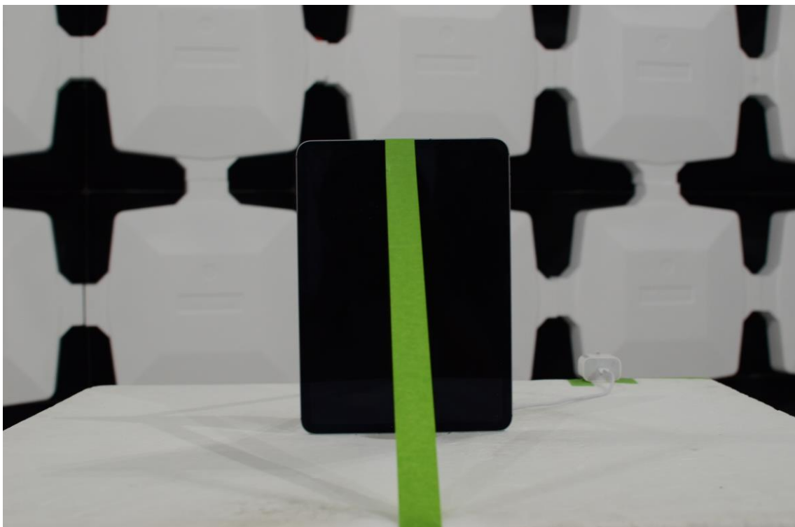
Figure 5: 1-18GHz Test Setup (Front View)
