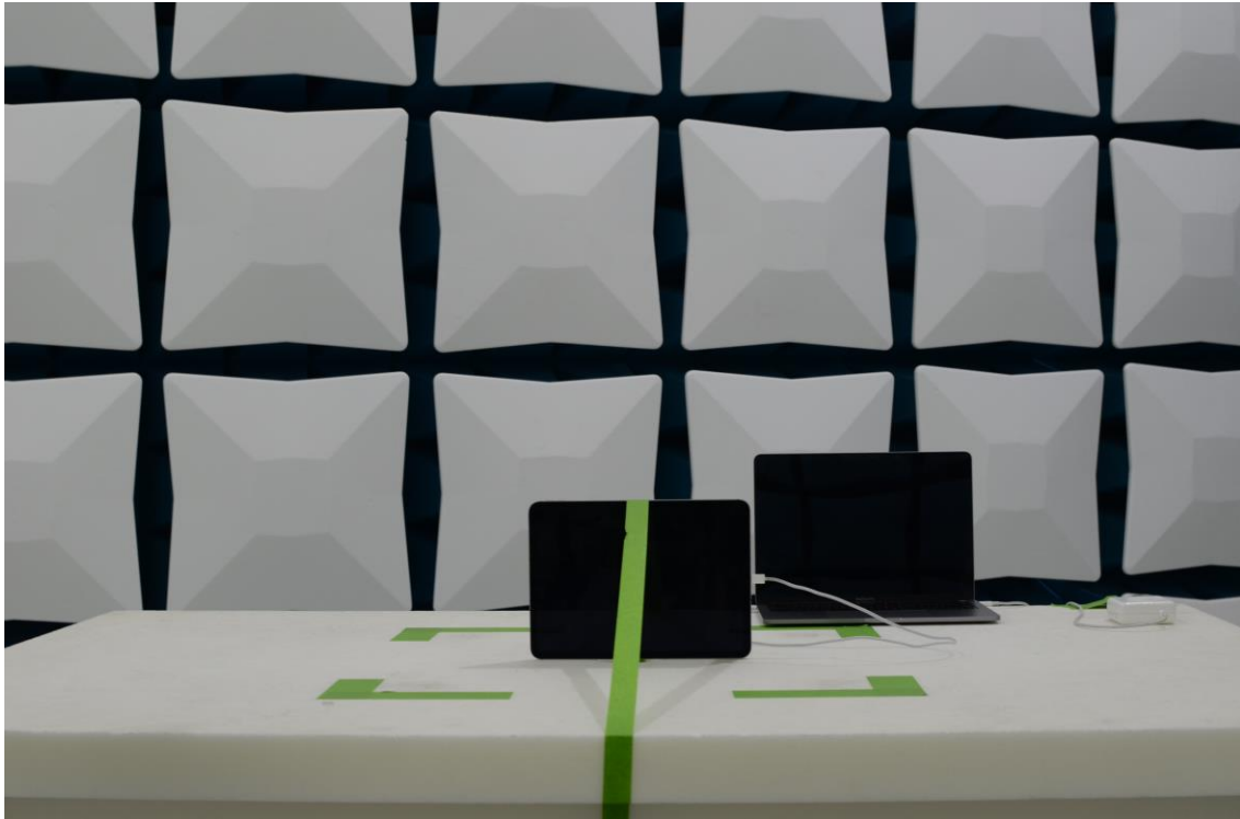
Figure 15: 30MHz-1GHz Test Setup (Front View)
