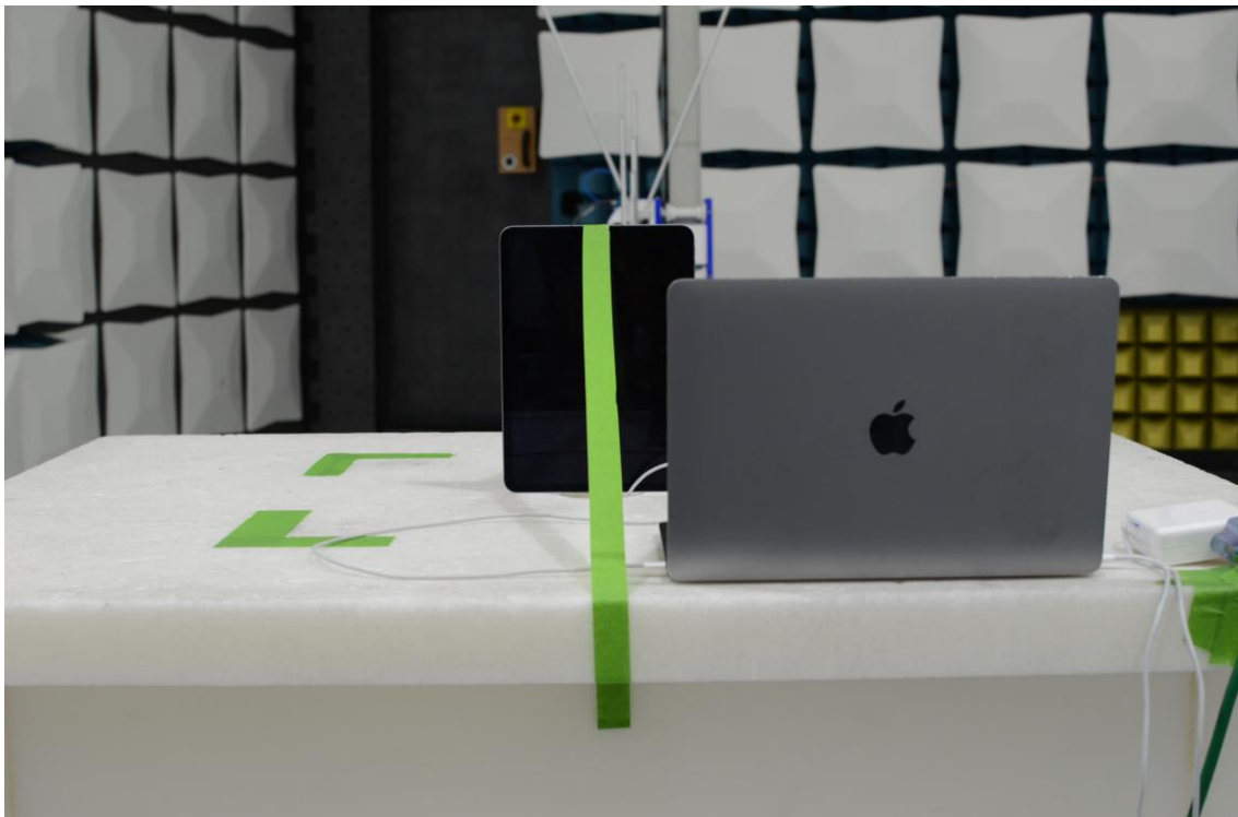
Figure 18: 30MHz-1GHz Test Setup (Rear View)
