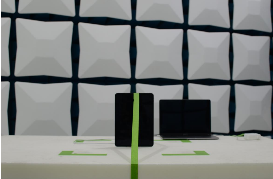
Figure 17: 30MHz-1GHz Test Setup (Front View)
