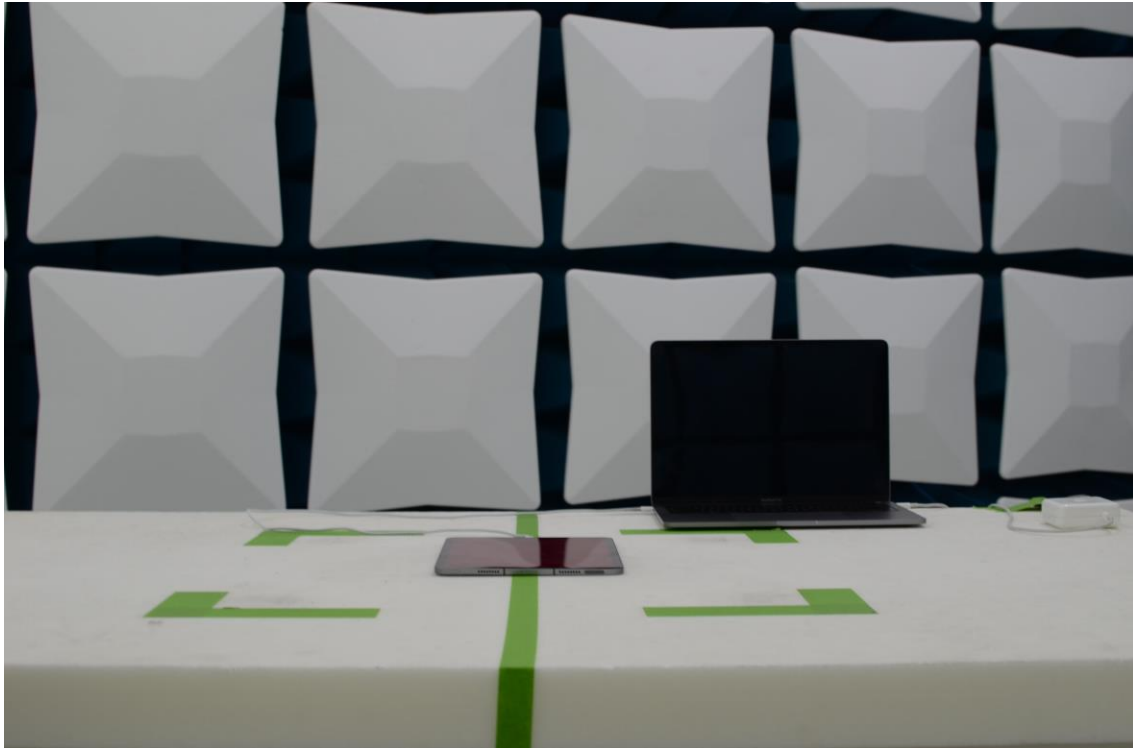
Figure 13: 30MHz-1GHz Test Setup (Front View)
