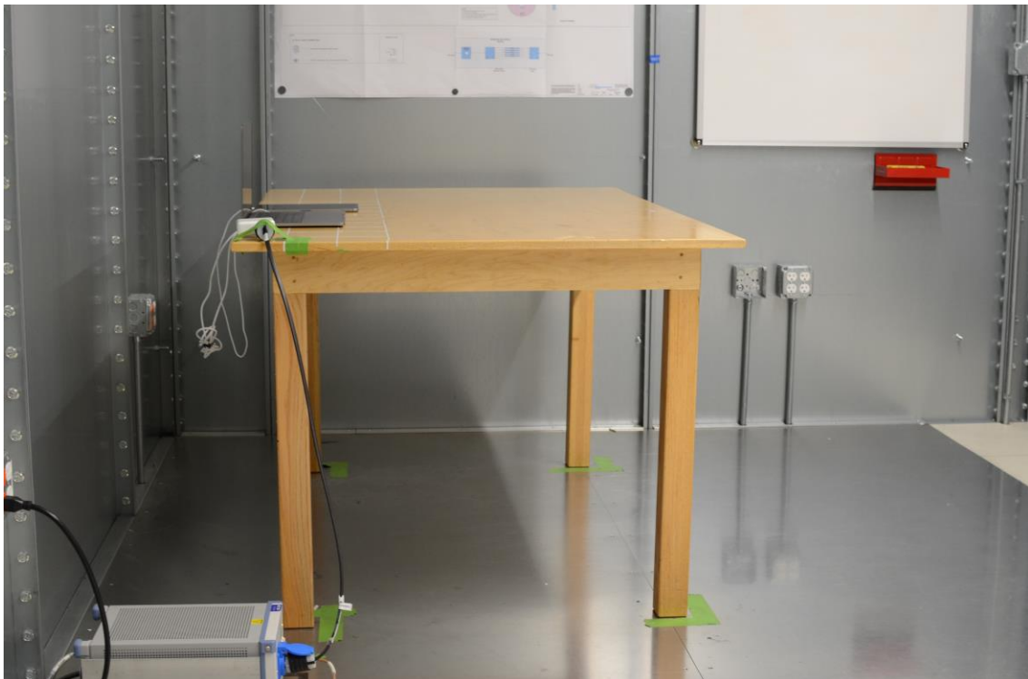
Figure 4: AC Line Conducted Emissions (Side View)
