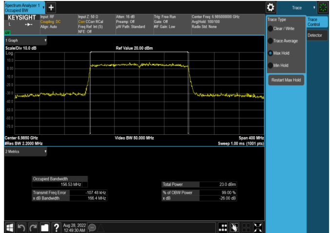
Plot 7-80. 26dB & 99% Bandwidth Plot Antenna 4a (160MHz 802.11ax (UNII Band 8) – Ch. 207, MCS2)
