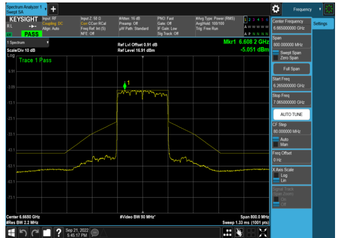
Plot 7-519. In-Band Emission Plot SDM Antenna 5b (160MHz 802.11ax (UNII Band 7) - Ch. 143, MCS4)
