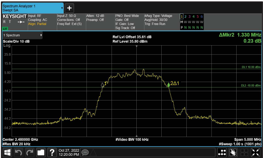
Figure 66 - Core 1 (B) 2480 MHz (CH78) 20 dB Bandwidth
