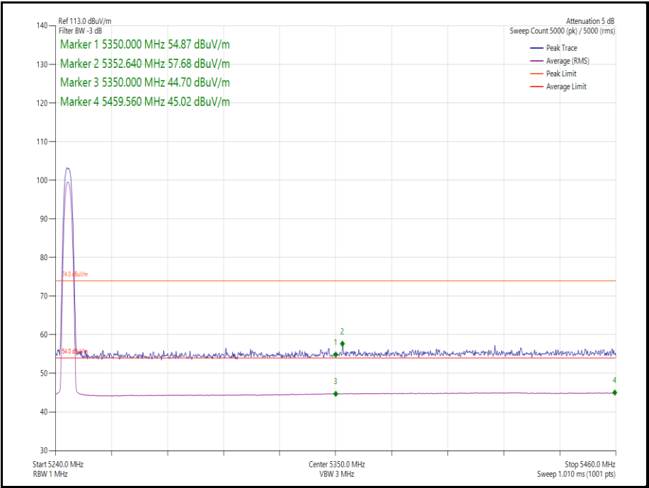
Figure 5 - Static - \pi/4 DQPSK/4-DH5 - 5245 MHz - Band Edge Frequency 5350 MHz
