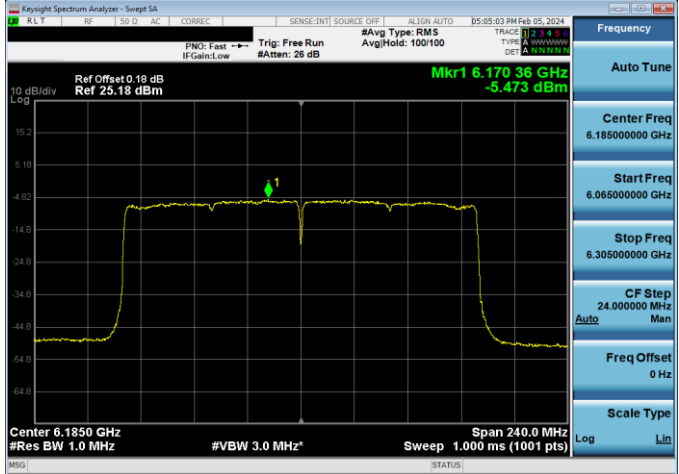
Plot 7-185. Power Spectral Density Plot LPI Antenna WF5B (160MHz 802.11ax (UNII Band 5) – Ch. 47, MCS2)
