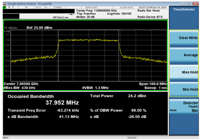
Plot 7-178. 26dB & 99% Bandwidth Plot Antenna WF7 (40MHz 802.11ax (UNII Band 8) – Ch. 211, MCS11)
