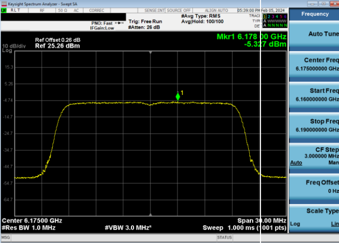
Plot 7-202. Power Spectral Density Plot LPI Antenna WF5B (20MHz 802.11ax (UNII Band 5) – Ch. 45, MCS4)
