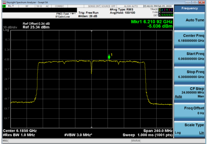
Plot 7-205. Power Spectral Density Plot LPI Antenna WF5B (160MHz 802.11ax (UNII Band 5) – Ch. 47, MCS4)
