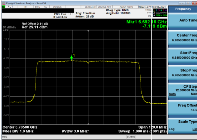
Plot 7-194. Power Spectral Density Plot LPI Antenna WF5B (80MHz 802.11ax (UNII Band 7) – Ch. 151, MCS2)
