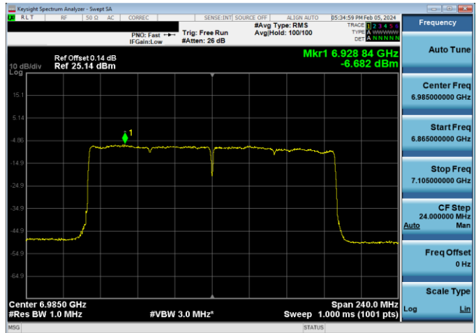
Plot 7-200. Power Spectral Density Plot LPI Antenna WF5B (160MHz 802.11ax (UNII Band 8) – Ch. 207, MCS2)
