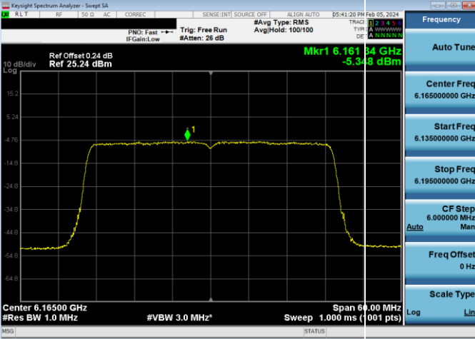
Plot 7-203. Power Spectral Density Plot LPI Antenna WF5B (40MHz 802.11ax (UNII Band 5) – Ch. 43, MCS4)
