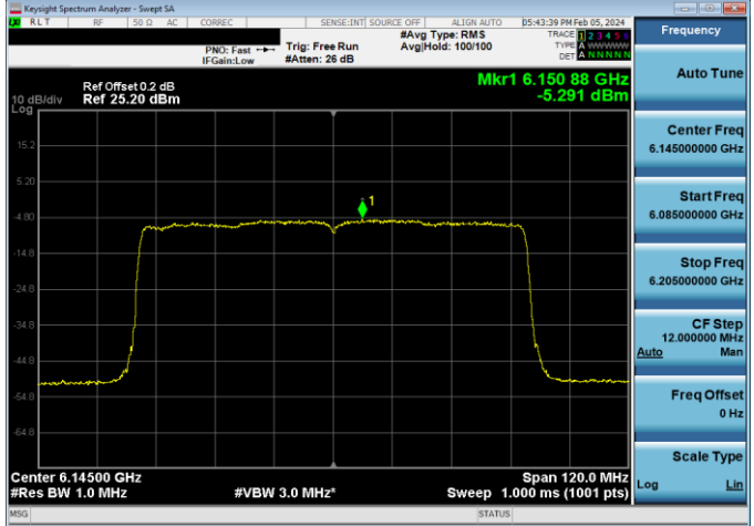
Plot 7-204. Power Spectral Density Plot LPI Antenna WF5B (80MHz 802.11ax (UNII Band 5) – Ch. 45, 24Mbps)
