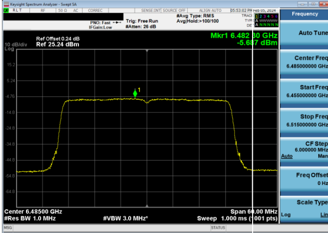
Plot 7-208. Power Spectral Density Plot LPI Antenna WF5B (40MHz 802.11ax (UNII Band 6) – Ch. 107, MCS4)
