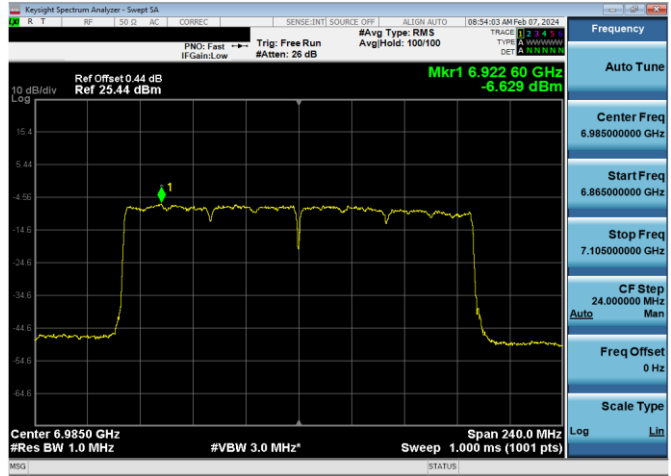
Plot 7-278. Power Spectral Density Plot LPI Antenna WF8 (160MHz 802.11ax (UNII Band 8) – Ch. 207, MCS11)
