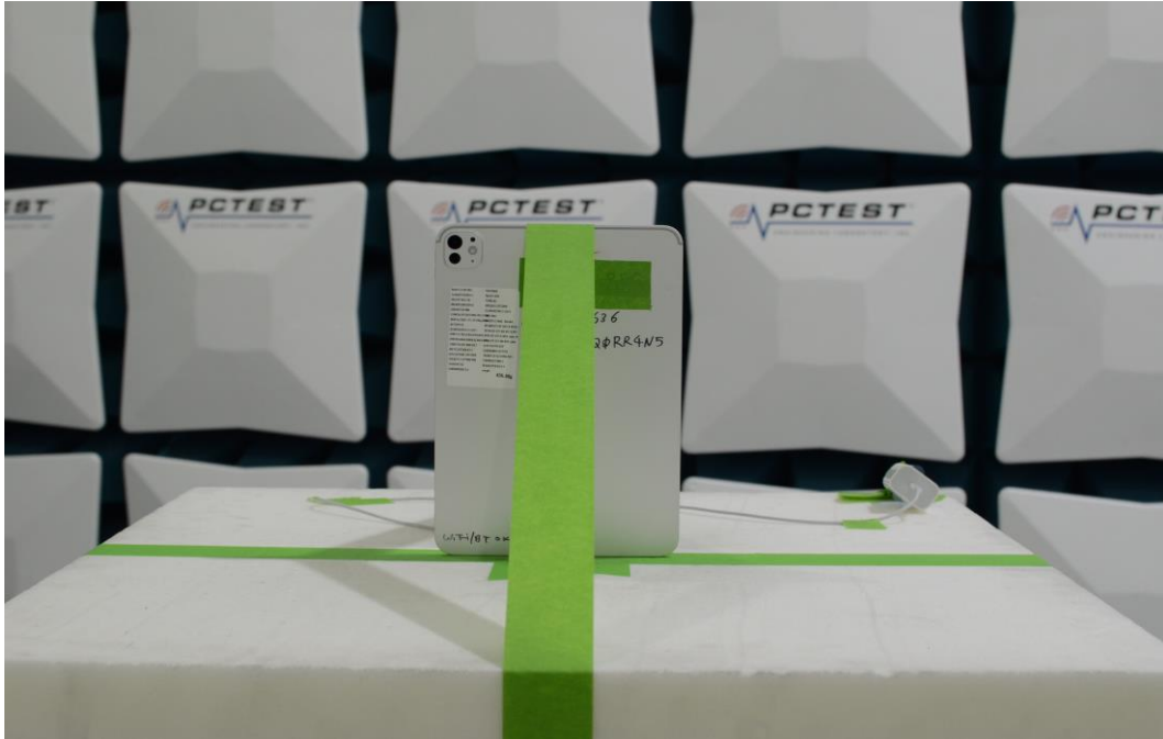
Figure 9: 1-18GHz Test Setup (Front View)
