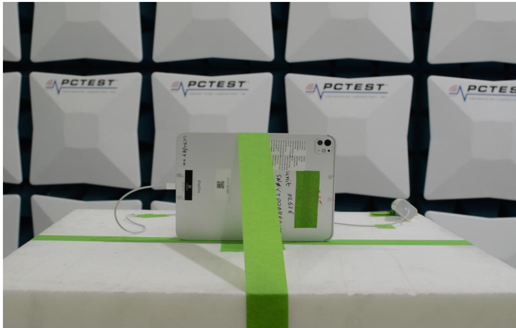
Figure 7: 1-18GHz Test Setup (Front View)
