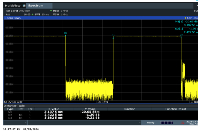
Figure 8-9 802.15.4 Transmission Plot – Antenna 4a/2a, Variant 1
