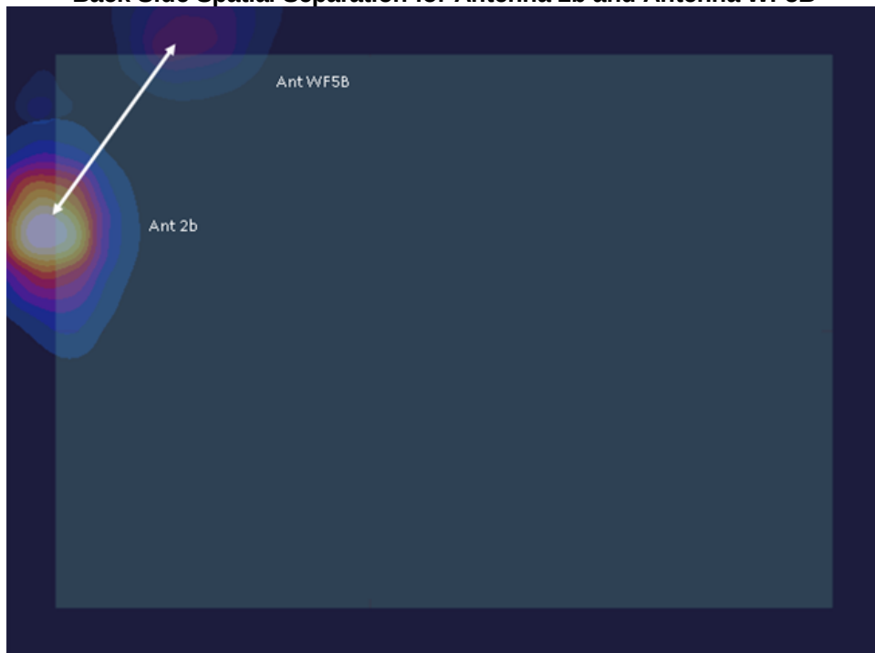
Figure 11-9 Back Side Spatial Separation for Antenna 2b and Antenna WF5B
