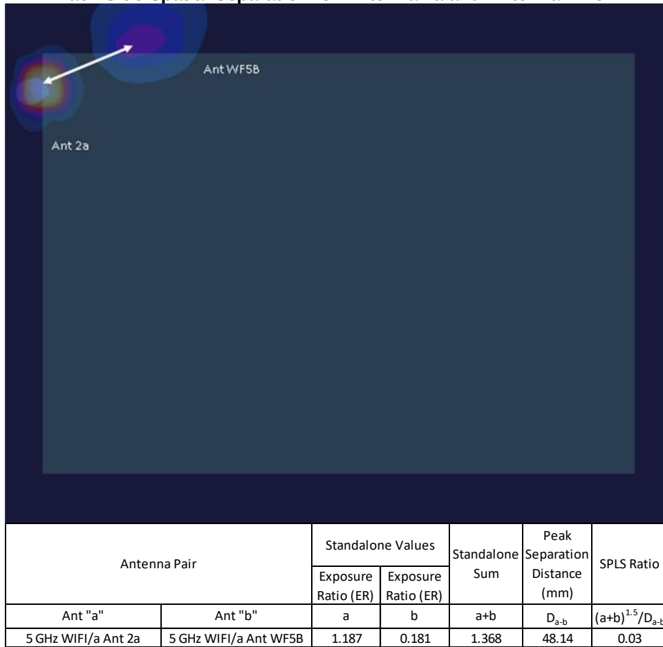
Figure 11-7 Back Side Spatial Separation for Antenna 2a and Antenna WF5B
