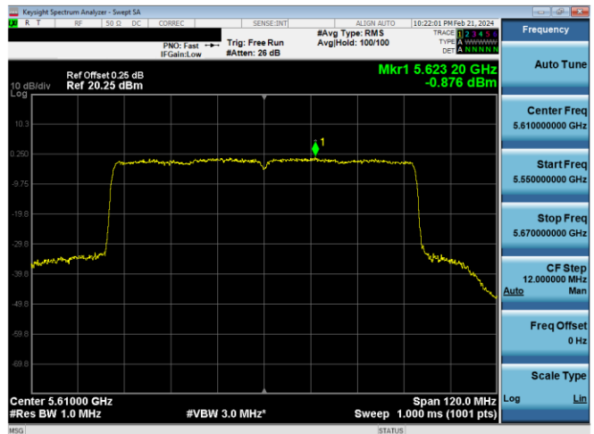
Plot 7-509. PSD Antenna 2a (80MHz BW 802.11ax(SU) – Ch. 122, MCS4)
