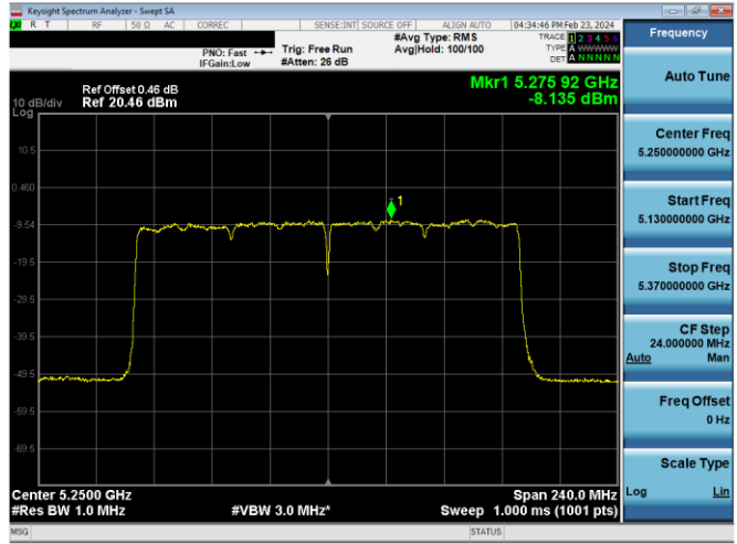
Plot 7-467. ISED PSD Antenna 4a (160MHz BW 11ax (SU) – Ch.50, MCS11)
