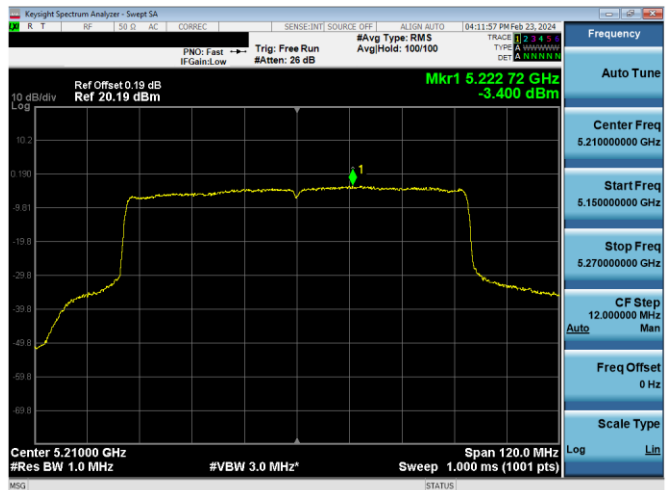
Plot 7-449. ISED PSD Antenna 4a (80MHz BW 11ax (SU) – Ch.42, MCS2)
