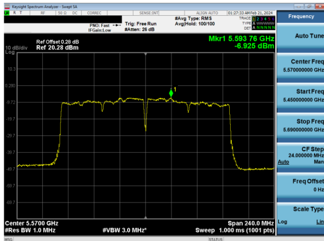
Plot 7-659. PSD CDD Primary Antenna WF5b (160MHz BW 802.11ac – Ch. 114, MCS4)
