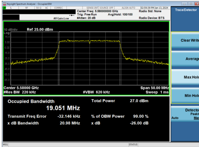
Plot 7-76. 26dB BW & 99% OBW Antenna 4a (20MHz BW 11ax – RU242 – Ch.116)
