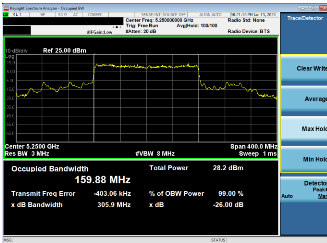
Plot 7-104. 26dB BW & 99% OBW Antenna 2a (160MHz BW 11ax - RU996x2 - Ch.50)
