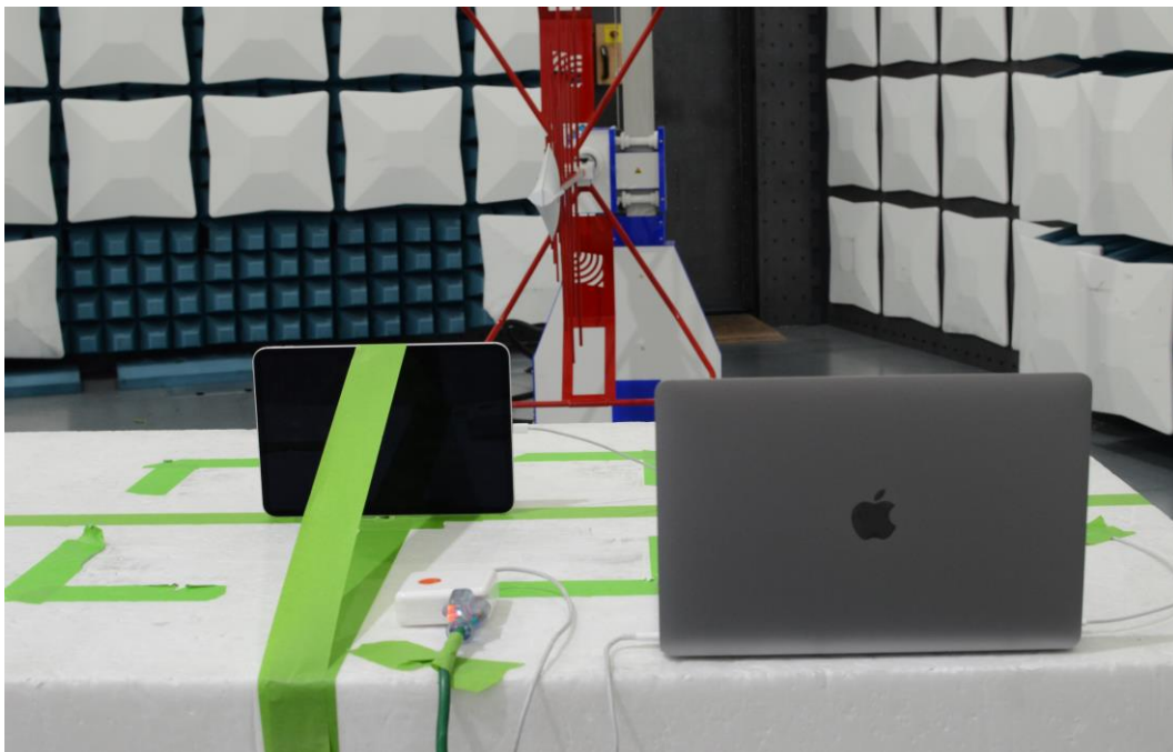
Figure 20: 30MHz-1GHz Test Setup (Rear View)
