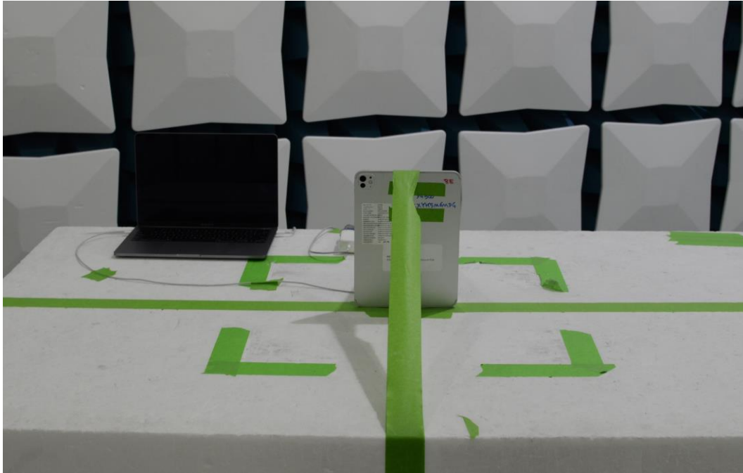
Figure 21: 30MHz-1GHz Test Setup (Front View)
