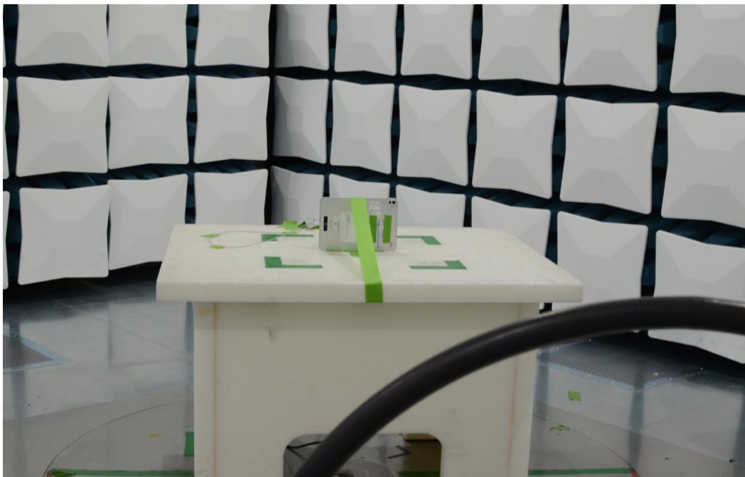
Figure 24: 9kHz-30MHz Test Setup (Front View)
