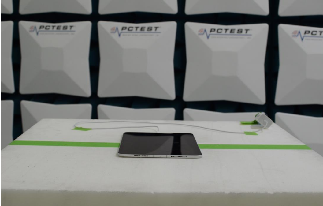
Figure 5: 1-18GHz Test Setup (Front View)
