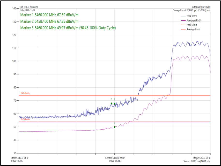
Figure 27 - 802.11ax HE20 CDD, Cores 0-1, SU- 5500 MHz Band Edge Frequency 5460 MHz
