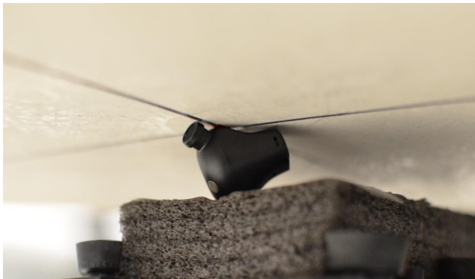
SAR Test Setup Photo 1: Head, Left Earbud, 0 mm
