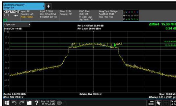
Figure 69 - 802.11n HT20 Minimum 6 dB EBW
