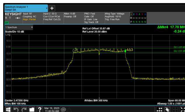
Figure 58 - 802.11n HT20 Maximum 6 dB EBW
