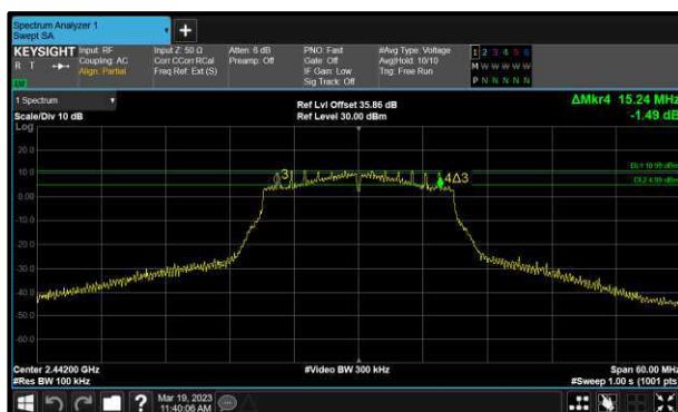
Figure 57 - 802.11n HT20 Minimum 6 dB EBW
