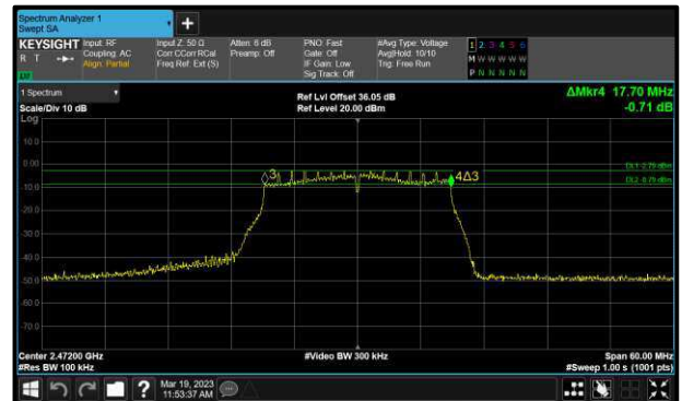
Figure 70 - 802.11n HT20 Maximum 6 dB EBW
