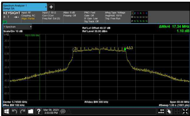
Figure 179 - 802.11n HT20 Minimum 6 dB EBW
