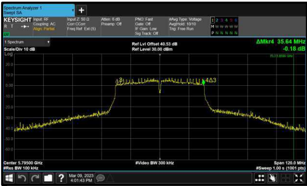
Figure 182 - 802.11n HT40 Maximum 6 dB EBW
