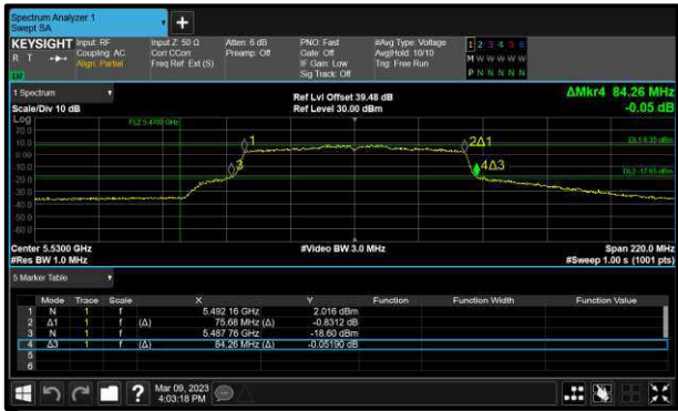
Figure 197 - 802.11ac VHT80 Minimum 99% OBW
