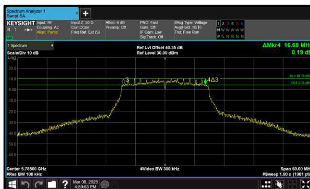
Figure 209 - 802.11n HT20 Minimum 6 dB EBW
