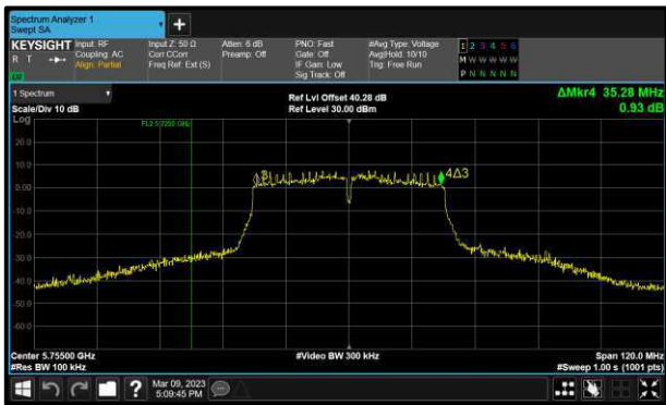
Figure 211 - 802.11n HT40 Minimum 6 dB EBW
