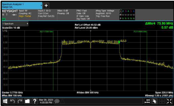
Figure 184 - 802.11ac VHT80 Maximum 6 dB EBW
