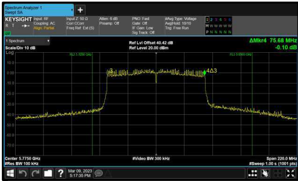
Figure 213 - 802.11ac VHT80 Minimum 6 dB EBW
