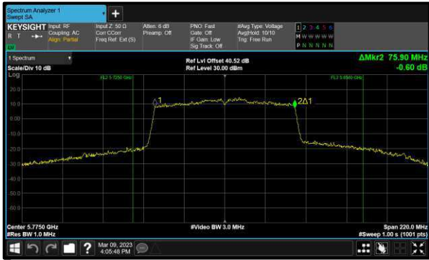
Figure 183 - 802.11ac VHT80 Minimum 6 dB EBW
