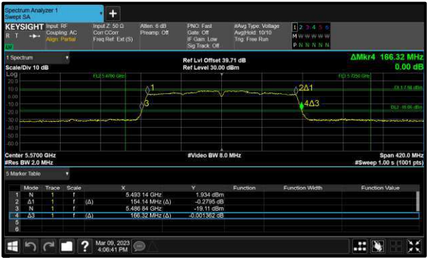
Figure 200 - 802.11ac VHT160 Maximum 99% OBW
