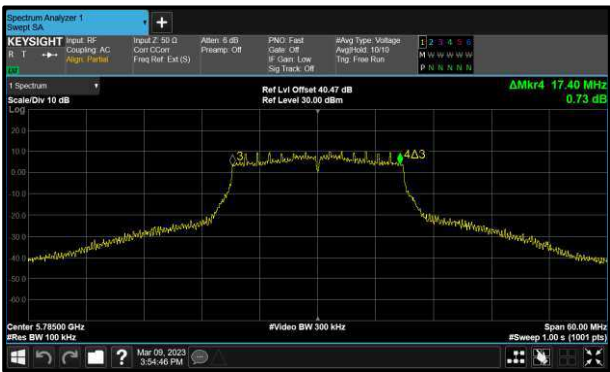
Figure 180 - 802.11n HT20 Maximum 6 dB EBW
