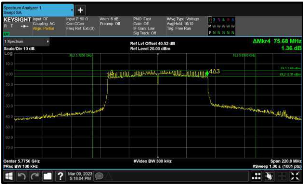
Figure 214 - 802.11ac VHT80 Maximum 6 dB EBW
