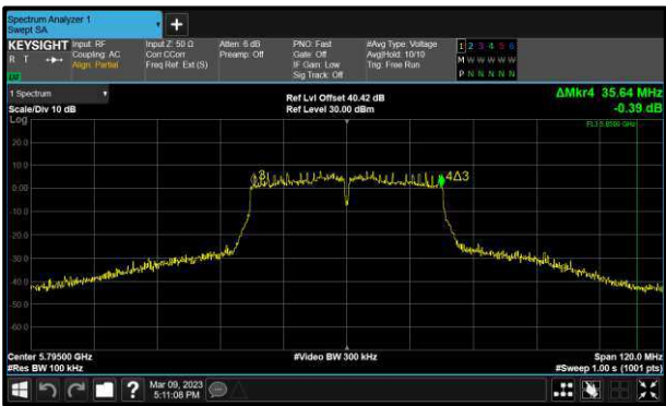
Figure 212 - 802.11n HT40 Maximum 6 dB EBW
