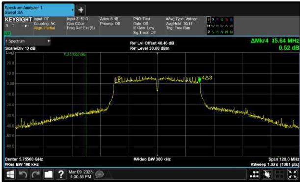
Figure 181 - 802.11n HT40 Minimum 6 dB EBW
