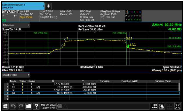
Figure 198 - 802.11ac VHT80 Maximum 99% OBW
