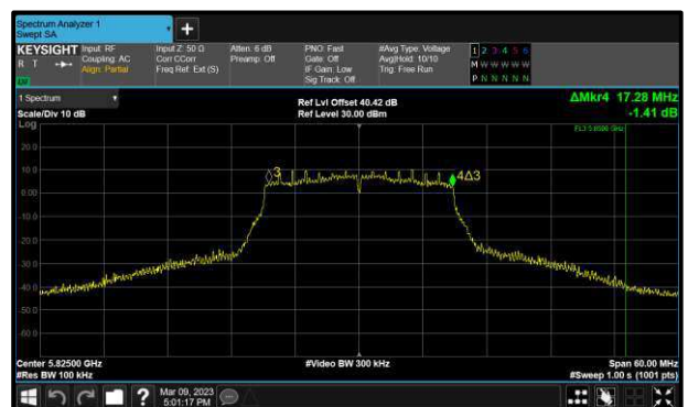
Figure 210 - 802.11n HT20 Maximum 6 dB EBW
