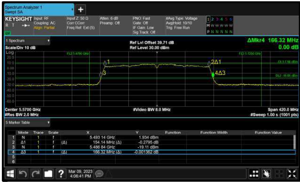
Figure 199 - 802.11ac VHT160 Minimum 99% OBW
