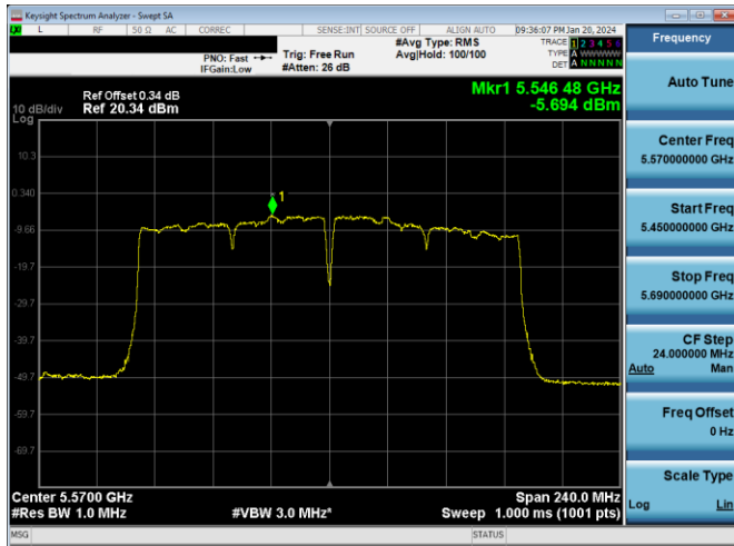
Plot 7-661. PSD CDD PRIMARY Antenna WF7a (160MHz BW 802.11ac - Ch. 114, MCS4)
