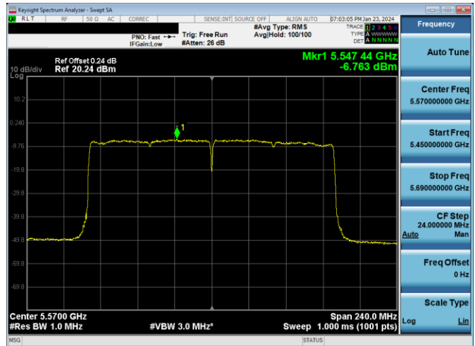
Plot 7-802. PSD CDD DIVERSITY Antenna WF2a (160MHz BW 802.11ax(SU) - Ch. 114, MCS2)
