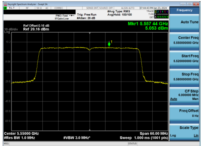
Plot 7-820. PSD CDD DIVERSITY Antenna WF2a (40MHz BW 802.11ax(SU) – Ch. 110, MCS4)
