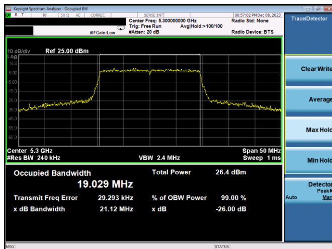
Plot 7-108. 26dB BW & 99% OBW Antenna WF7b (20MHz BW 11ax– RU242 – Ch.60)
