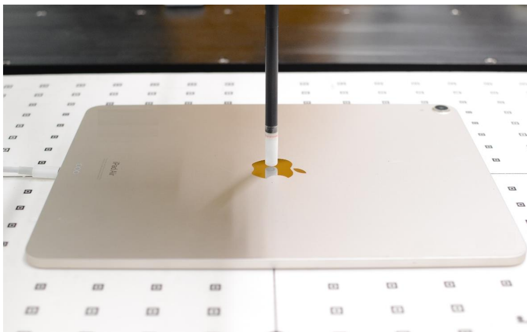
Near Field Power Density Test Setup Photo 16: Backside at 2mm – WF7a/7b/2a
