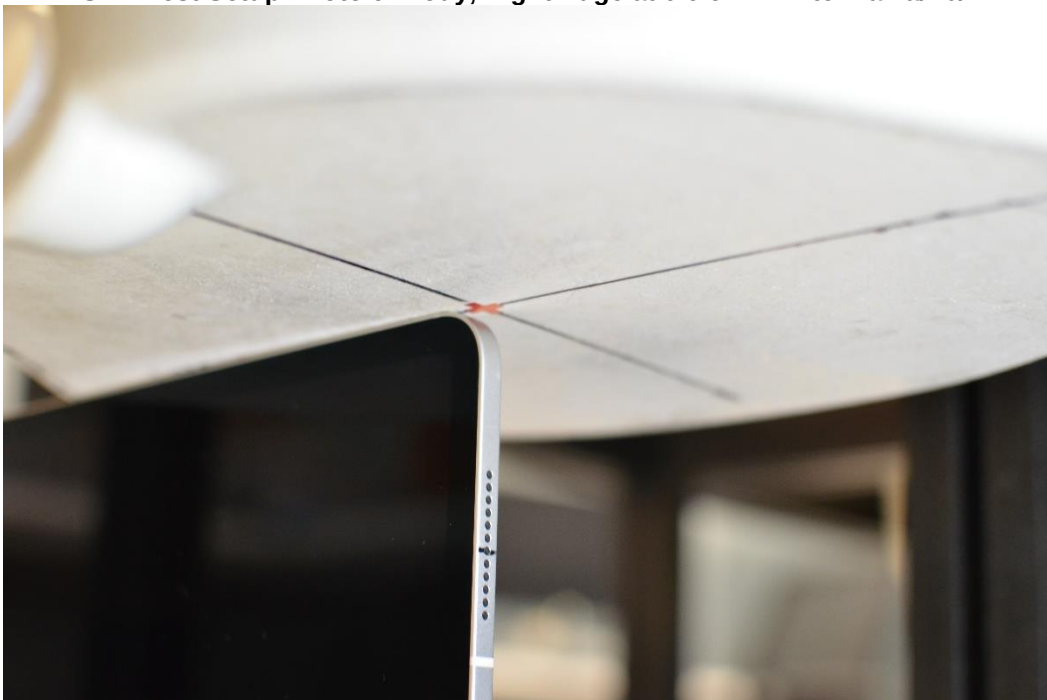
SAR Test Setup Photo 9: Body, Right Edge at 0.0 cm – Antenna 1a/1b/2
