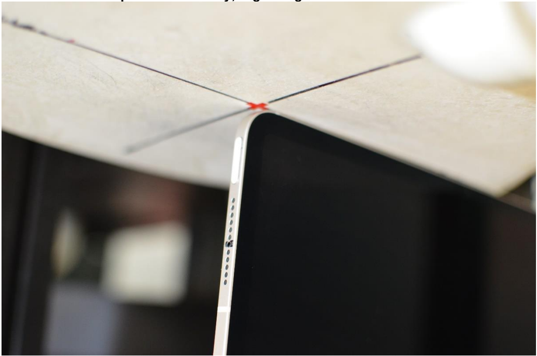
SAR Test Setup Photo 10: Body, Right Edge at 0.0 cm – Antenna 3a/3b/4/5T
