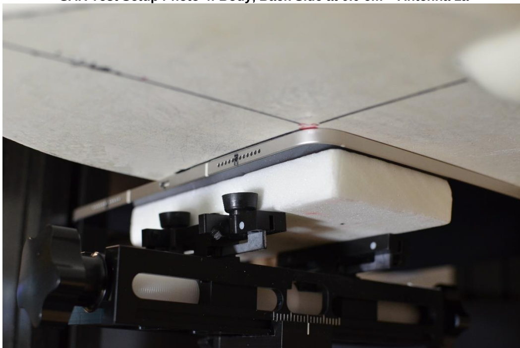
SAR Test Setup Photo 4: Body, Back Side at 0.0 cm – Antenna 1a
