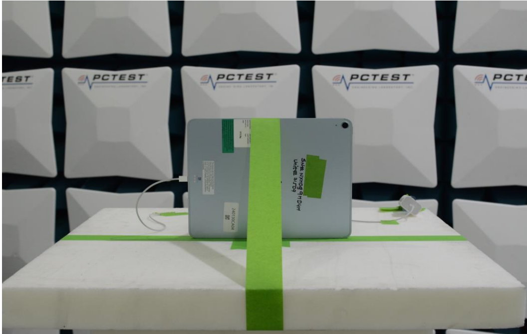
Figure 3: 1-18GHz Test Setup (Front View)
