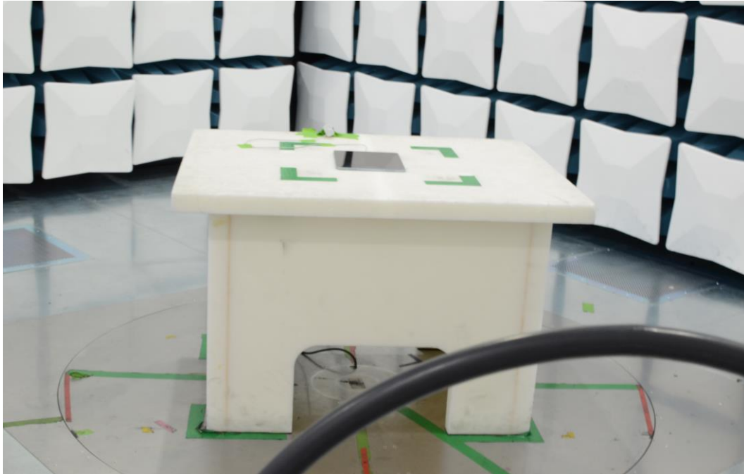
Figure 19: 9kHz-30MHz Test Setup (Front View)
