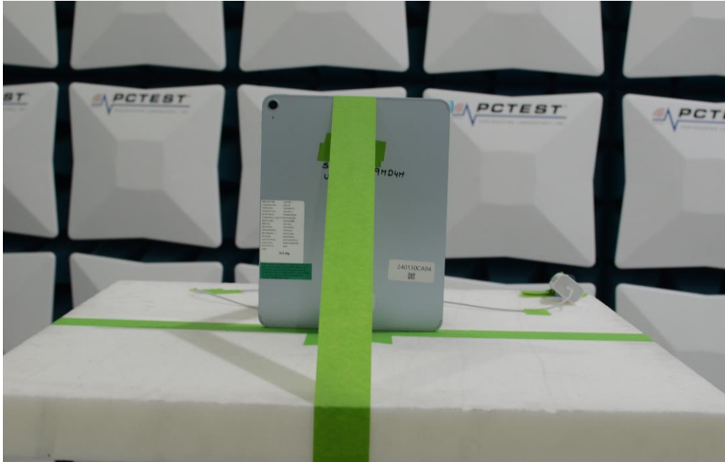
Figure 5: 1-18GHz Test Setup (Front View)
