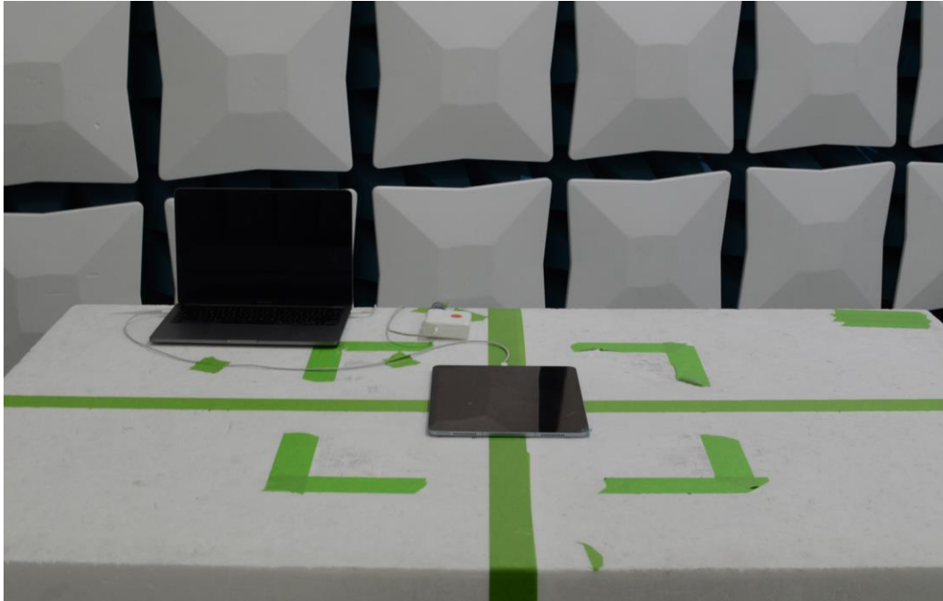
Figure 13: 30MHz-1GHz Test Setup (Front View)
