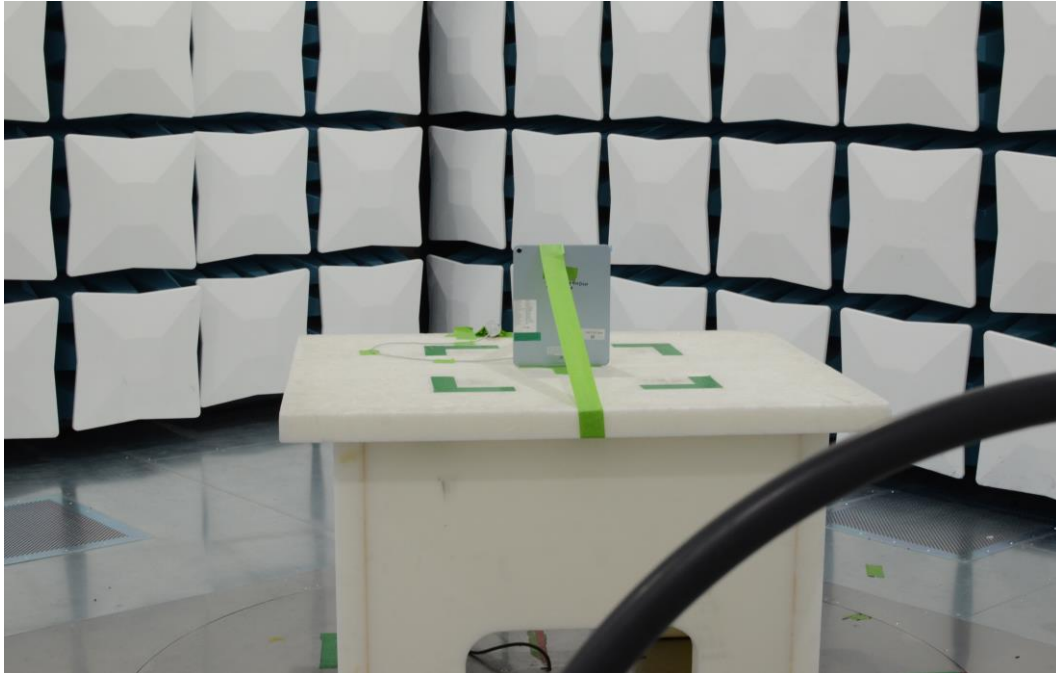
Figure 21: 9kHz-30MHz Test Setup (Front View)
