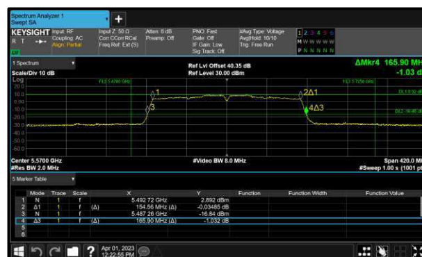
Figure 183 - 802.11ac VHT160 Maximum 99% OBW
