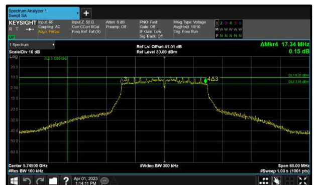
Figure 193 - 802.11n HT20 Maximum 6 dB EBW
