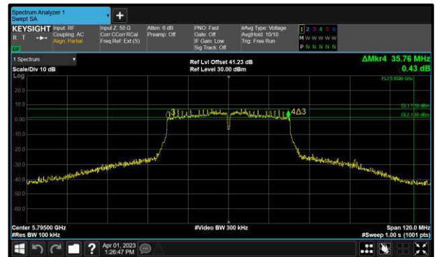
Figure 195 - 802.11n HT40 Maximum 6 dB EBW
