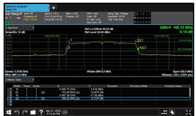
Figure 239 - 802.11ac VHT160 Maximum 99% OBW
