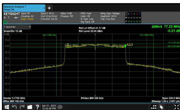
Figure 172 - 802.11ax HE80 SU Minimum 6 dB EBW
