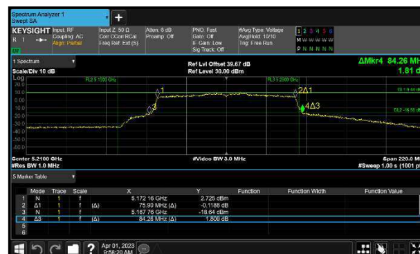
Figure 209 - 802.11ac VHT80 Maximum 99% OBW
