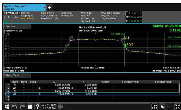
Figure 206 - 802.11n HT40 Minimum 99% OBW
