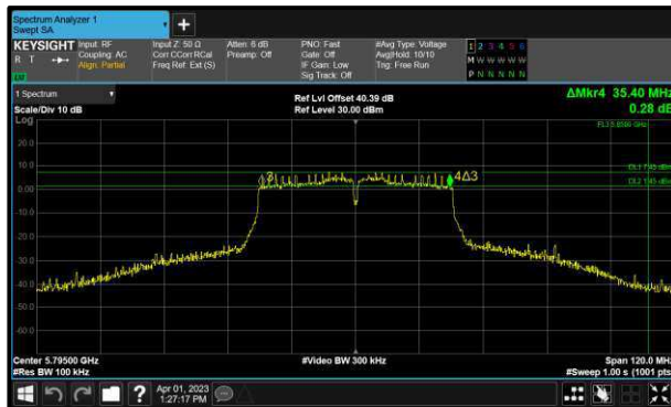
Figure 194 - 802.11n HT40 Minimum 6 dB EBW
