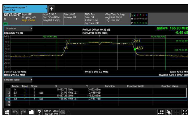
Figure 210 - 802.11ac VHT160 Minimum 99% OBW
