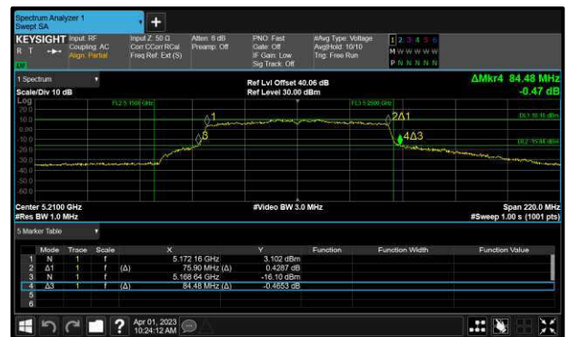
Figure 237 - 802.11ac VHT80 Maximum 99% OBW
