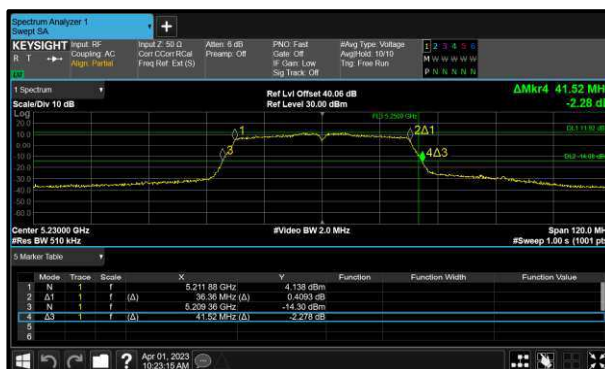
Figure 234 - 802.11n HT40 Minimum 99% OBW
