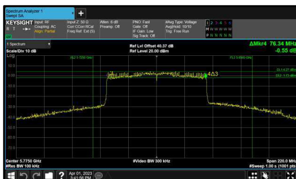
Figure 230 - 802.11ax HE80 SU Minimum 6 dB EBW
