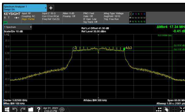
Figure 220 - 802.11n HT20 Minimum 6 dB EBW
