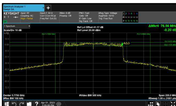
Figure 202 - 802.11ax HE80 SU Minimum 6 dB EBW
