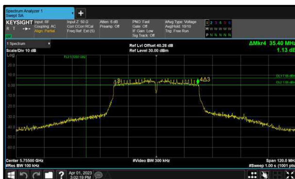
Figure 222 - 802.11n HT40 Minimum 6 dB EBW
