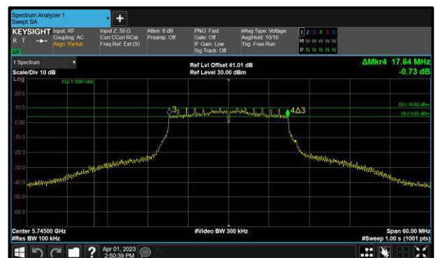
Figure 221 - 802.11n HT20 Maximum 6 dB EBW
