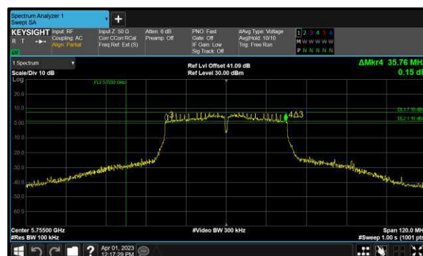
Figure 165 - 802.11n HT40 Maximum 6 dB EBW
