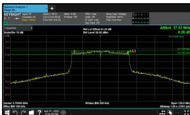
Figure 228 - 802.11ax HE40 SU Minimum 6 dB EBW
