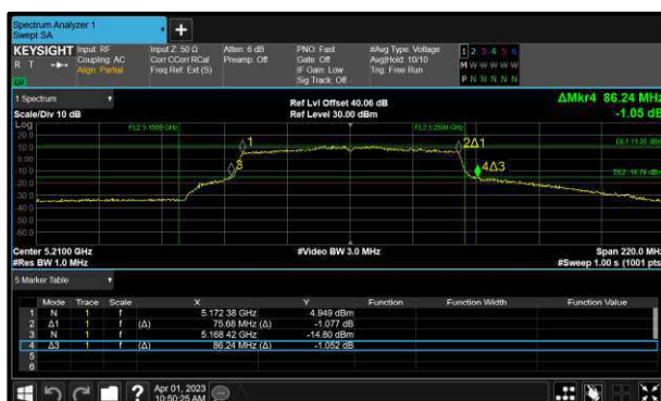
Figure 180 - 802.11ac VHT80 Minimum 99% OBW
