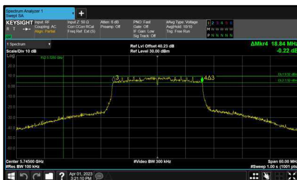
Figure 226 - 802.11ax HE20 SU Minimum 6 dB EBW
