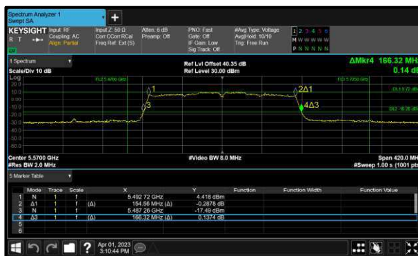
Figure 238 - 802.11ac VHT160 Minimum 99% OBW
