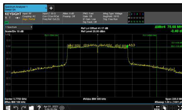
Figure 225 - 802.11ac VHT80 Maximum 6 dB EBW
