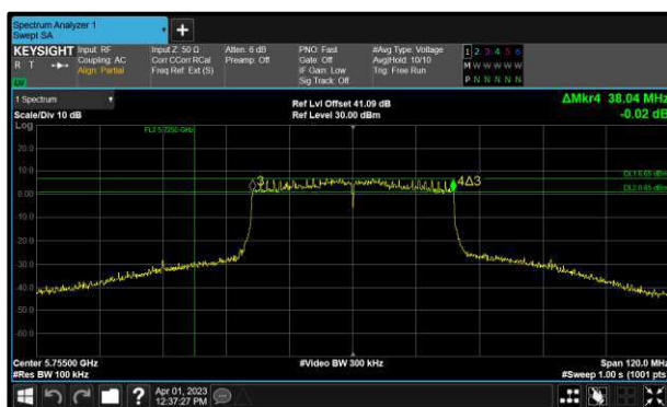
Figure 170 - 802.11ax HE40 SU Minimum 6 dB EBW
