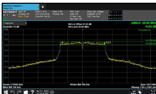
Figure 164 - 802.11n HT40 Minimum 6 dB EBW
