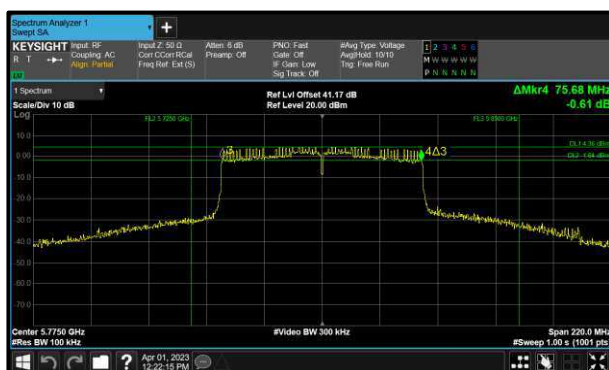
Figure 166 - 802.11ac VHT80 Minimum 6 dB EBW
