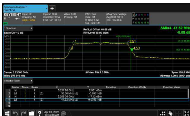
Figure 178 - 802.11n HT40 Minimum 99% OBW
