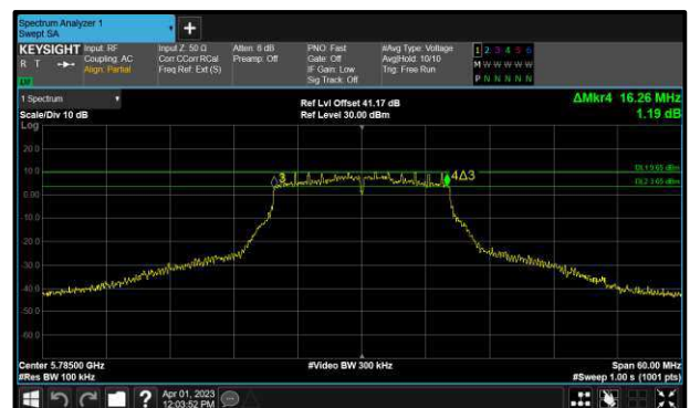
Figure 161 - 802.11a Maximum 6 dB EBW
