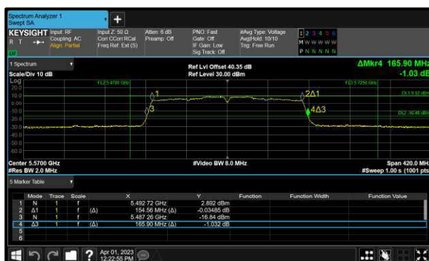
Figure 182 - 802.11ac VHT160 Minimum 99% OBW
