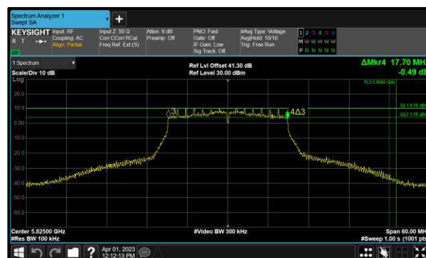
Figure 163 - 802.11n HT20 Maximum 6 dB EBW
