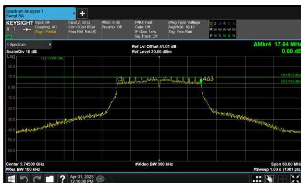
Figure 162 - 802.11n HT20 Minimum 6 dB EBW
