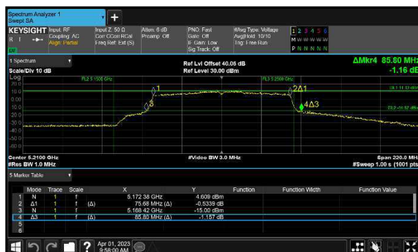
Figure 208 - 802.11ac VHT80 Minimum 99% OBW
