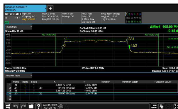
Figure 211 - 802.11ac VHT160 Maximum 99% OBW
