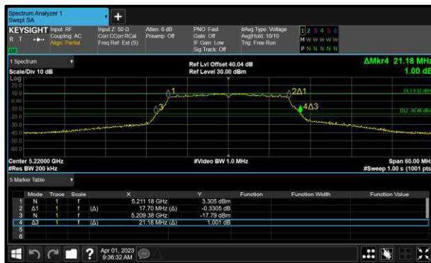
Figure 176 - 802.11n HT20 Minimum 99% OBW
