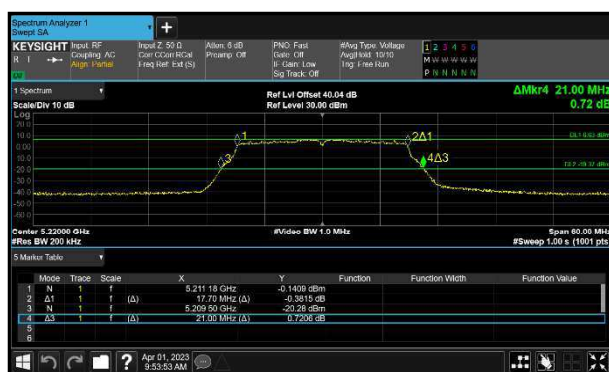
Figure 204 - 802.11n HT20 Minimum 99% OBW
