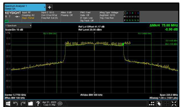
Figure 197 - 802.11ac VHT80 Maximum 6 dB EBW
