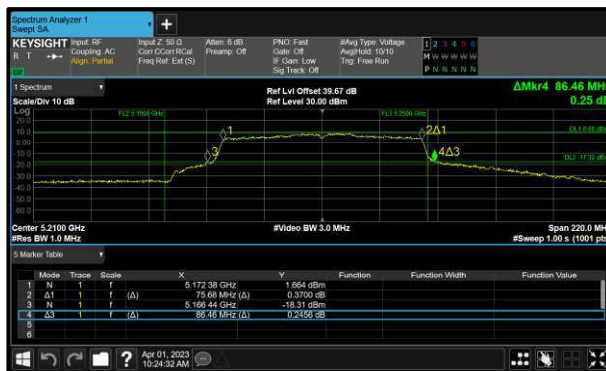
Figure 236 - 802.11ac VHT80 Minimum 99% OBW
