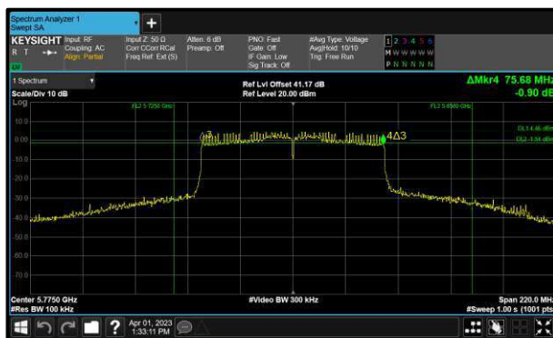
Figure 196 - 802.11ac VHT80 Minimum 6 dB EBW
