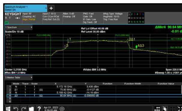
Figure 181 - 802.11ac VHT80 Maximum 99% OBW
