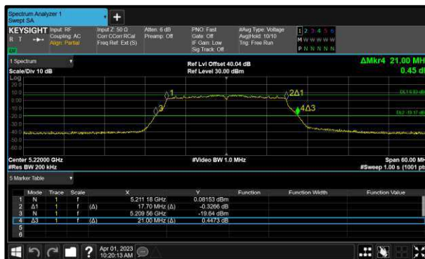
Figure 232 - 802.11n HT20 Minimum 99% OBW
