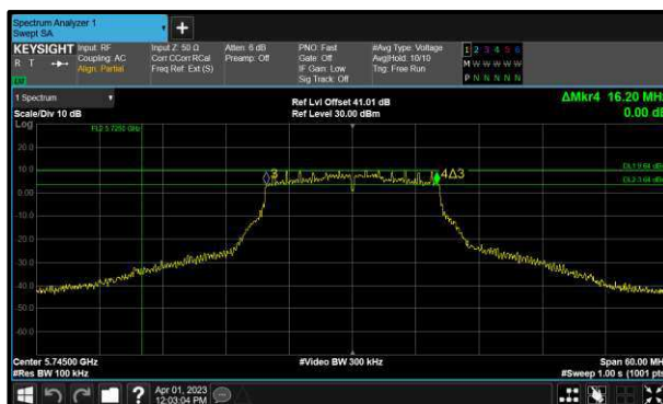
Figure 160 - 802.11a Minimum 6 dB EBW
