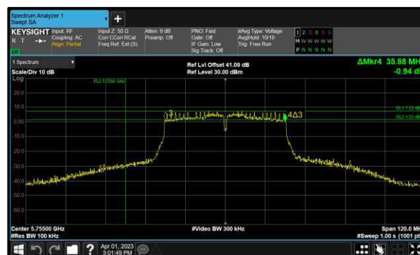
Figure 223 - 802.11n HT40 Maximum 6 dB EBW
