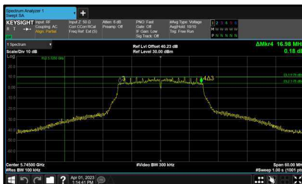
Figure 192 - 802.11n HT20 Minimum 6 dB EBW
