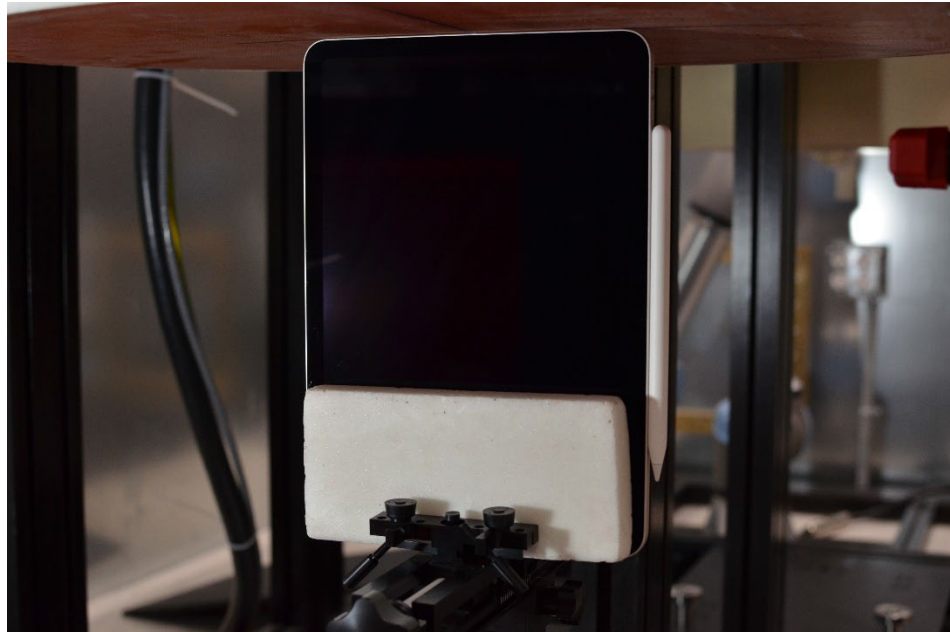
Wireless Power Transfer Test Setup Photo 13 – Top Edge at 0mm
