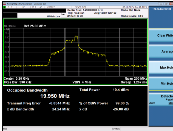
Plot 7-26. 26dB BW & 99% OBW Antenna 3c (80MHz BW 11ax Index 44 – RU52 – Ch.58)
