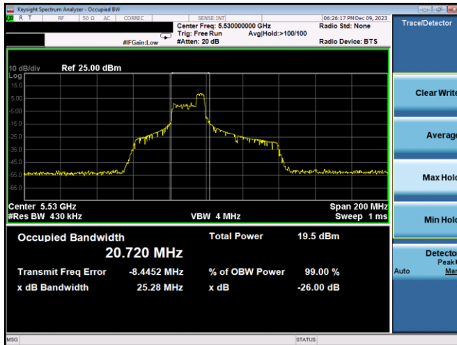
Plot 7-38. 26dB BW & 99% OBW Antenna 3c (80MHz BW 11ax Index 44 – RU52 – Ch.106)
